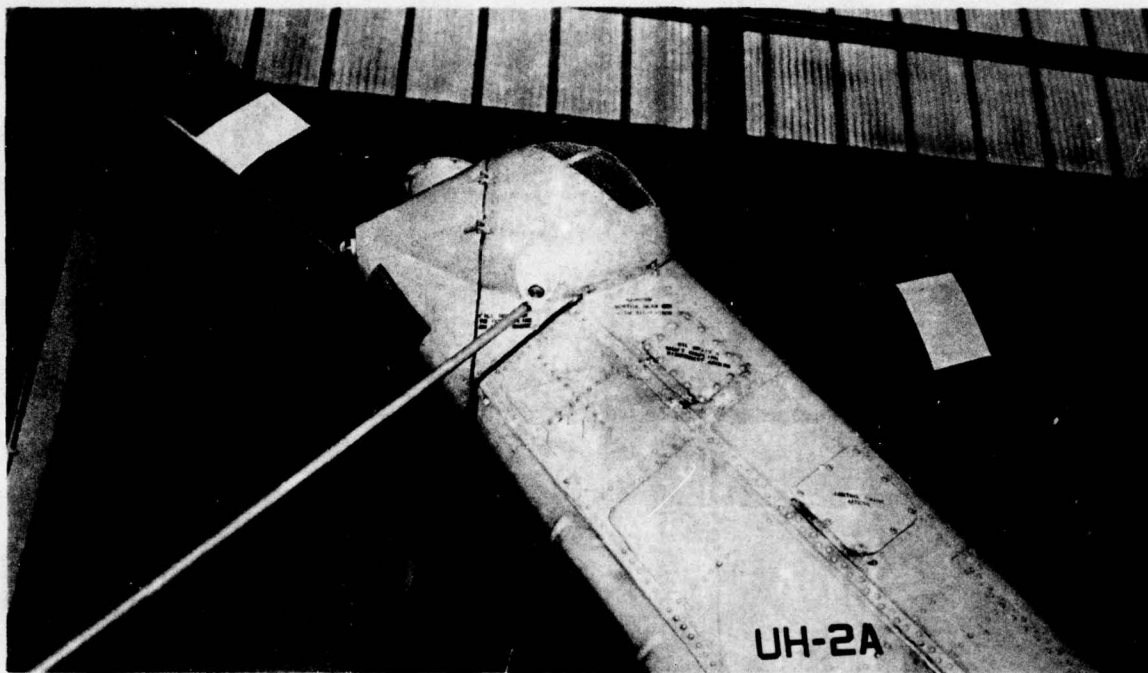
Figure 5. Tail-rotor gear box sight gauge is difficult to read from the ground.
