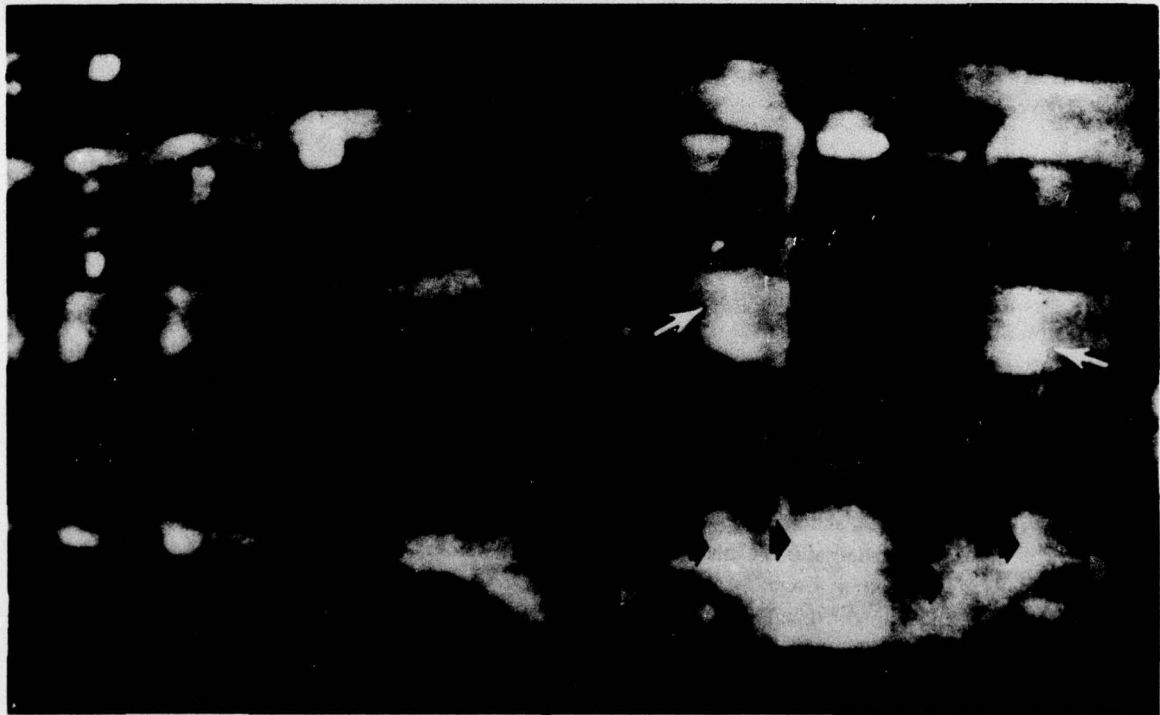
Figure 5a. Thermogram taken on 1 April 1974, after installation of reflectors. Note that the area of heat loss is reduced by about 50% (compare with photograph on cover).
