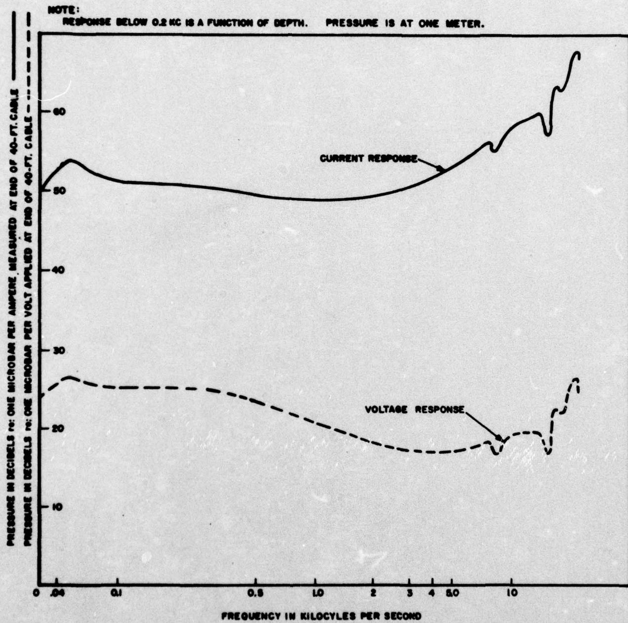
FIGURE 2-9. TRANSMITTING RESPONSE CURVES, J9 TRANSDUCER
