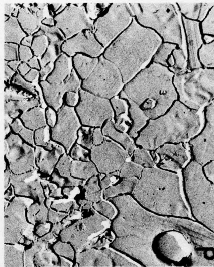
FIGURE 4. MICROSTRUCTURES OF POLISHED AND ETCHED LONGITUDINAL SECTIONS OF \text{Si}_3\text{N}_4 AND OF VARIOUS SIALONS: (a) NC132, (b) HS130-1, (c) G35AlON-1, (d) SS1/R3-1. 12000X
