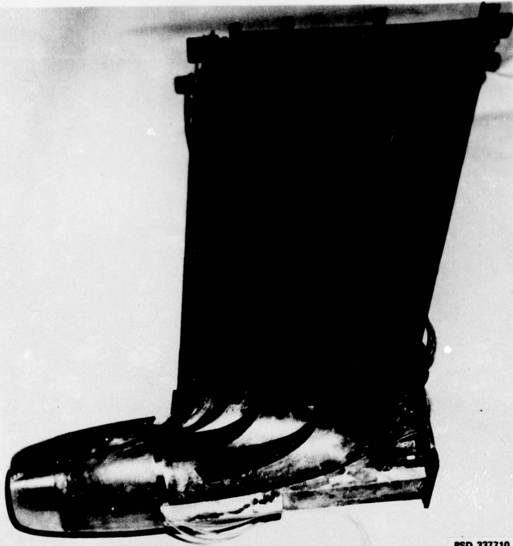
Figure 33 – Internal View of Supercavitating Model Showing Splitter Vanes in Elbow and Strut
