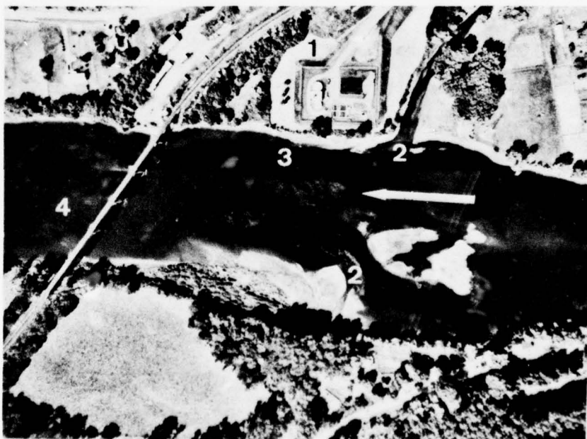
g. 1) Boston and Maine Railroad Bridge near the Windsor Treatment Plant. 2) The two mill brooks entering from both sides. 3) Effluent is seen discharging from the plant to the river and remaining alongshore but gradually dispersing. 4) The riprap protecting the pier cribs and deposition zones behind the piers is also visible.
