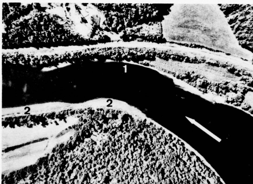
d. River bend at Section 12. Note the surface constriction as flow reaches the bend. 1) A small surface slick of some type with deterioration caused by the turbulence. 2) Accretion of material on the inside bank.
