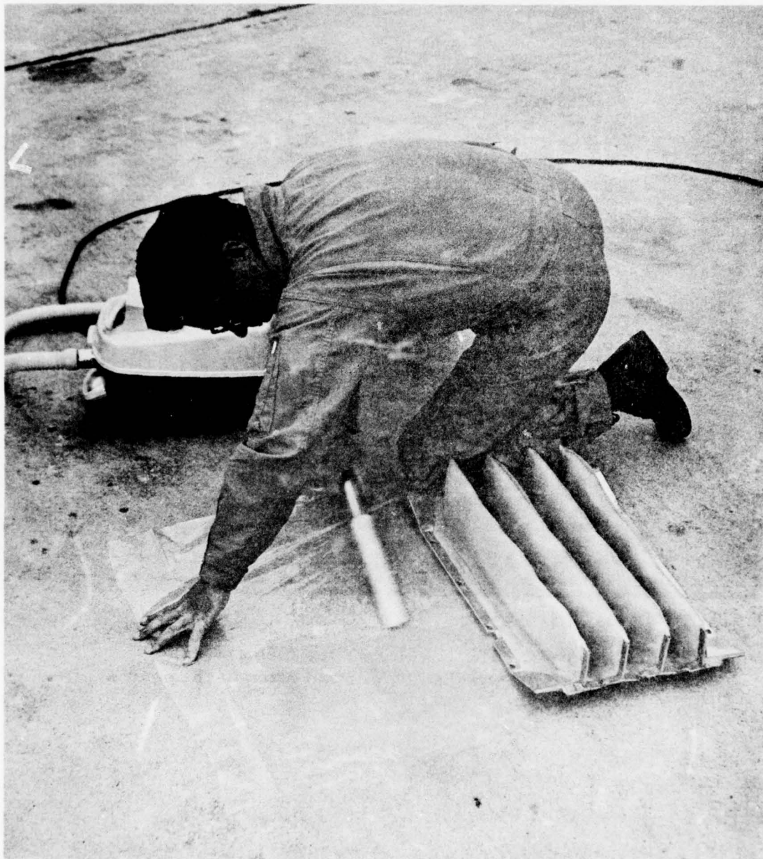
Figure 26. Collecting samples from Barrier Filter element after hover in sand and dust environment.
