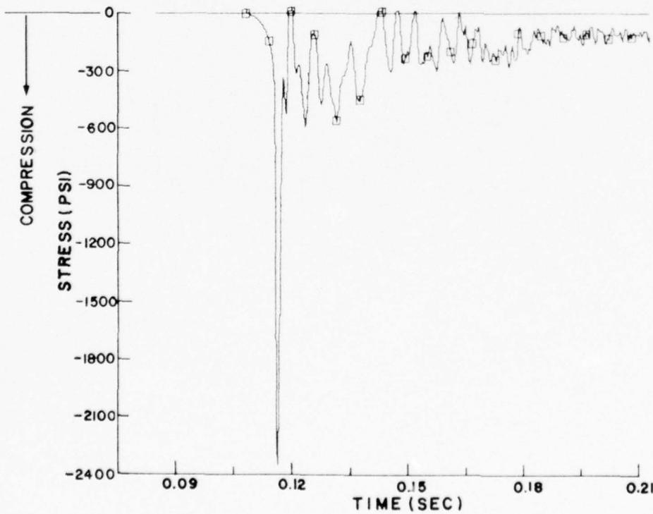
FIG. 15 PROBLEM P3 - VERTICAL STRESS AND IMPULSE NEAR TOP CORNER OF STRUCTURE, 1 FT AWAY
