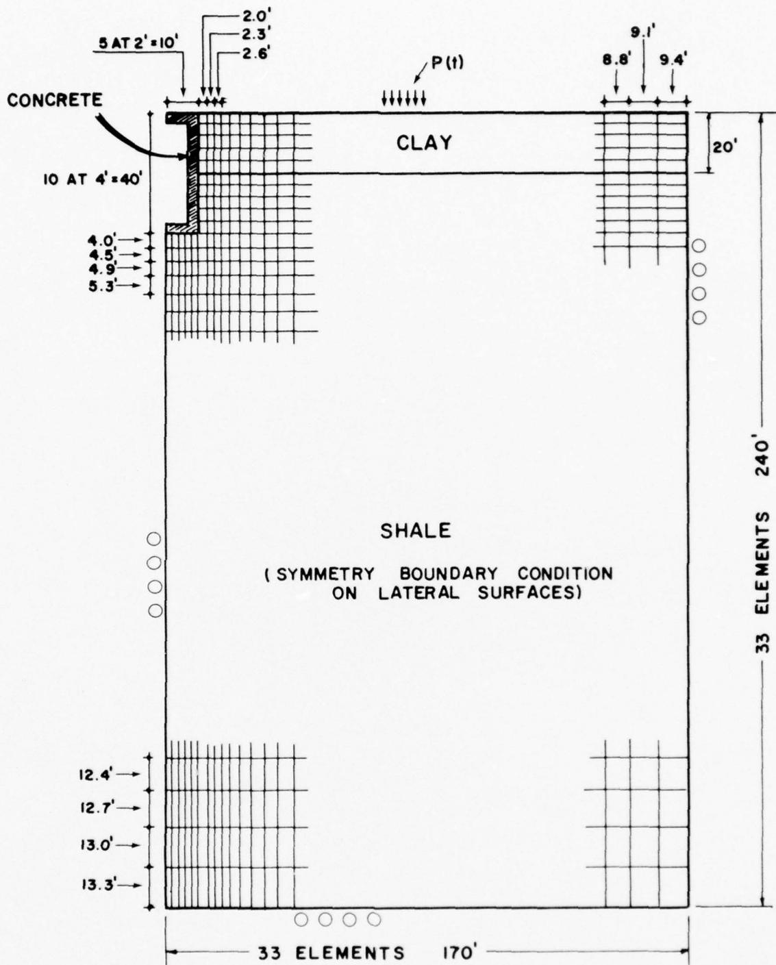
FIG. 4 PROBLEM P3 - FINITE ELEMENT MESH
