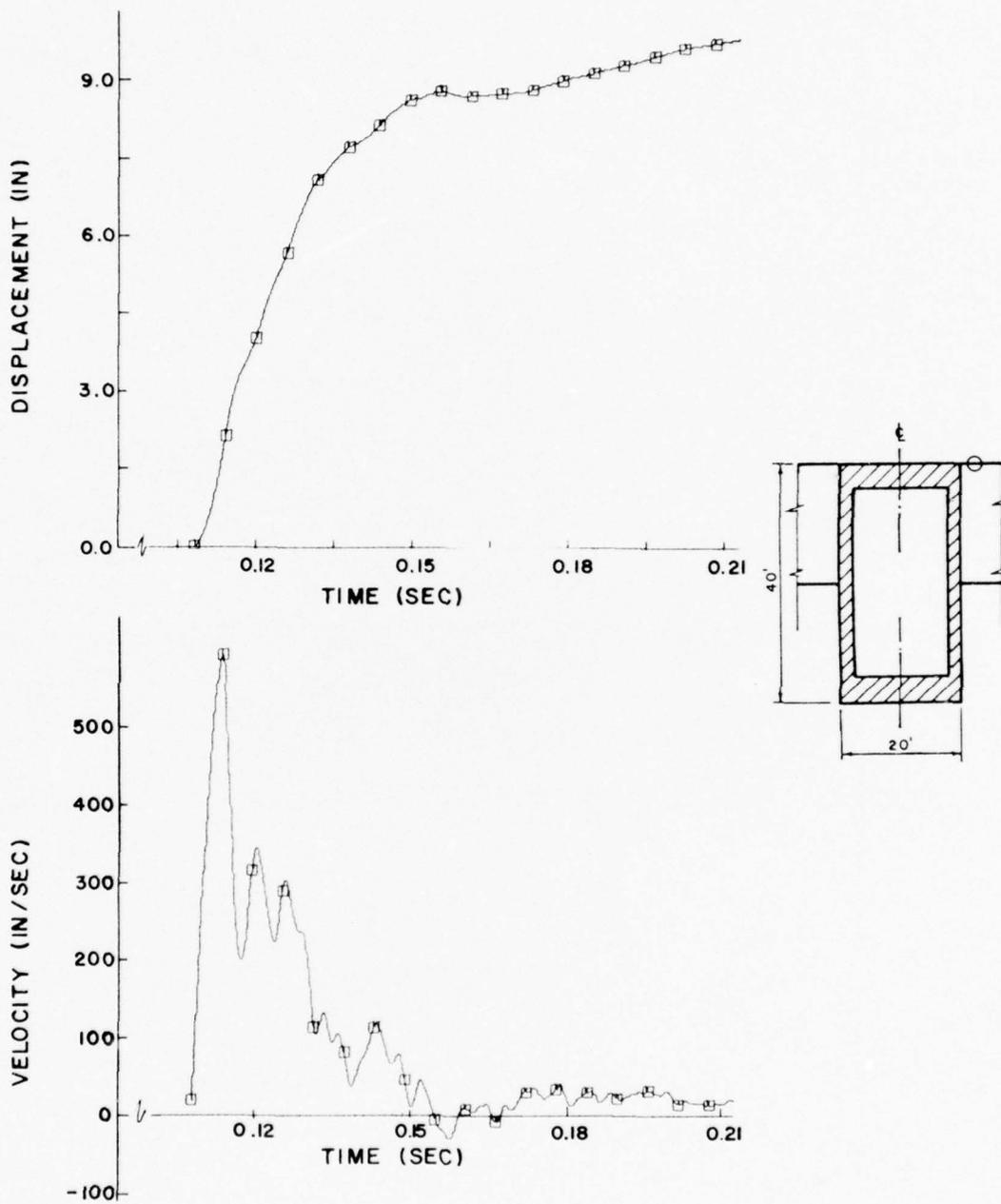
FIG. 12 PROBLEM P3 - VERTICAL RESPONSE 2 FT AWAY FROM TOP CORNER OF STRUCTURE
