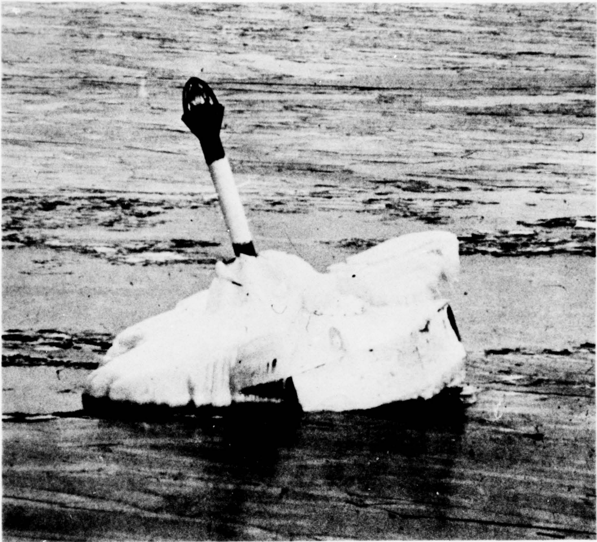
Figure 8. 16-foot-diameter octagonal ice buoy with ice and snow on deck (Detour Reef Light Station - FY74)
