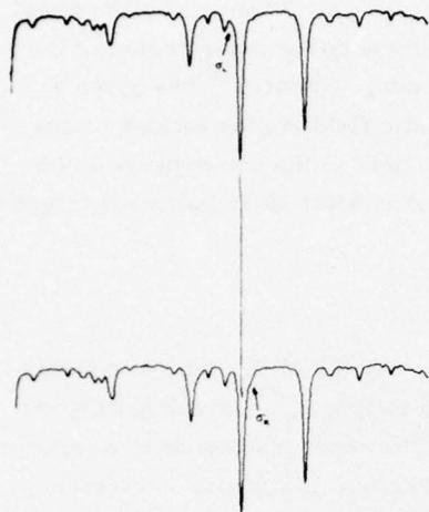
Figure 10a. Spectra of a Magnetic Element in Opposite Circular Polarizations in the Fe I Line, at 1564.8 nm. This line has a large Lande' factor ( $g=3$ ) and shows a large Zeeman splitting because of this and because of the large wavelength
