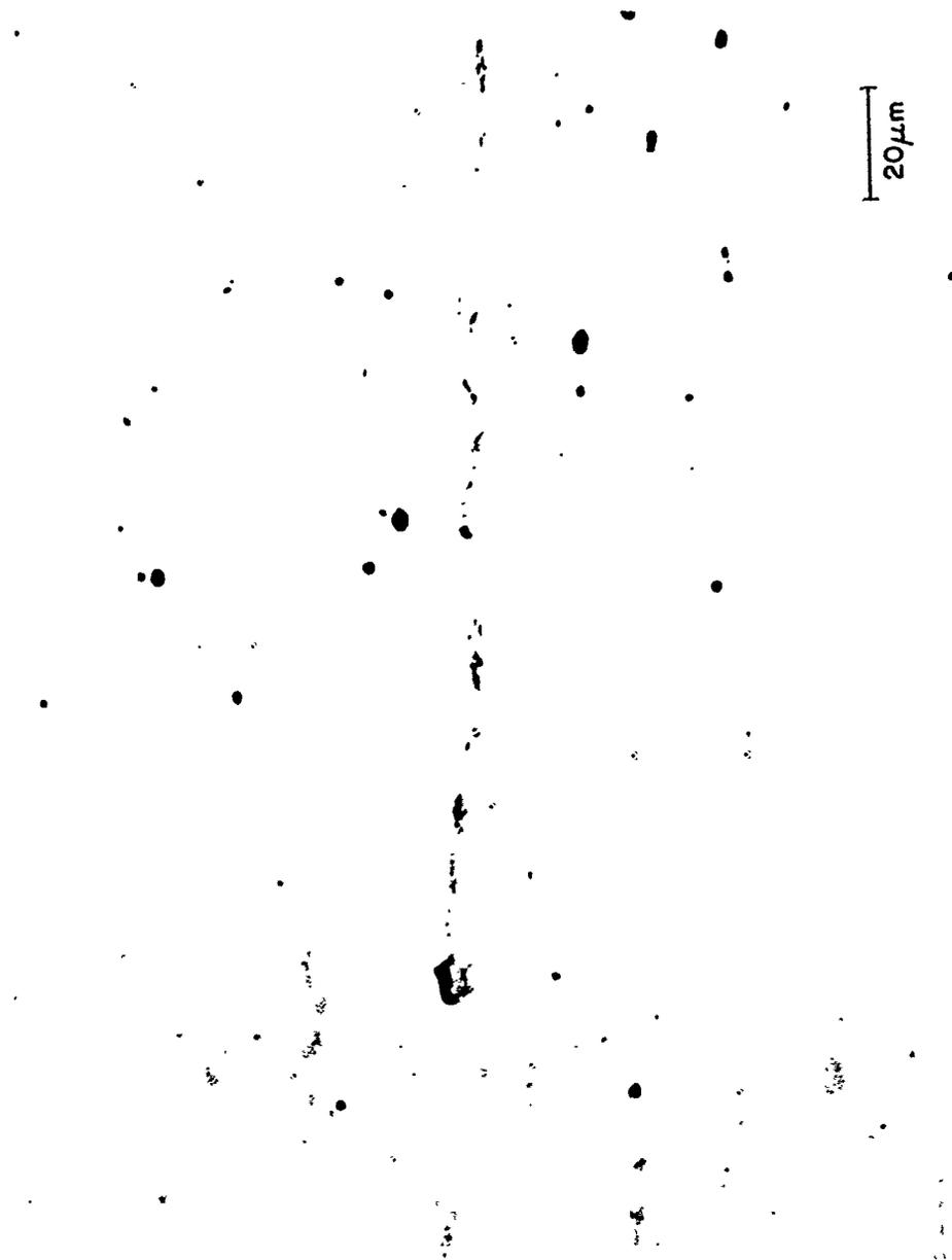
Figure 34. 7075 Aluminum Braze with 10  $\mu\text{m}$  Vapor Deposited Magnesium at 1.38 MPa (200 psi) Pressure, As-Brazed Condition. 500X No Etch
