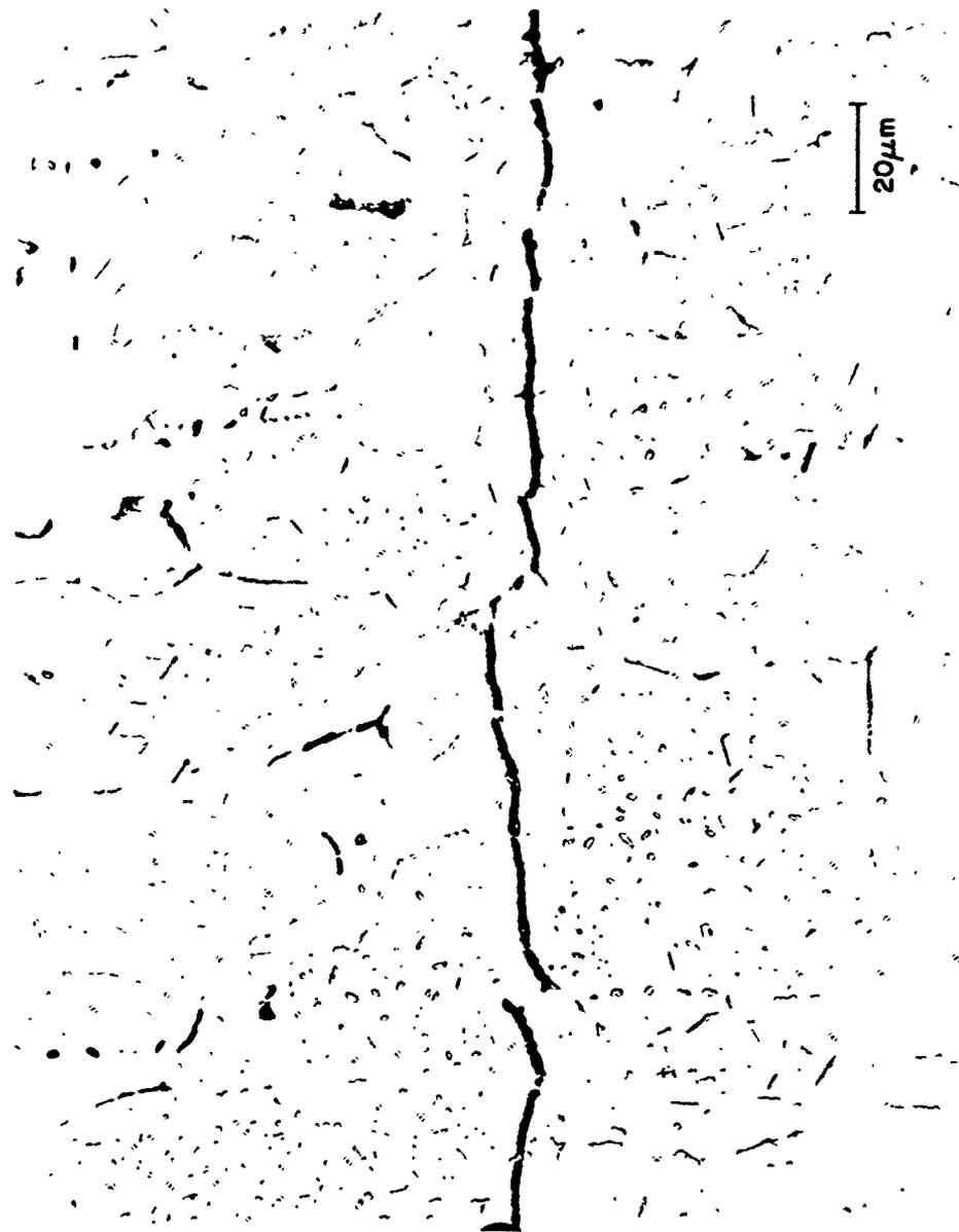
Figure 20. 6061 Aluminum Braze with 10 μm Vapor Deposited Silver at 26 MPa (3.8 ksi) Pressure, As-Brazed Condition. 500X 1% HF
