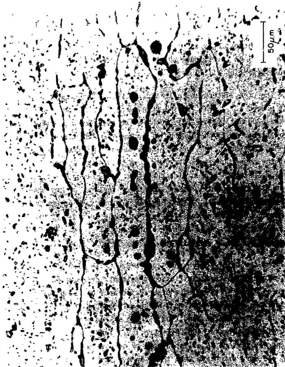
Figure 5. 6061 Aluminum Brazed with 25  $\mu\text{m}$  Silver Foil at 70 kPa (10 psi) Pressure, As-Brazed Condition. 250X 1% HF
