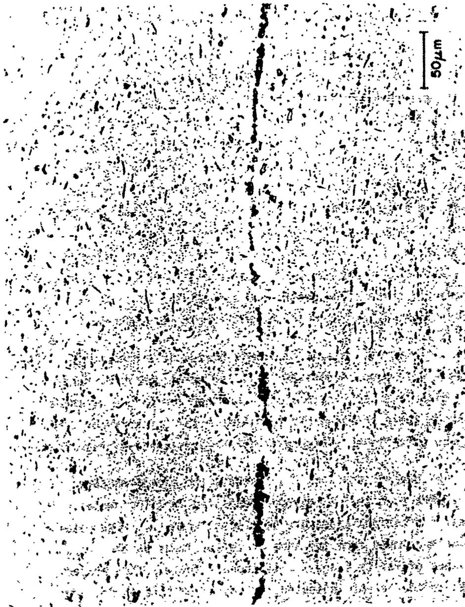
Figure 15. 6061 Aluminum Braze with 34  $\mu\text{m}$  Electroplated Silver at 1380 kPa (200 psi) Pressure, As-Brazed Condition. 200X 20% NaOH
