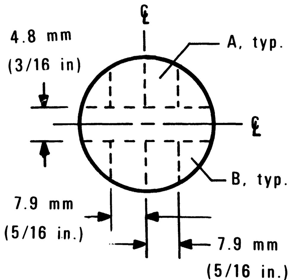
Figure 4. Sectioning Plan for 25.4 mm (1 in.) Diameter Brazed Cylinders.
