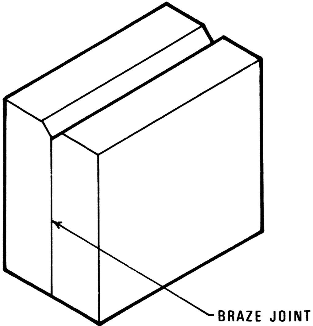
Figure 2. Specimen for Wedge Test
