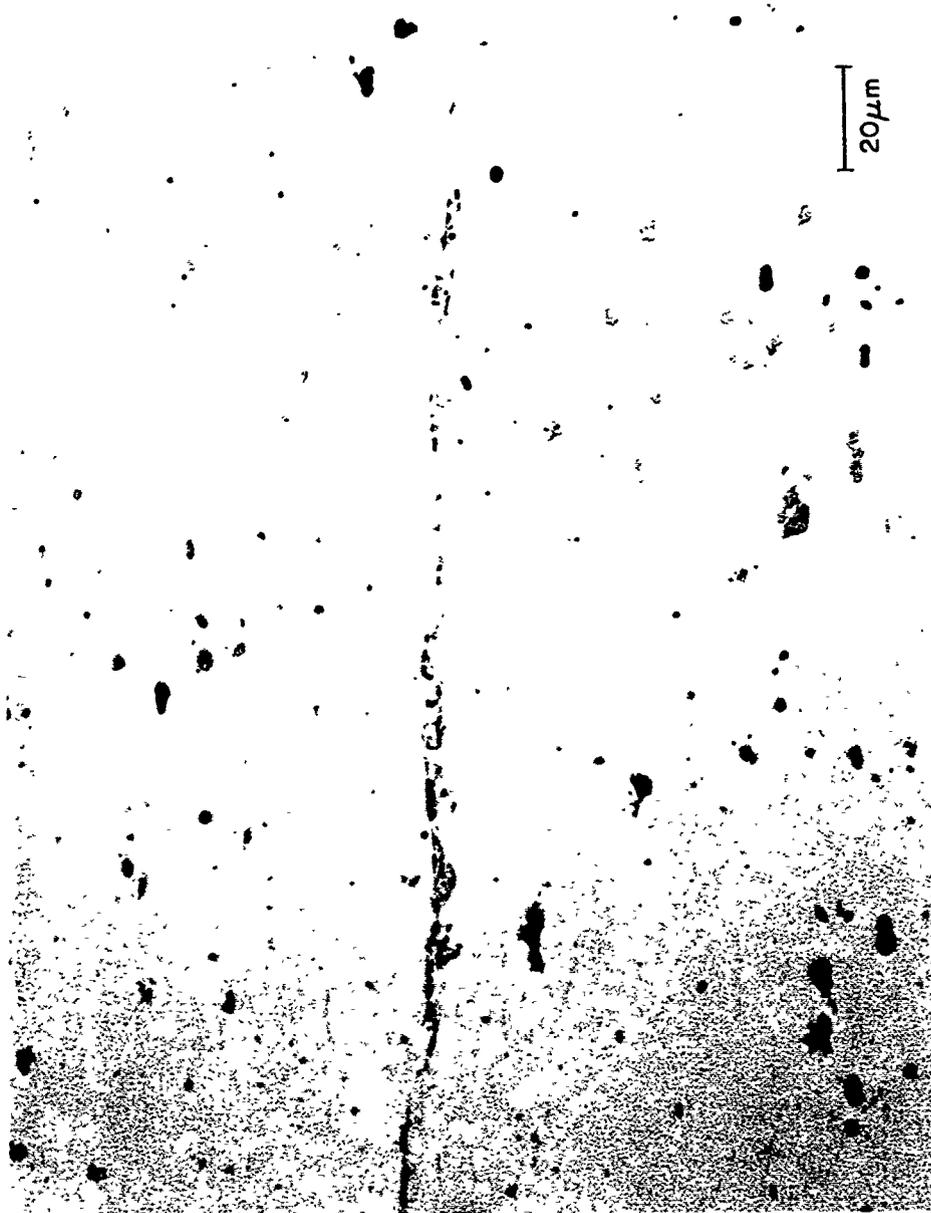
Figure 35. 7075 Aluminum Brazed with 2  $\mu\text{m}$  Vapor Deposited Magnesium at 6.89 MPa (1000 psi) Pressure, As-Brazed Condition. 500X No Etch
