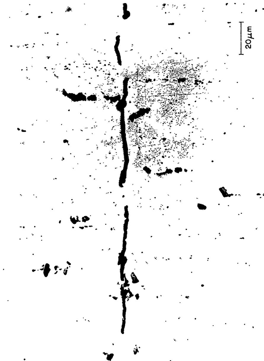
Figure 21. 6061 Aluminum Brazed with 10  $\mu\text{m}$  Vapor Deposited Silver at 26 MPa (3.8 ksi) Pressure, As-Brazed Condition. 500X 1% HF
