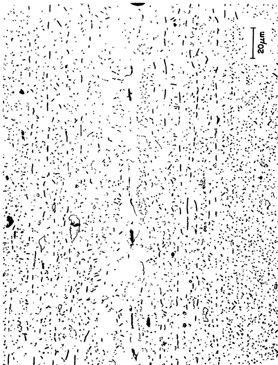
Figure 37. 7075 Aluminum Brazed with 1 μm Electroplated Ag28Cu Filler
