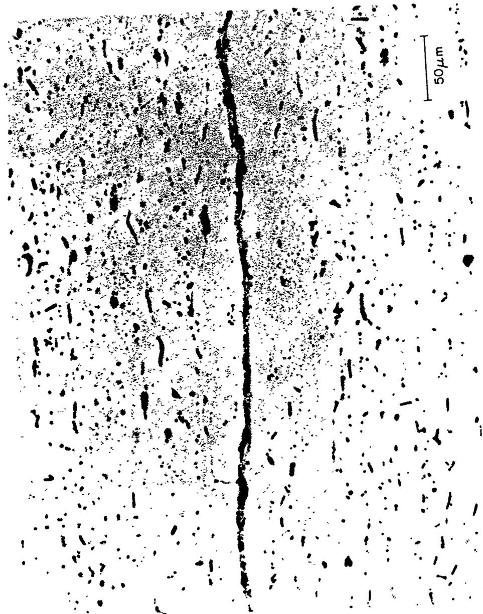
Figure 28. 6061 Aluminum Brazed with 6 μm Vapor Deposited Copper at 1.38 MPa (200 psi) Pressure, As-Brazed Condition. 250X 0.5% HF
