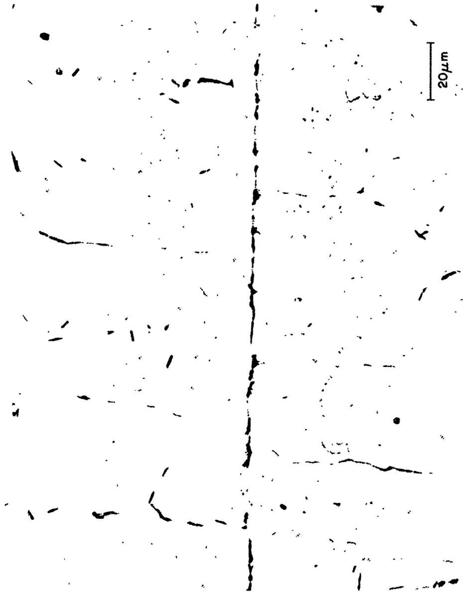
Figure 18. 6061 Aluminum Braze with 2  $\mu$ m Vapor Deposited Silver at 26 MPa (3.8 ksi) Pressure, As-Brazed Condition. 500X 1% HF
