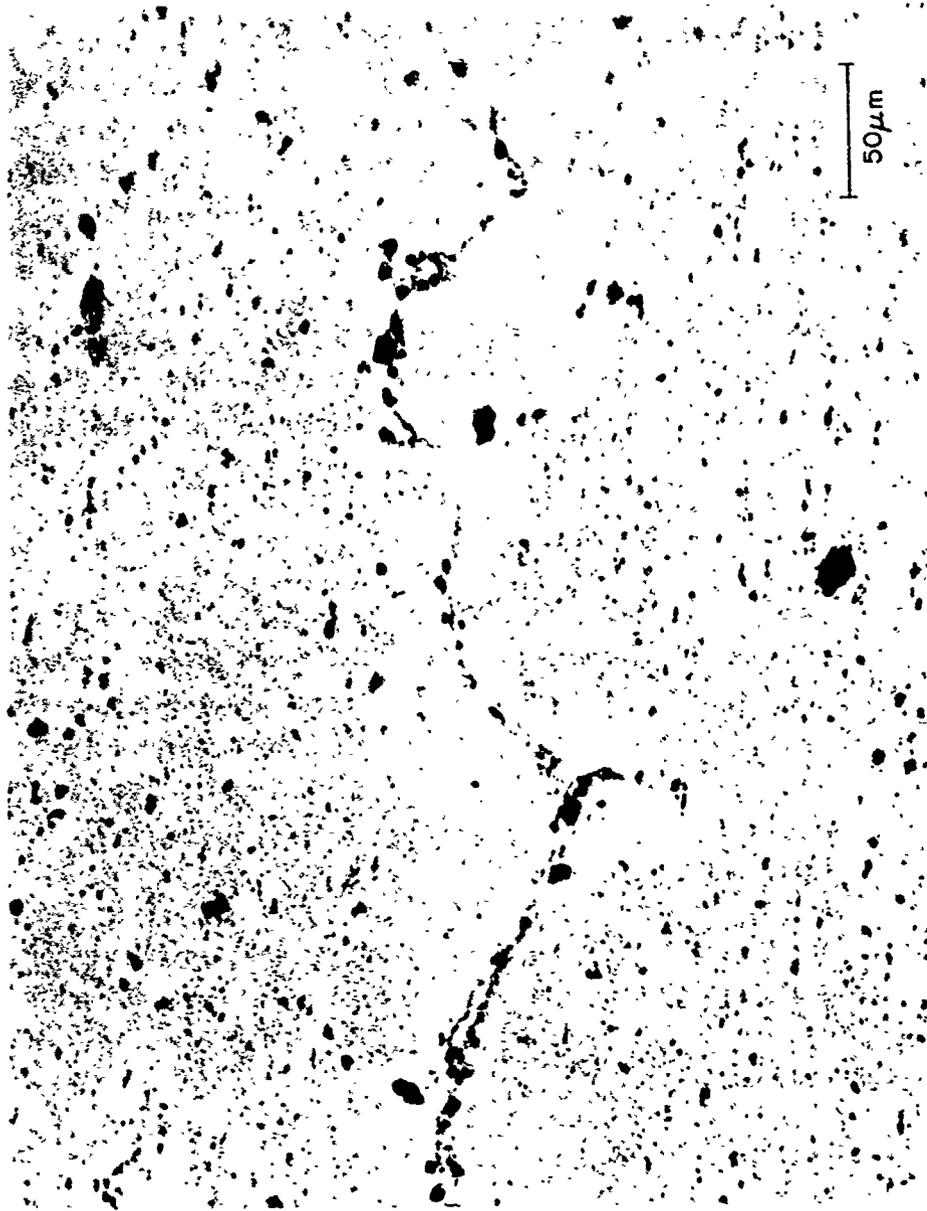
Figure 27. 6061 Aluminum Brazed with 12 μm Copper Foil at 1.38 MPa (200 psi) Pressure, Diffusion Treated 1000 Hours at 500°C. 250X Kellers
