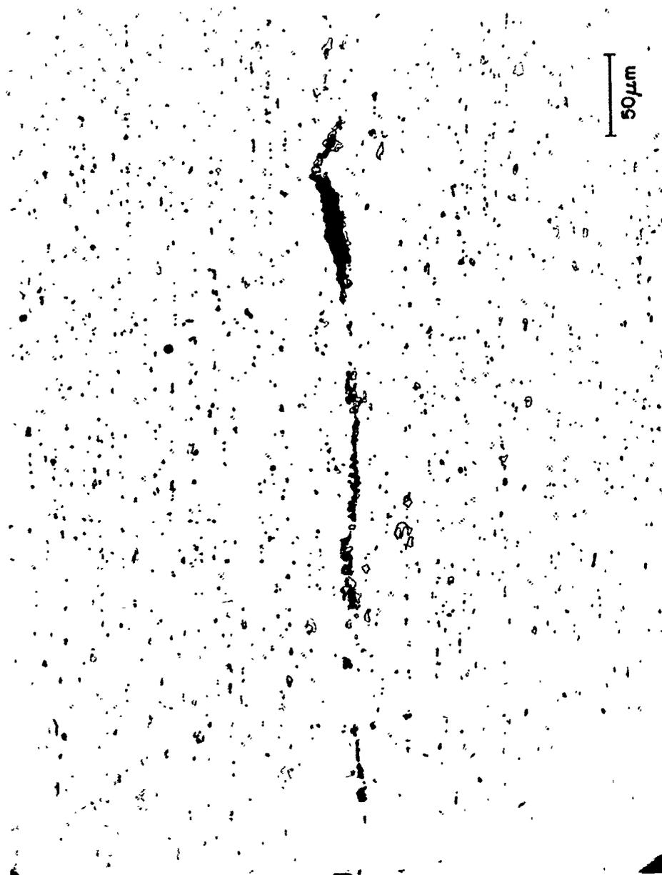
Figure 16. 6061 Aluminum Brazed with 58  $\mu\text{m}$  Electroplated Silver at 1380 kPa (200 psi) Pressure, T6 Condition. 200X 20% NaOH
