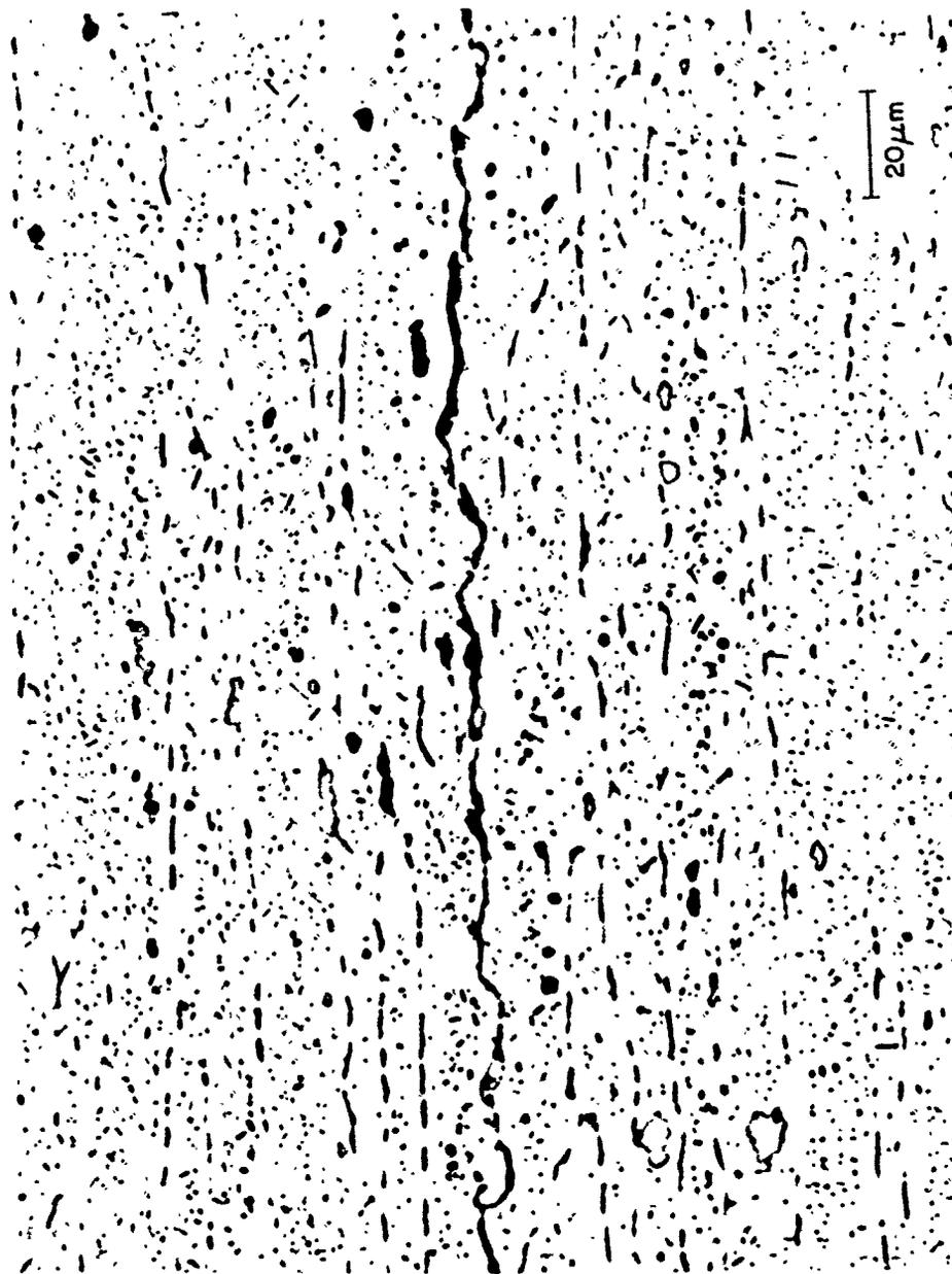
Figure 32. 7075 Aluminum Braze with 25  $\mu\text{m}$  Magnesium Foil at 490°C, As-Brazed Condition. 500X 0.5% HF
