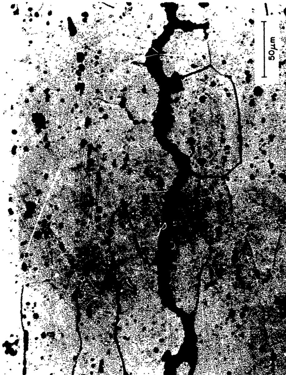
Figure 7. 6061 Aluminum Brazed with 25 μm Silver Foil at 70 kPa (10 psi) Pressure, T6 Condition. 250X 1% HF
