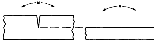
Fig. 3. Nominal stress in the presence of a crack is equivalent to replacing cracked body by a smooth body (at right) having the same depth as the unbroken ligament, obviously a defective "analysis."
