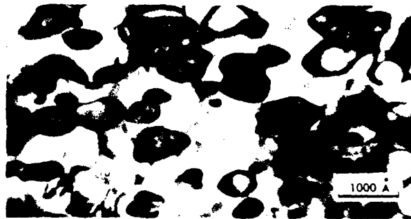
(a) Bright field electron micrograph of the \omega phase formed in Ti-11.6Mo
