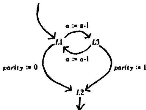
From this it can be deduced that the L1-L3 loop does not alter *parity*, and that after this loop exits to L2 control cannot pass back to the loop, and so that *PARITY* need not be an argument to L1 or L3 in the SCHEME version.
