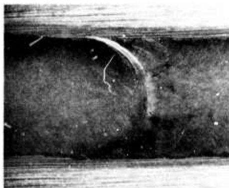
Figure 5-30 Photomicrographs of Varestraint Test Specimens in (I) Udimet 718 and (II) Inconel 718 alloys in the ST(1800°F) condition at various augmented strain levels (X10)
