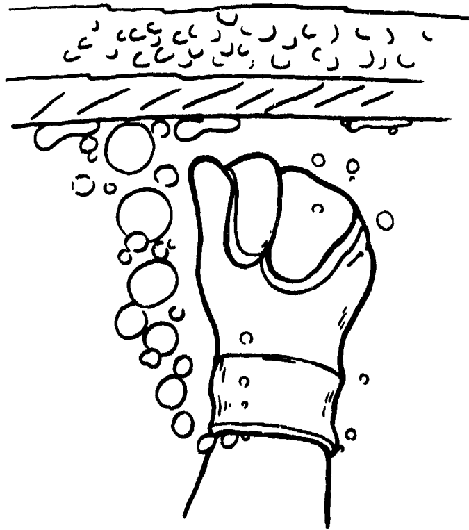
FIGURE 3-3. DIVER LEAKING AIR FROM SUIT AT CUFF
