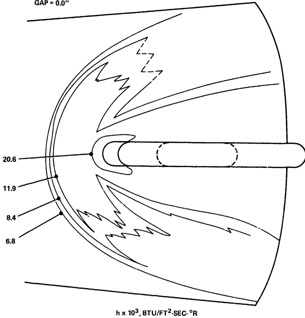
FIG. 19 ISOHEATING CONTOURS FOR FLUSH-MOUNTED UNSWEPT FIN. TOP VIEW
