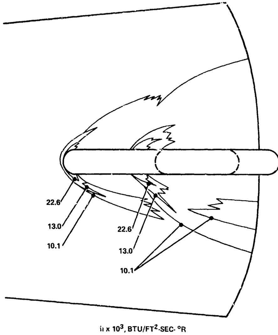
FIG. 32 ISOHEATING CONTOURS FOR 60° SWEEP FIN WITH 0.060-INCH FIN-CONE GAP. TOP VIEW
