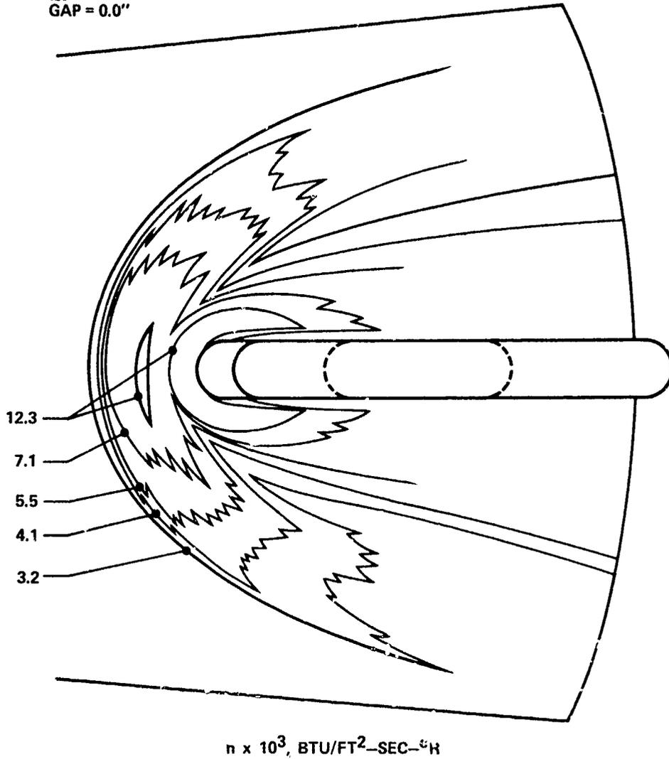
FIG. 18 ISOHEATING CONTOURS FOR FLUSH-MOUNTED UNSWEPT FIN. TOP VIEW, ABOUT 10° FORWARD OF LEADING EDGE
