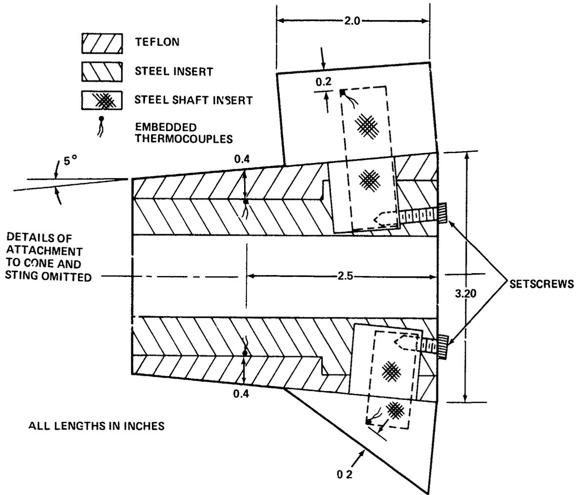
FIG. A - 1 SCHEMATIC DIAGRAM OF FINNED EXTENSION
