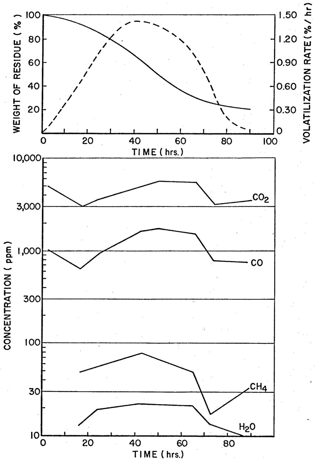
Figure 1. Weight loss and volatilization rate of, and concentration of volatiles from poly-1,4-phenylene during isothermal aging at 371°C in air
