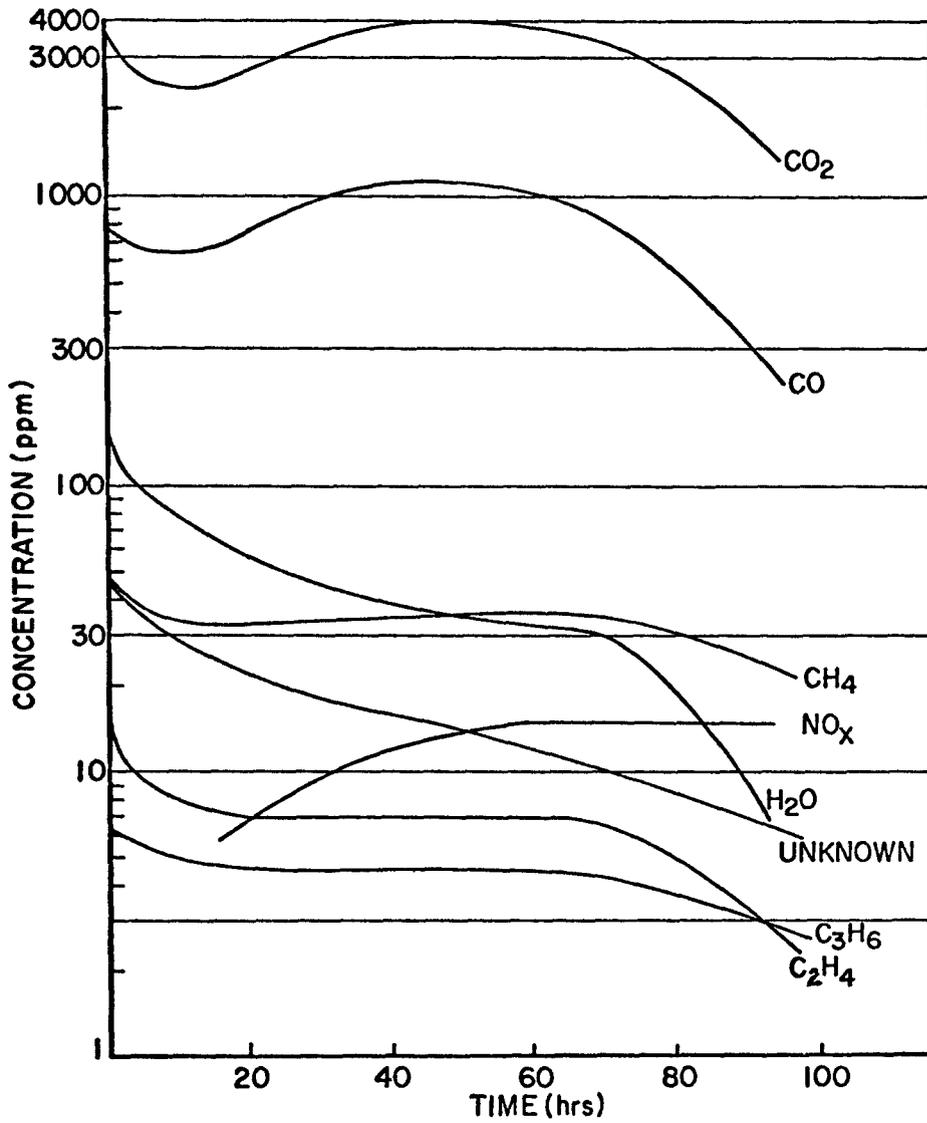
Figure 12. Concentration of volatiles from poly-p-benzamide fiber during isothermal aging at 371°C in air
