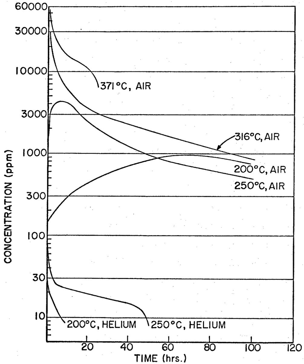
Figure 3. Concentrations of carbon dioxide from poly-2,6-dimethyl-1,4-phenylene oxide (PPO) during isothermal aging at 200, 250, 316, and 371°C in helium and in air
