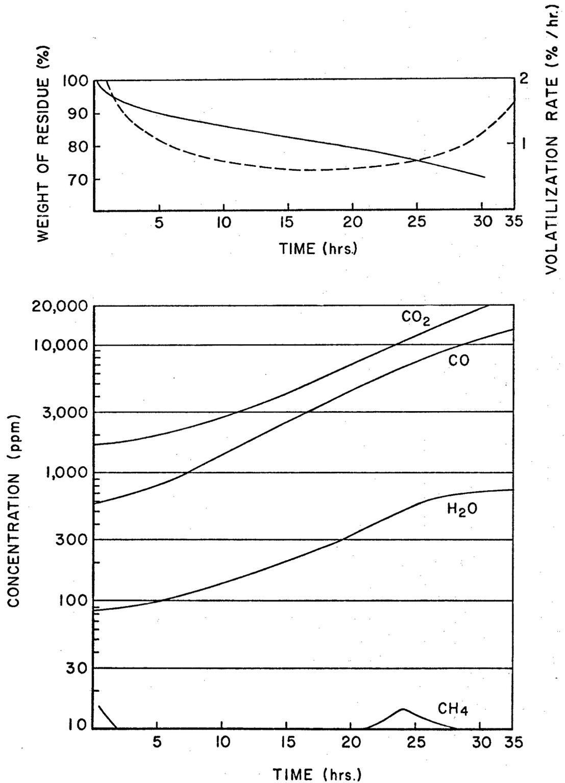
Figure 9. Weight loss and volatilization rate of, and concentration of volatiles from, poly-2,6-diphenyl-1,4-phenylene oxide (P<sub>3</sub>O) during isothermal aging at 371°C in air
