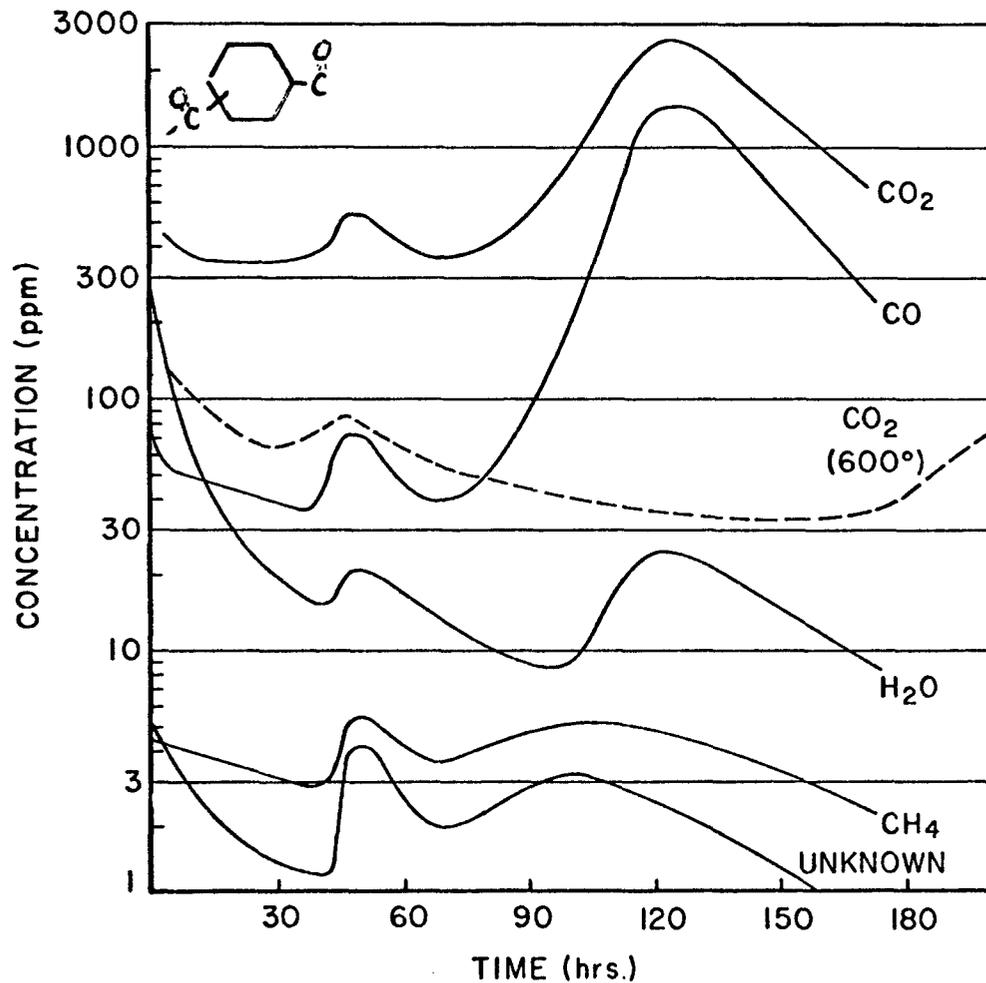
Figure 10. Weight loss and volatilization rate of, and concentration of volatiles from poly(p-phenylene) iso-terephthalate at 371°C, and of carbon dioxide at 600°F, in air
