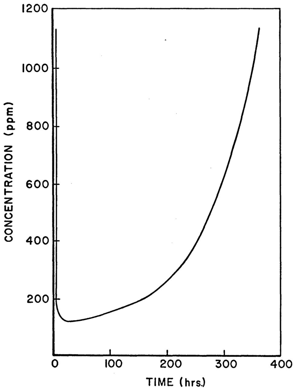
Figure 8. Concentration of carbon dioxide from poly-2,6-diphenyl-1,4-phenylene oxide (P<sub>3</sub>O) during isothermal aging at 316°C in air
