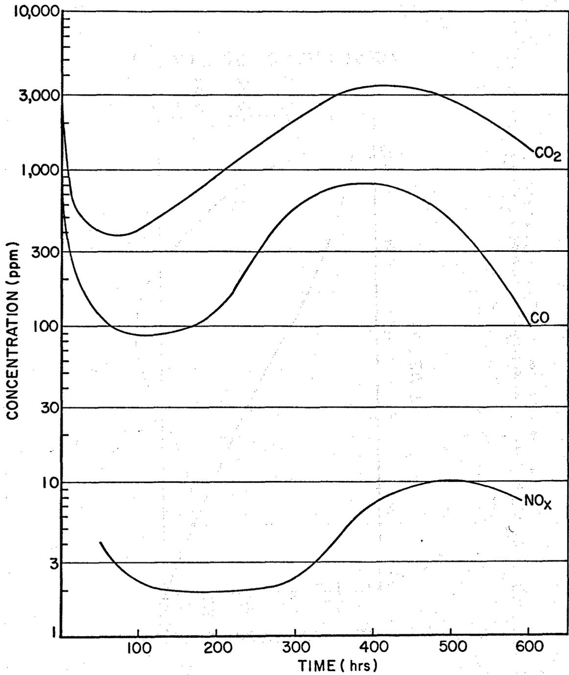
Figure 19. Concentration of volatiles (I) from polybenzimidazobenzophenanthroline (BBB) during isothermal aging at 371°C in air
