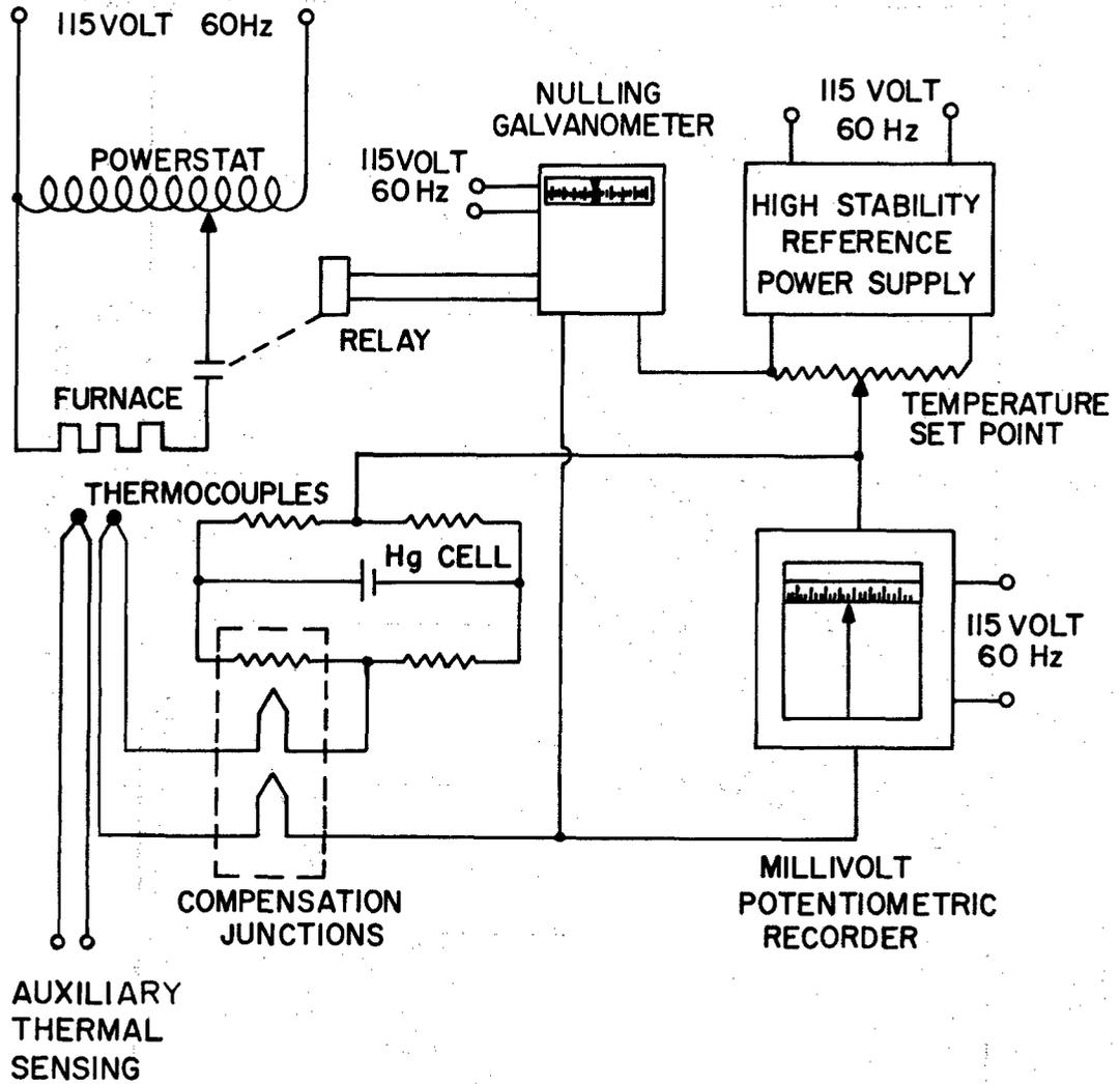
Figure 23. Circuit Diagram of the Thermal Measurement and Control System
