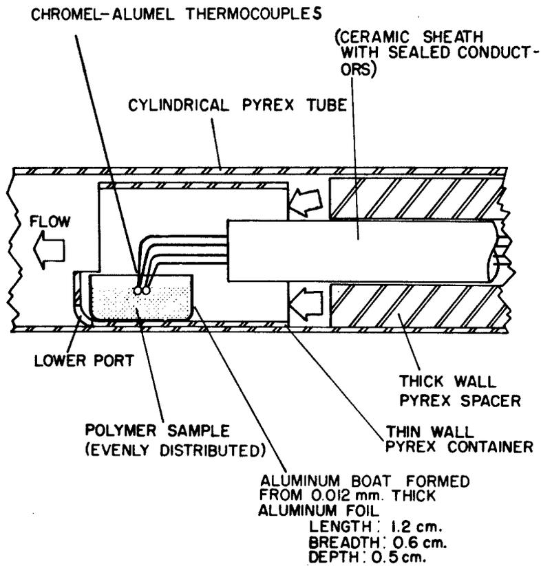
Figure 24. Sampleholder of the Isothermal Aging - Effluent Gas Analysis Equipment
