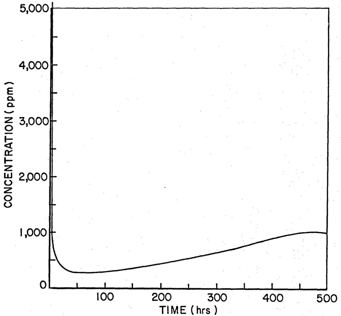
Figure 21. Concentration of carbon dioxide from polybenzimidazoisoquinoline (BBL) during isothermal aging at 371°C in air
