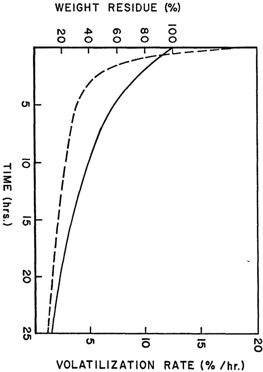
Figure 6. Weight loss and volatilization rate of poly-2,6-dimethyl-1,4-phenylene oxide (PPO) during isothermal aging at 371°C in air
