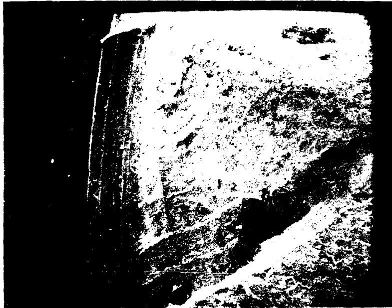
Figure 14. SEM micrograph of the OZ cap screw fracture, 10x. Note regions of fatigue crack initiation and propagation. Coarse machining marks can be observed on the thread area.
