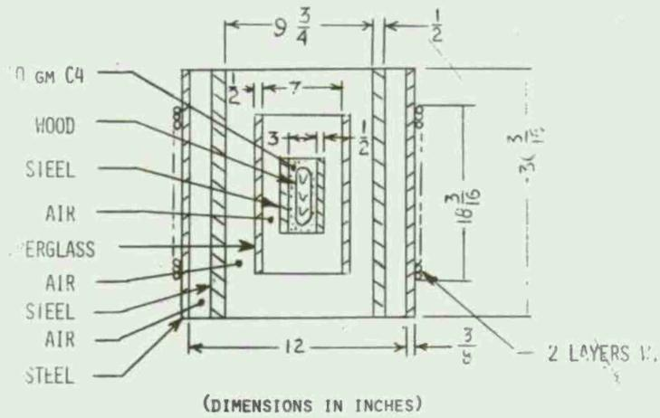
Fig 2a Basic 1/2-scale construction
