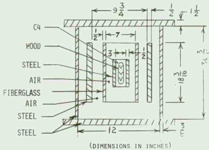
Fig 2b Basic 1/2-scale construction with end plates
