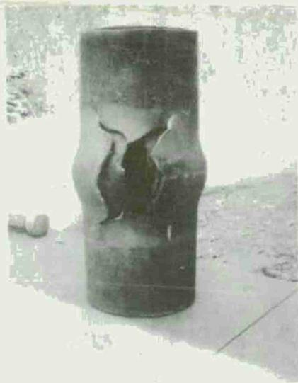
Half-scale test with 910-g cased charge. Test 9 (Table 6).
