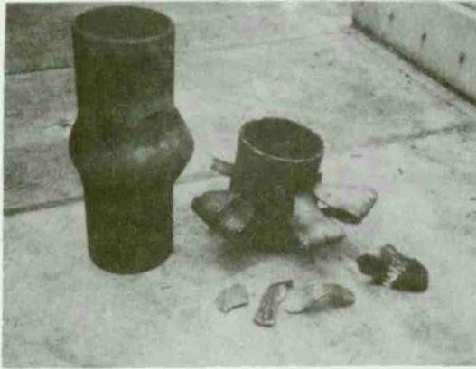
a. Left: cased charge 550-g with fiberglass 18 cm ID x 1.27 cm wall, Test 3. Right: no liner. Test 4 (Table 8)
