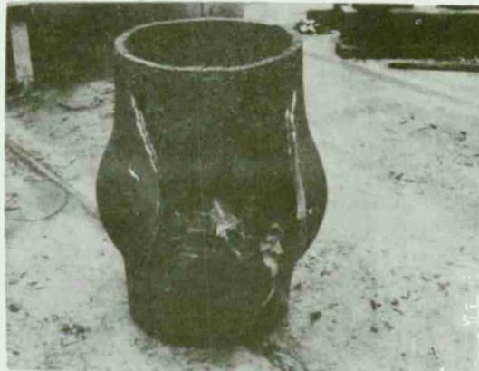
b. Cased charge 550-g heavy wall fiberglass liner. Test 18 (Table 8)
