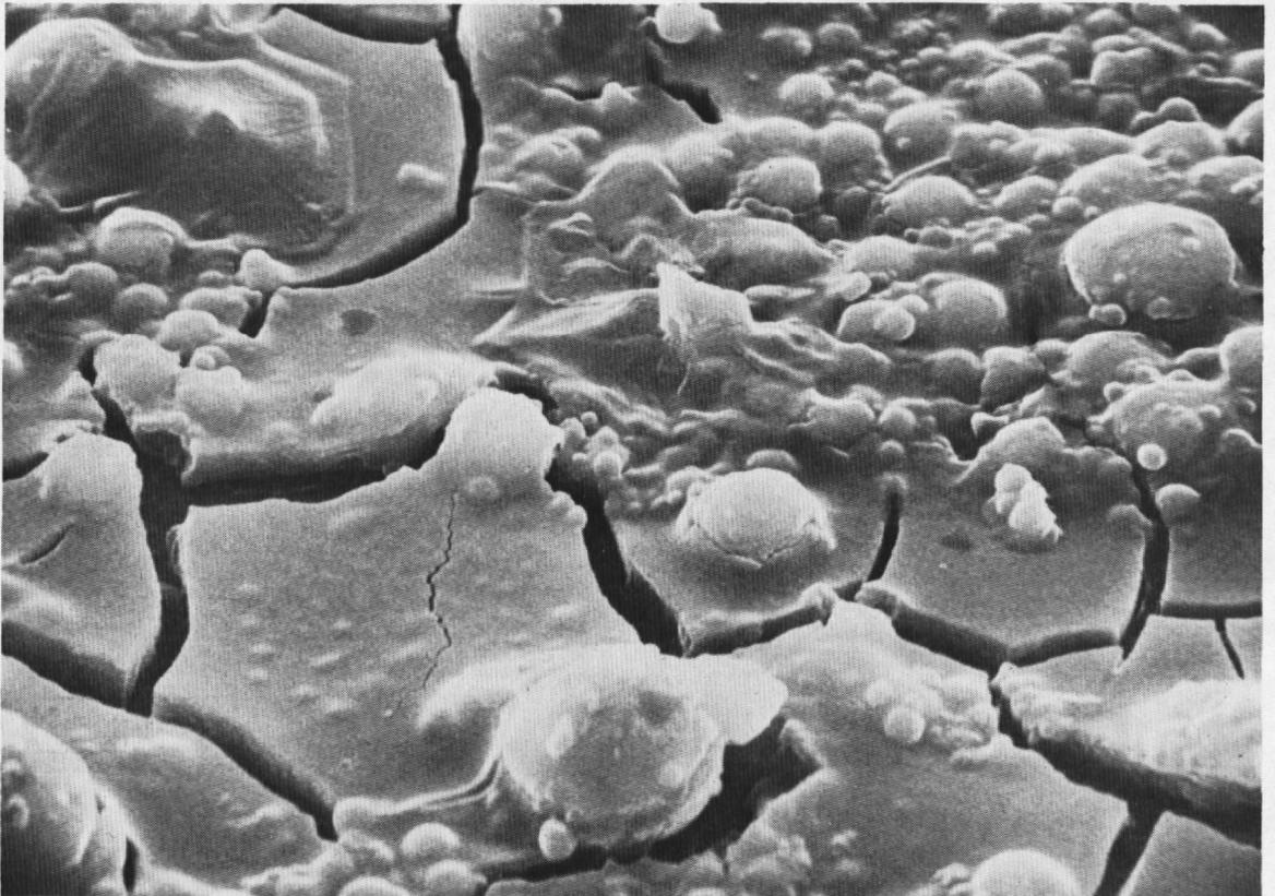
Figure 62. Aluminum chloride deposit.
