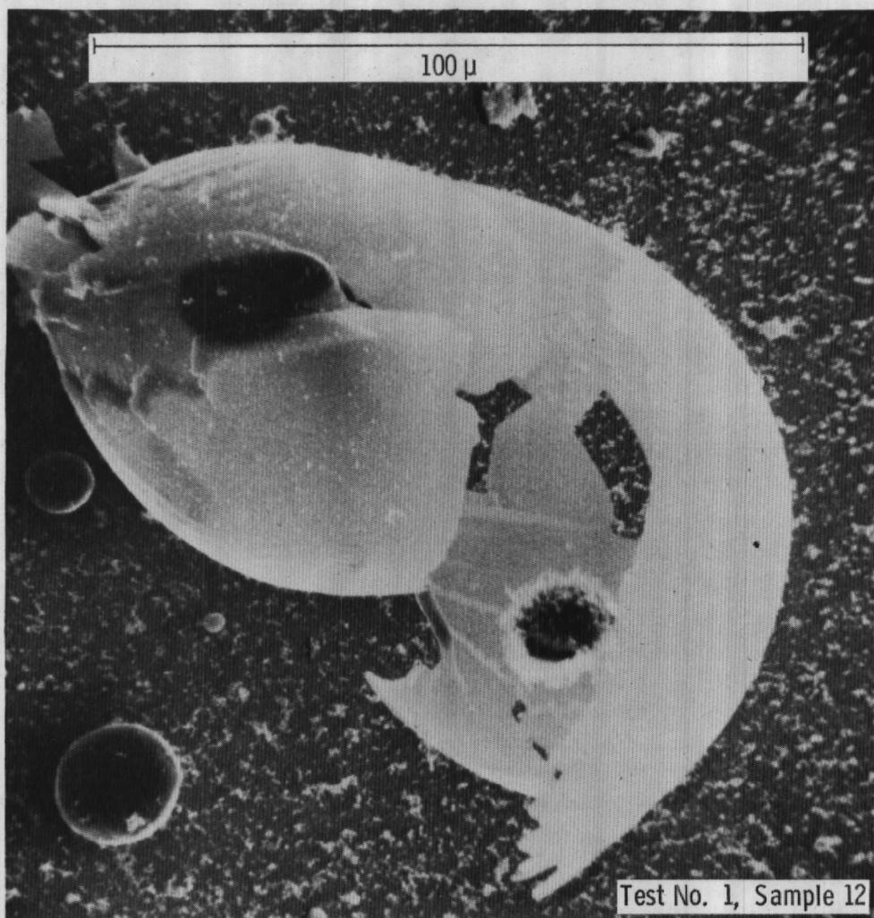
Figure 55. Broken Al<sub>2</sub>O<sub>3</sub> sphere.
