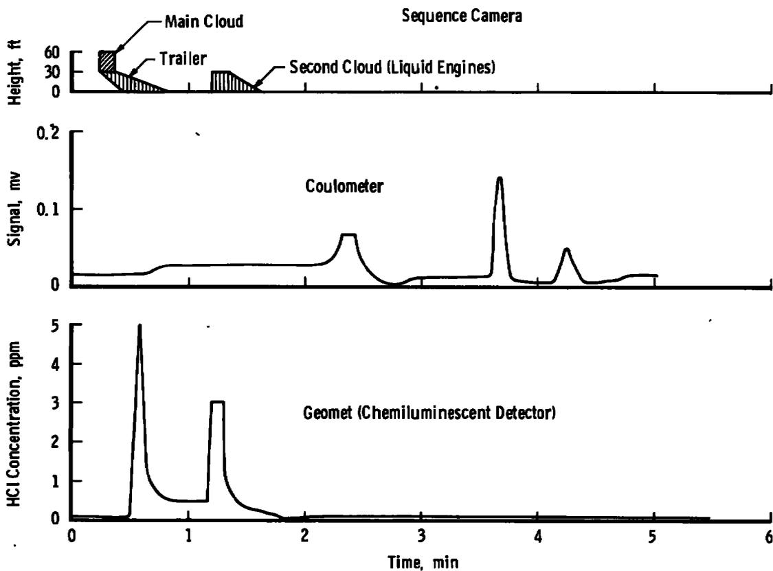
Figure 40. Comparison of HCl data MSFC Test No. 5.
