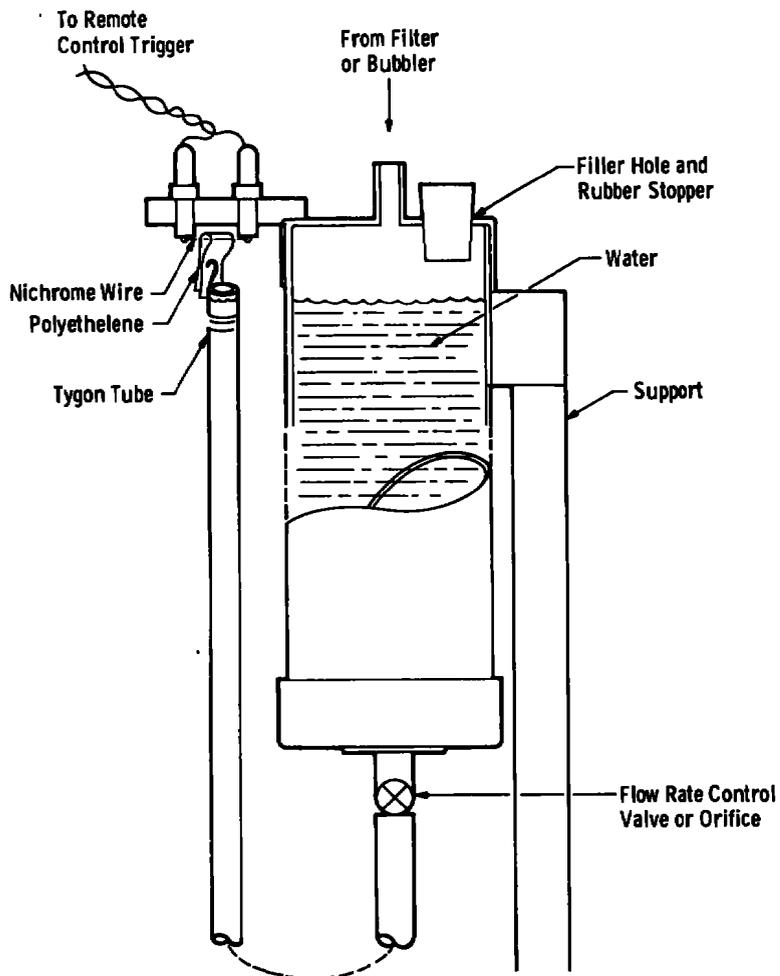
Figure 27. Water-driven sampling pump.
