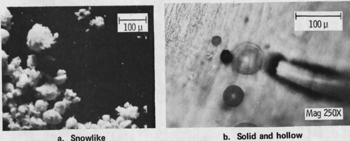
**Figure 54. Varieties of  $\text{Al}_2\text{O}_3$  spheres.**
