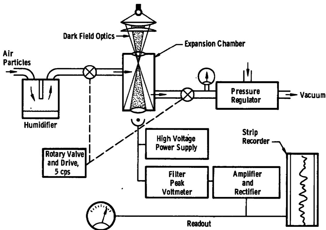
Figure 10. Schematic of condensation nuclei counter.
