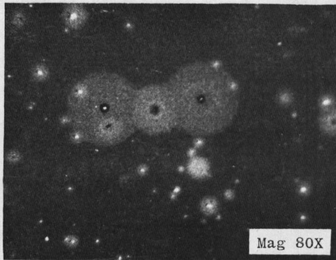
Figure 39. Optical microphotographs of acid droplet stains.
