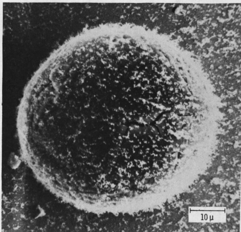
Figure 65.  $\text{Al}_2\text{O}_3$  particle with surface deposit.
