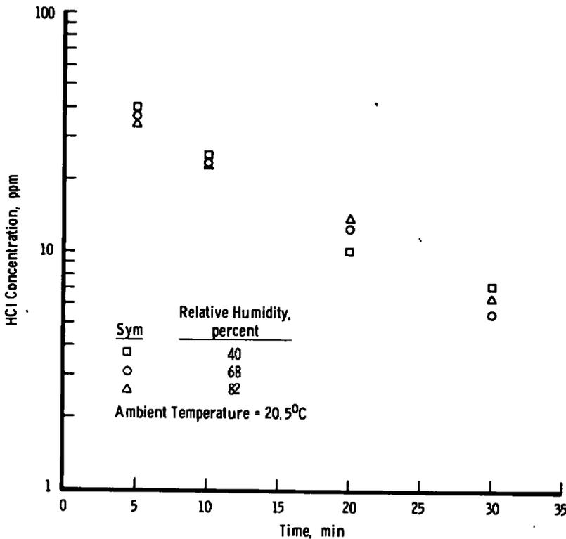
Figure 14. Decay of HCl gas released in chamber.
