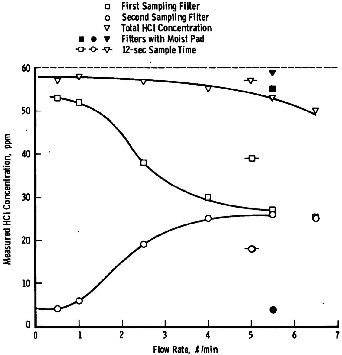
Figure 45. Evaluation of millipore filters as HCl detectors.
