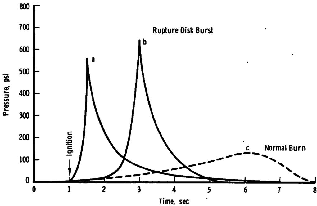
**Figure 3. Pressure profile with throat plugged.**
