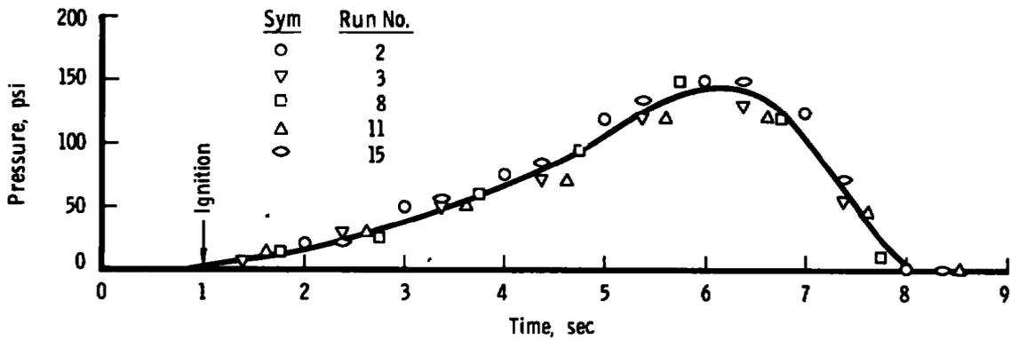
**Figure 4. Pressure profile during rocket burn.**
