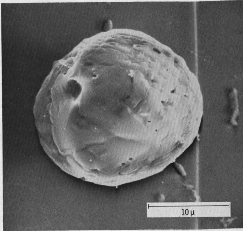
Figure 52. Fused  $\text{Al}_2\text{O}_3$  spheres.
