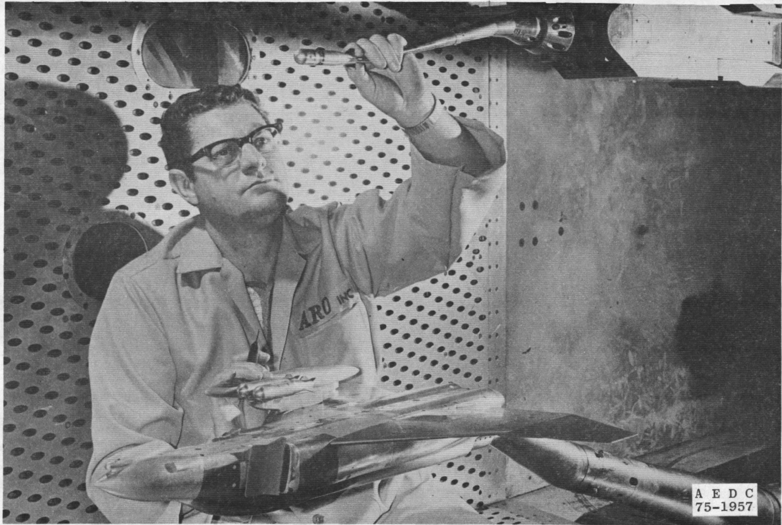
Figure 9. Tunnel installation photograph showing parent-aircraft model, a store model, and CTS.
