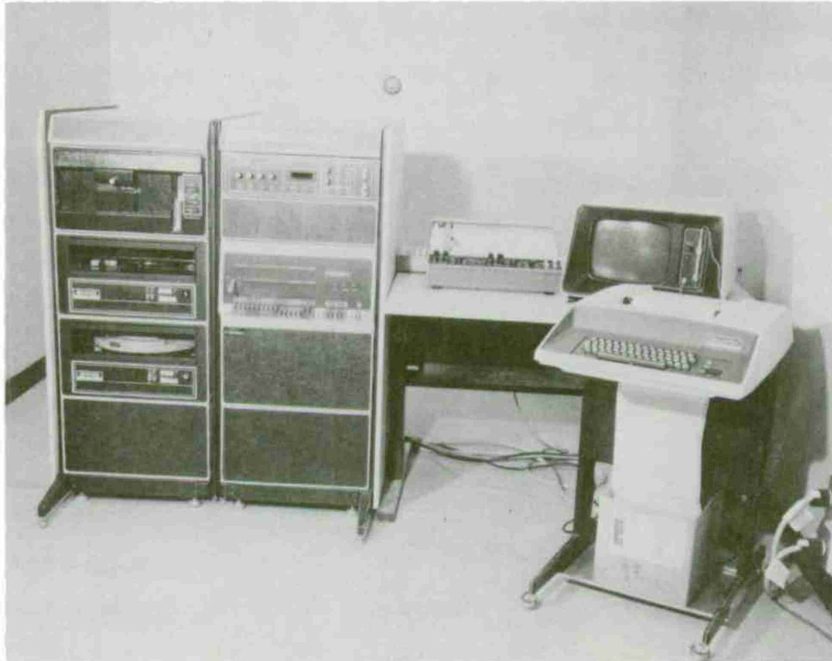
FIGURE 4. PDP-11/40 MINICOMPUTER SYSTEM WITH REFRESH GRAPHICS DISPLAY TERMINAL USED IN DEVELOPING THE "TRACKS" SYSTEM OF COMPUTER PROGRAMS
