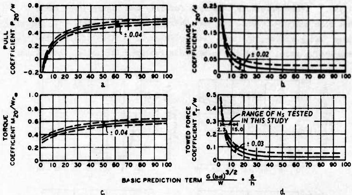
Figure 7. Relation of performance coefficients to sand mobility number for turn angle  $\alpha = 0$ ,  $v_w$  (wheel velocity) = 1.5 m/sec for powered condition, and  $v_a$  (carriage velocity) = 1.5 m/sec  $\approx v_w$  for towed condition<sup>21</sup>
