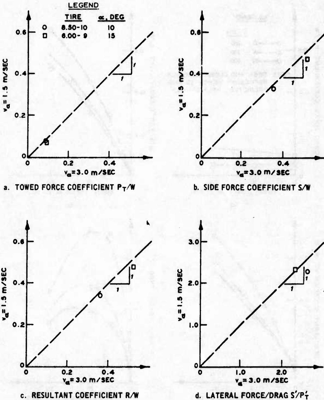
Figure 15. Comparison of performance parameters of the 8.50-10, 8-PR and 6.00-9, 4-PR tires operating under similar conditions at carriage velocities ( $v_a$ ) of 3.0 and 1.5 m/sec on clay
