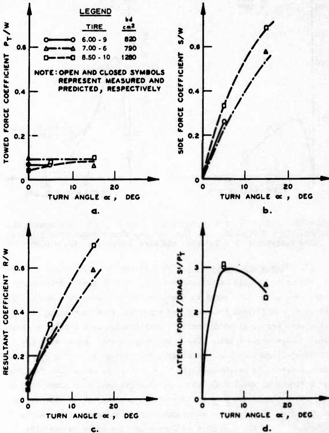
Figure 29. Influence of turn angle and tire width  $\times$  diameter ( $bd$ ) on performance parameters for three tires on clay. Tire deflection  $\delta/h = 0.35$ , average cone penetration resistance  $C = 350$  kPa, design wheel load  $W = 3000$  N
