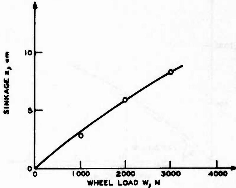
Figure 41. Sinkage as function of wheel load for 6.00-9, 4-PR tire at 15-deg turn angle on mortar sand with tire deflection  $\delta/h = 0.15$  and average penetration resistance gradient  $G = 2.6$  MPa/m
