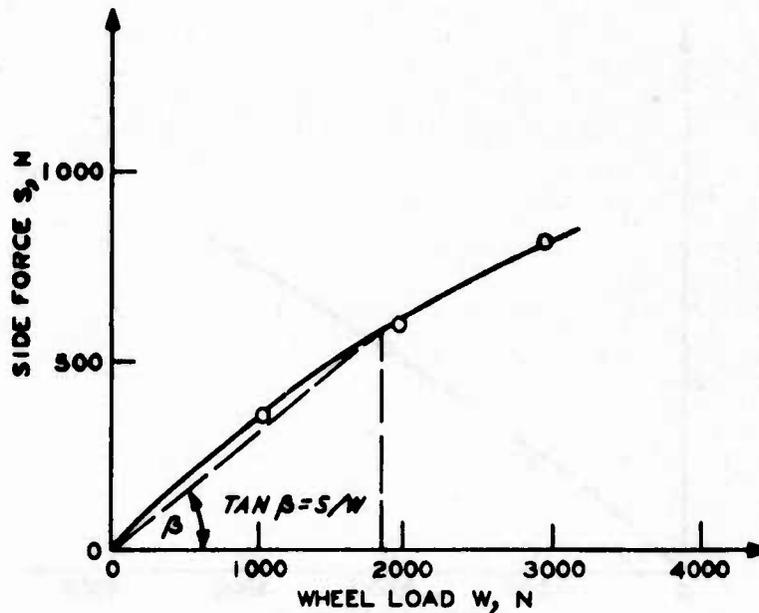
Figure 40. Side force as function of wheel load for 6.00-9, 4-PR tire at 15-deg turn angle on mortar sand with tire deflection  $\delta/h = 0.15$  and average penetration resistance gradient  $G = 2.6$  MPa/m
