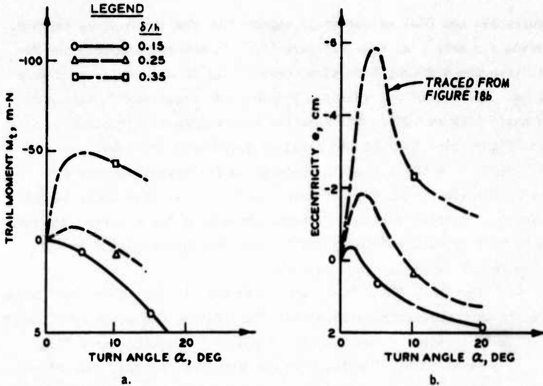
Figure 21. Influence of turn angle and tire deflection on trail moment and eccentricity for 8.50-10, 8-PR tire on clay with average cone penetration resistance  $C = 350$  kPa and design wheel load  $W' = 5800$  N
