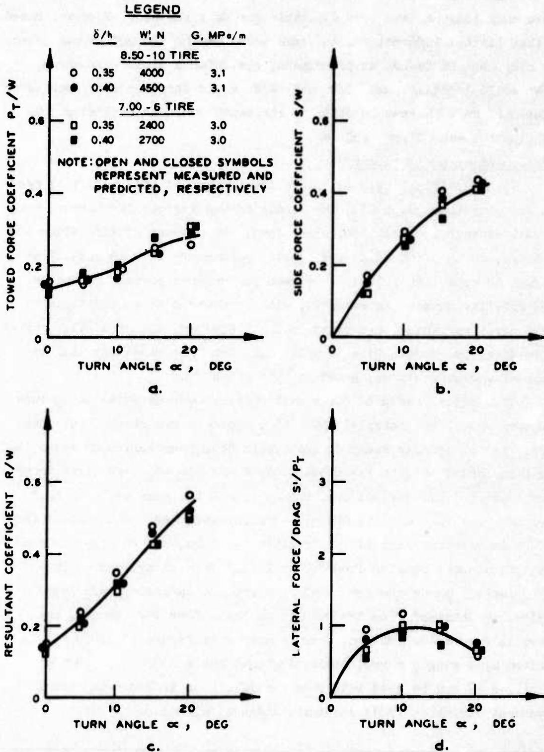
Figure 43. Relations between turn angle and performance parameters for two tires tested at various conditions resulting in average sand mobility number ( $N'_s$ ) of 10.4
