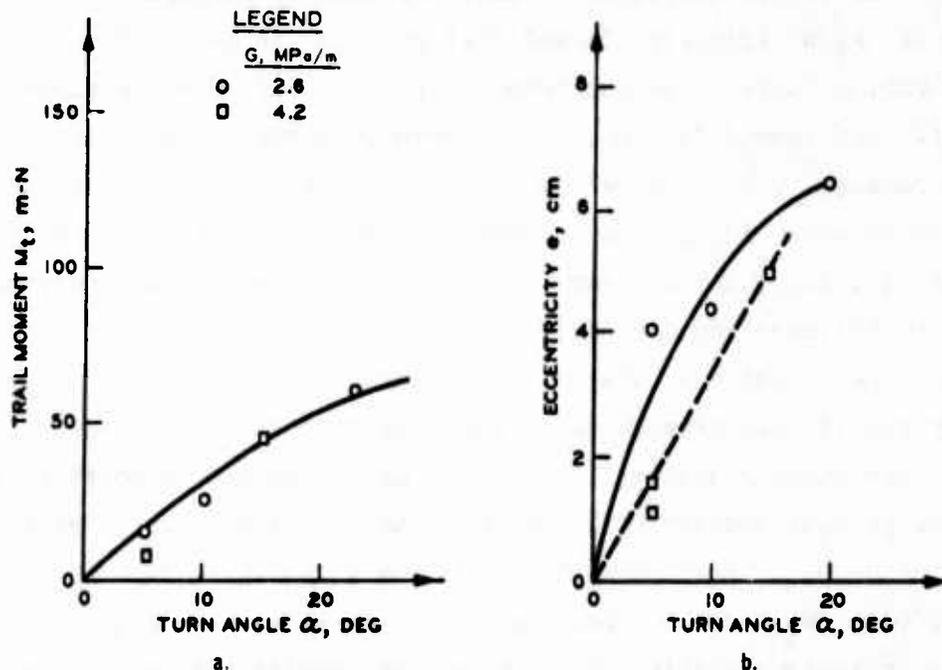
Figure 35. Influence of turn angle and soil strength on trail moment and eccentricity for 6.00-9, 4-PR tire on mortar sand with tire deflection  $\delta/h = 0.35$  and design wheel load  $W' = 2000$  N
