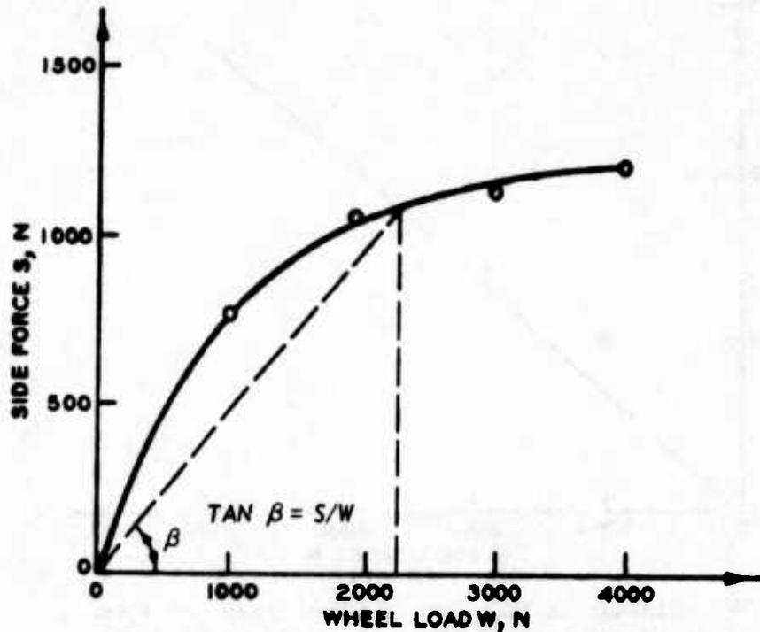
Figure 26. Side force as function of wheel load for 6.00-9, 4-PR tire at 10-deg turn angle on clay with tire deflection  $\delta/h = 0.25$  and average cone penetration resistance  $C = 350$  kPa
