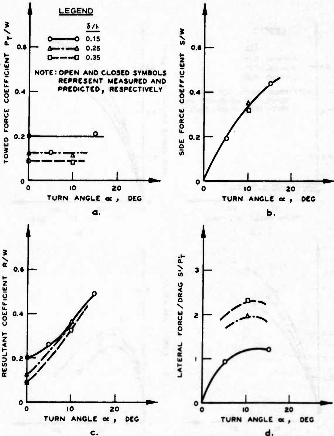
Figure 19. Influence of turn angle and tire deflection on performance parameters for 8.50-10, 8-PR tire on clay with average cone penetration resistance  $C = 350$  kPa and design wheel load  $W' = 5800$  N
