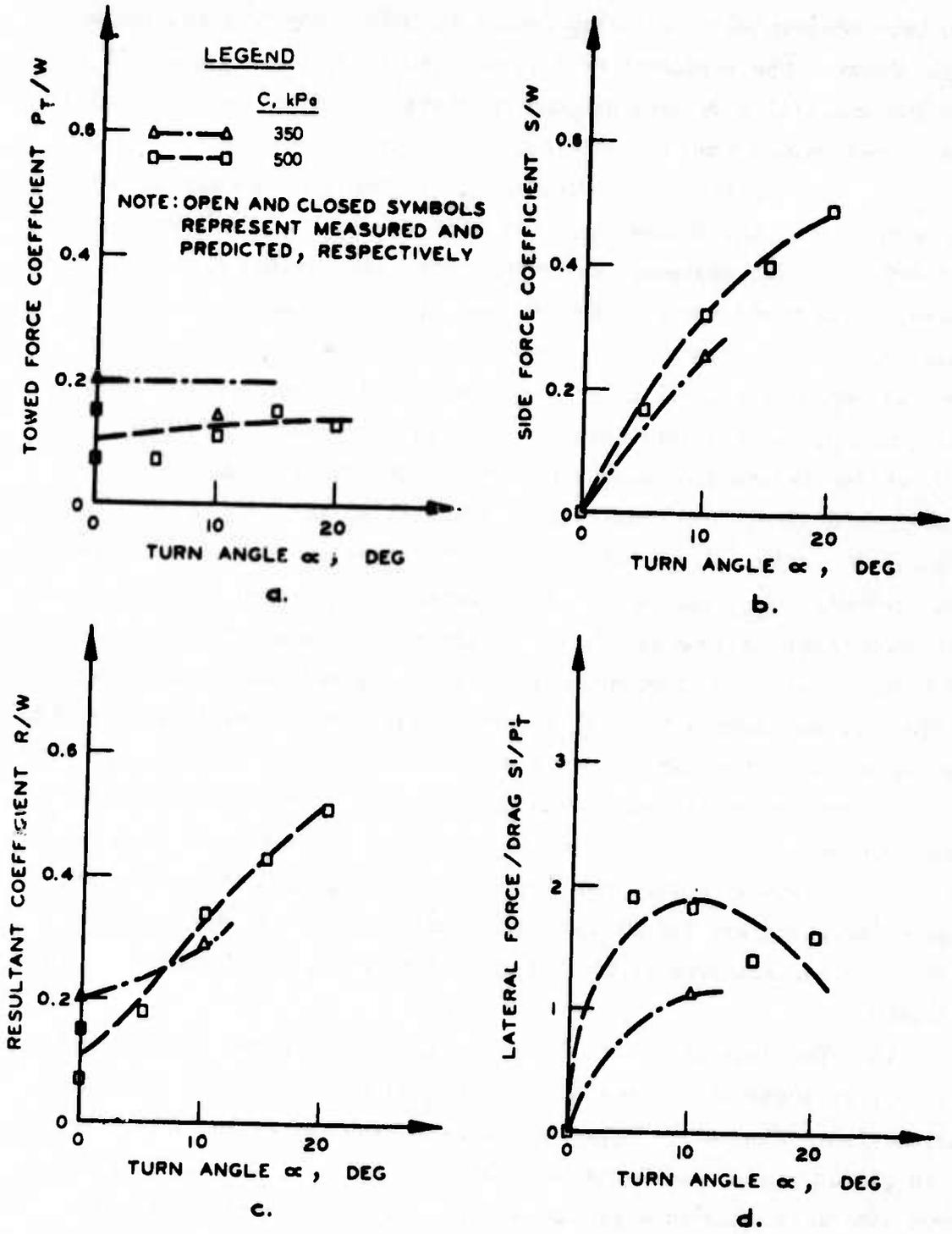
Figure 17. Influence of turn angle and soil strength on performance parameters for 7.00-6, 6-PR tire on clay with tire deflection  $\delta/h = 0.35$  and design wheel load  $W' = 5800$  N
