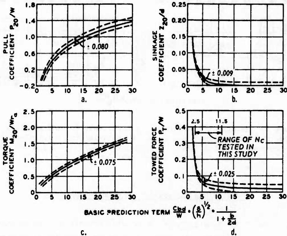
Figure 6. Relation of performance coefficients to clay mobility number for turn angle  $\alpha = 0$ ,  $v_w$  (wheel velocity) = 1.5 m/sec for powered condition, and  $v_a$  (carriage velocity) = 1.5 m/sec  $\approx v_w$  for towed condition<sup>21</sup>
