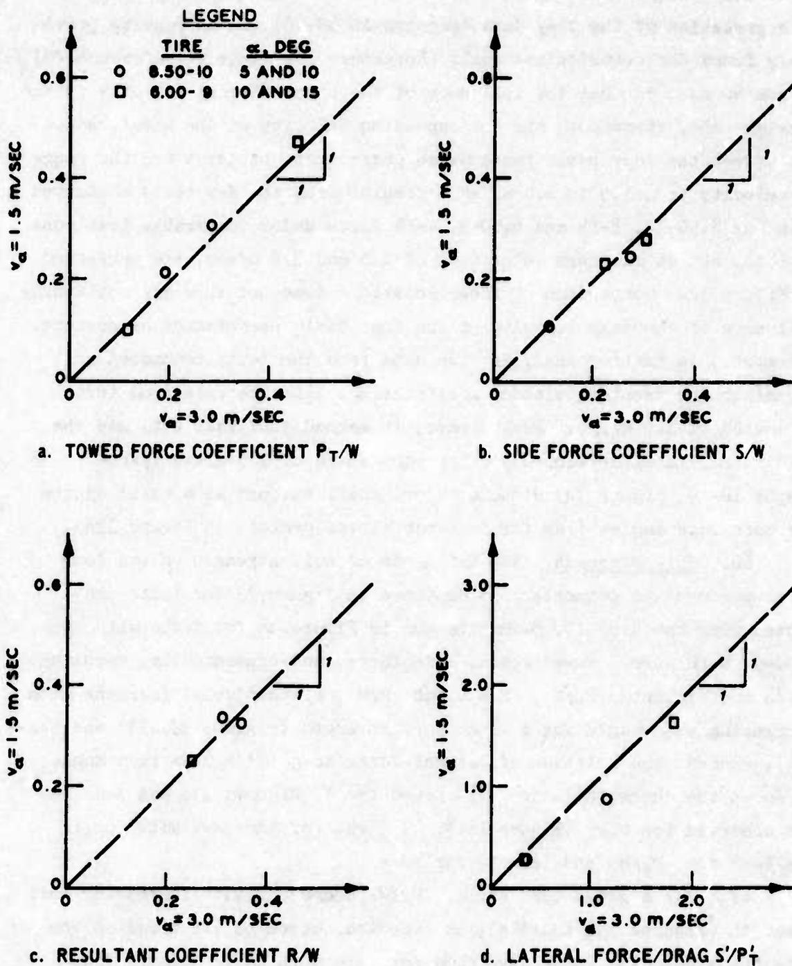
Figure 32. Comparison of performance parameters of 8.50-10, 8-PR and 6.00-9, 4-PR tires operating under similar conditions at carriage speeds ( $v_a$ ) of 3.0 m/sec and 1.5 m/sec on mortar sand
