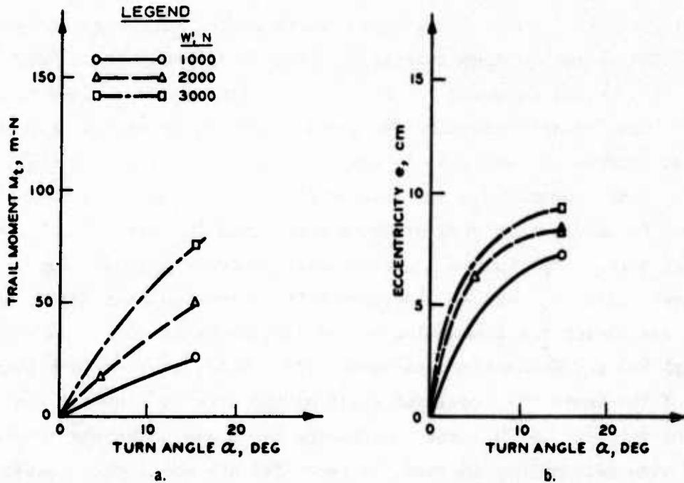
Figure 42. Influence of turn angle and wheel load on trail moment and eccentricity for 6.00-9, 4-PR tire on mortar sand with average penetration resistance gradient  $G = 2.6$  MPa/m and tire deflection  $\delta/h = 0.15$
