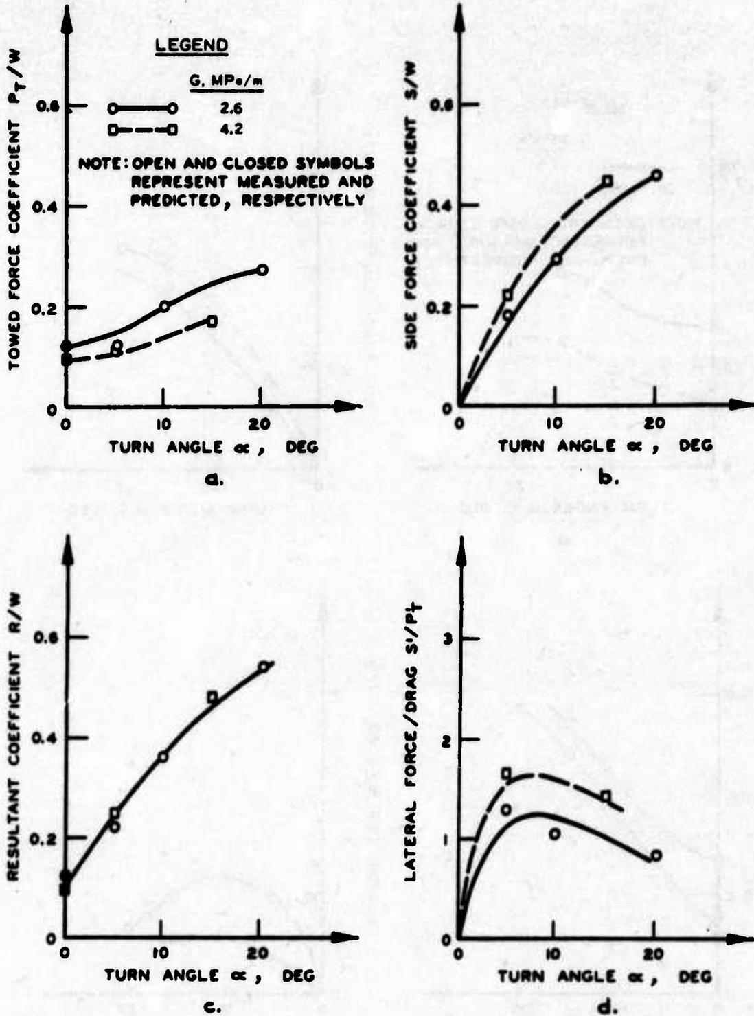
Figure 34. Influence of turn angle and soil strength on performance parameters for 6.00-9, 4-PR tire on mortar sand with tire deflection  $\delta/h = 0.35$  and design wheel load  $W' = 2000$  N
