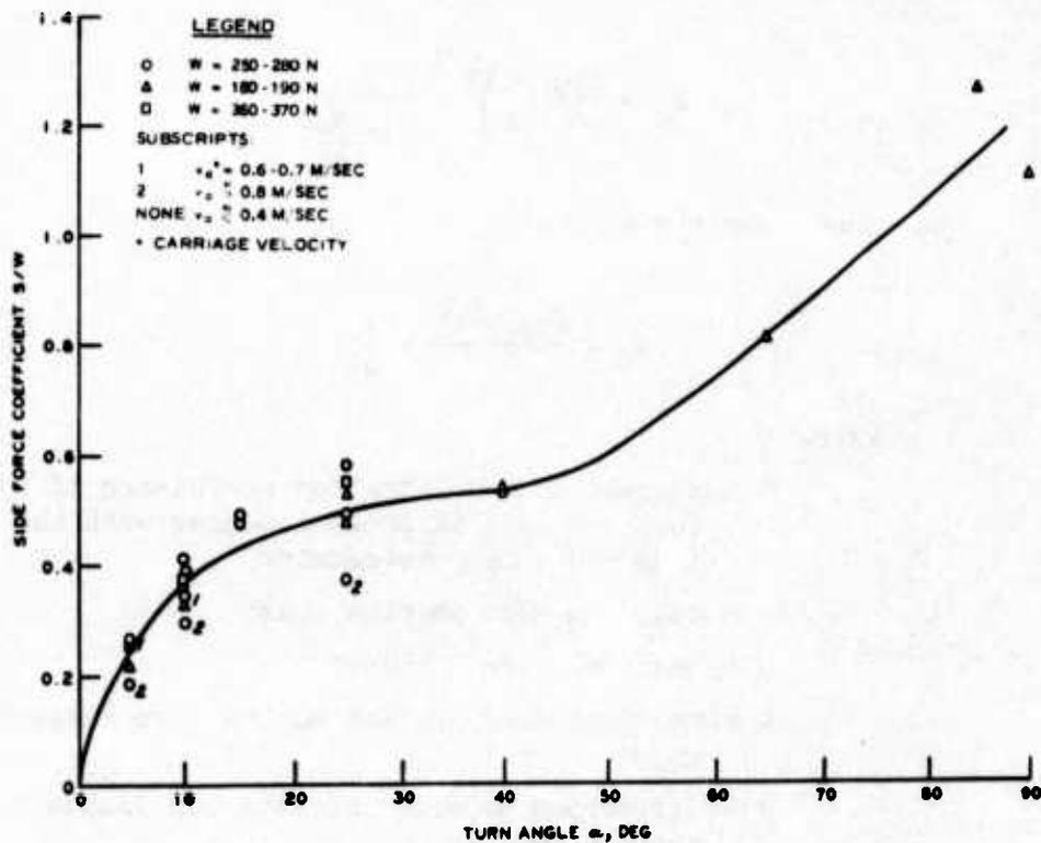
Figure 5. Turn angle versus side force coefficient for the LRV wheel<sup>15</sup>
