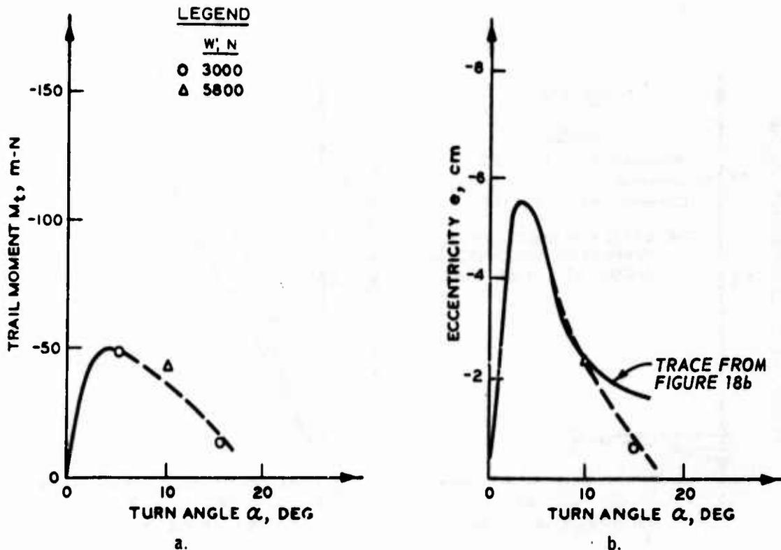
Figure 28. Influence of turn angle and wheel load on trail moment and eccentricity for 8.50-10, 8-PR tire on clay with average cone penetration resistance  $C = 350$  kPa and tire deflection  $\delta/h = 0.35$
