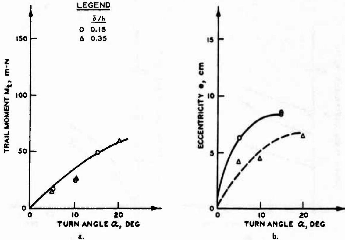
Figure 38. Influence of turn angle and deflection on trail moment and eccentricity for 6.00-9, 4-PR tire on mortar sand with average penetration resistance gradient  $G = 2.6$  MPa/m and design wheel load  $W' = 2000$  N
