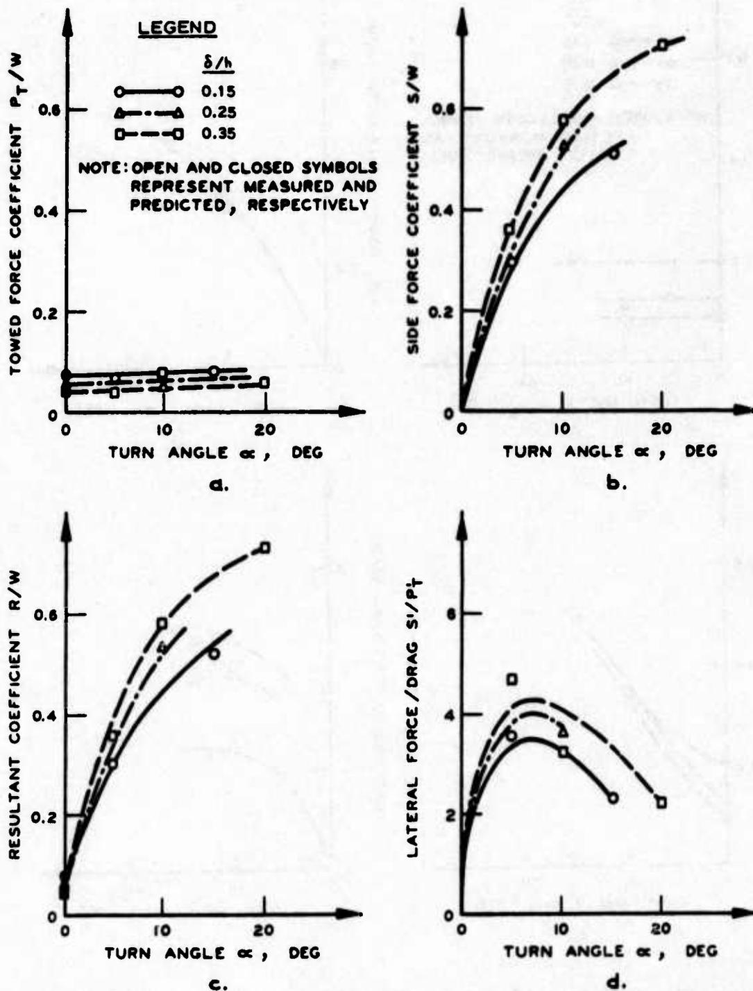
Figure 20. Influence of turn angle and tire deflection on performance parameters for 6.00-9, 4-PR tire on clay with average cone penetration resistance  $C = 350$  kPa and design wheel load  $W' = 2000$  N
