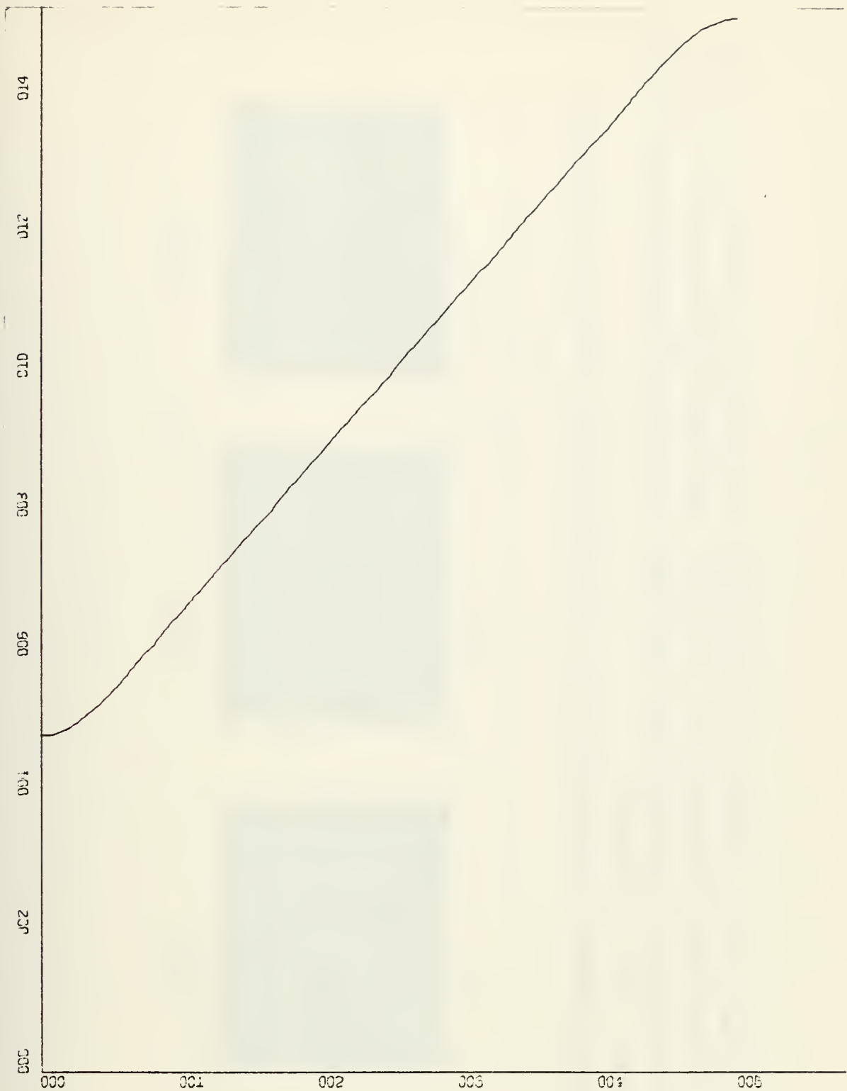
FIGURE 4.1 Theoretical Amplitude Frequency Response of Prewhitening Filter. Length = 11. Hamming window.
