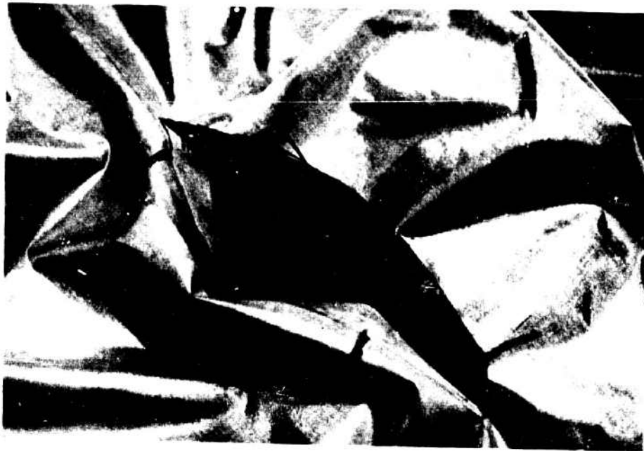
Figure 12. Close-Up of Bladder Failure after Removing the Bladder from Air Chamber 1 of Shelter Section F-2
