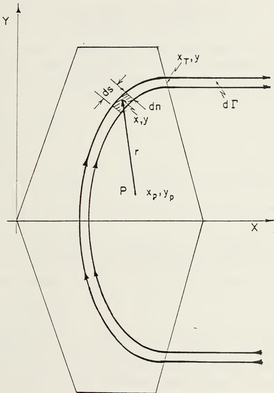
Fig. 5 Induced velocity in the x-y plane
