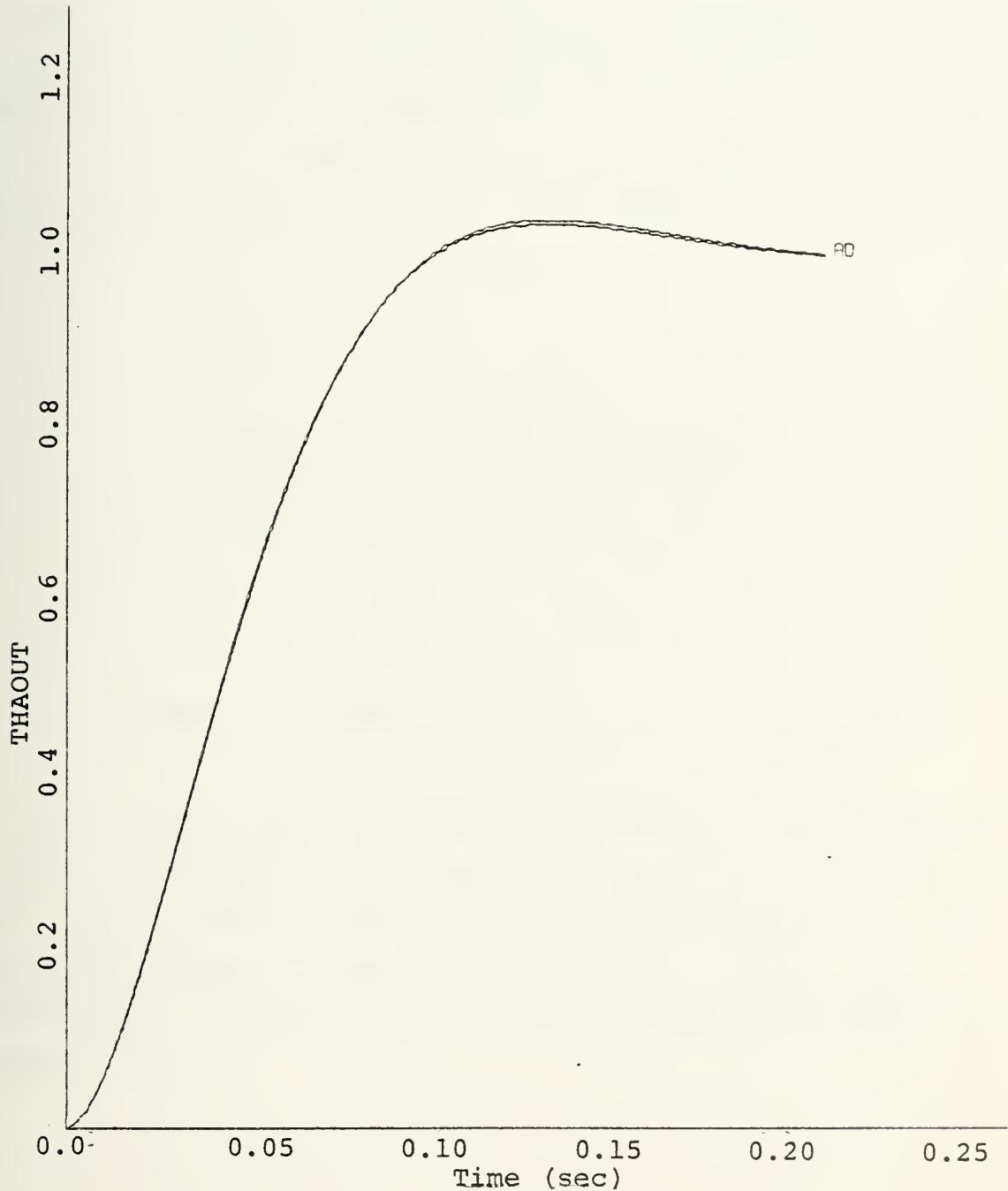
FIGURE 9 Pseudo Tachometer Compensated System's Response
