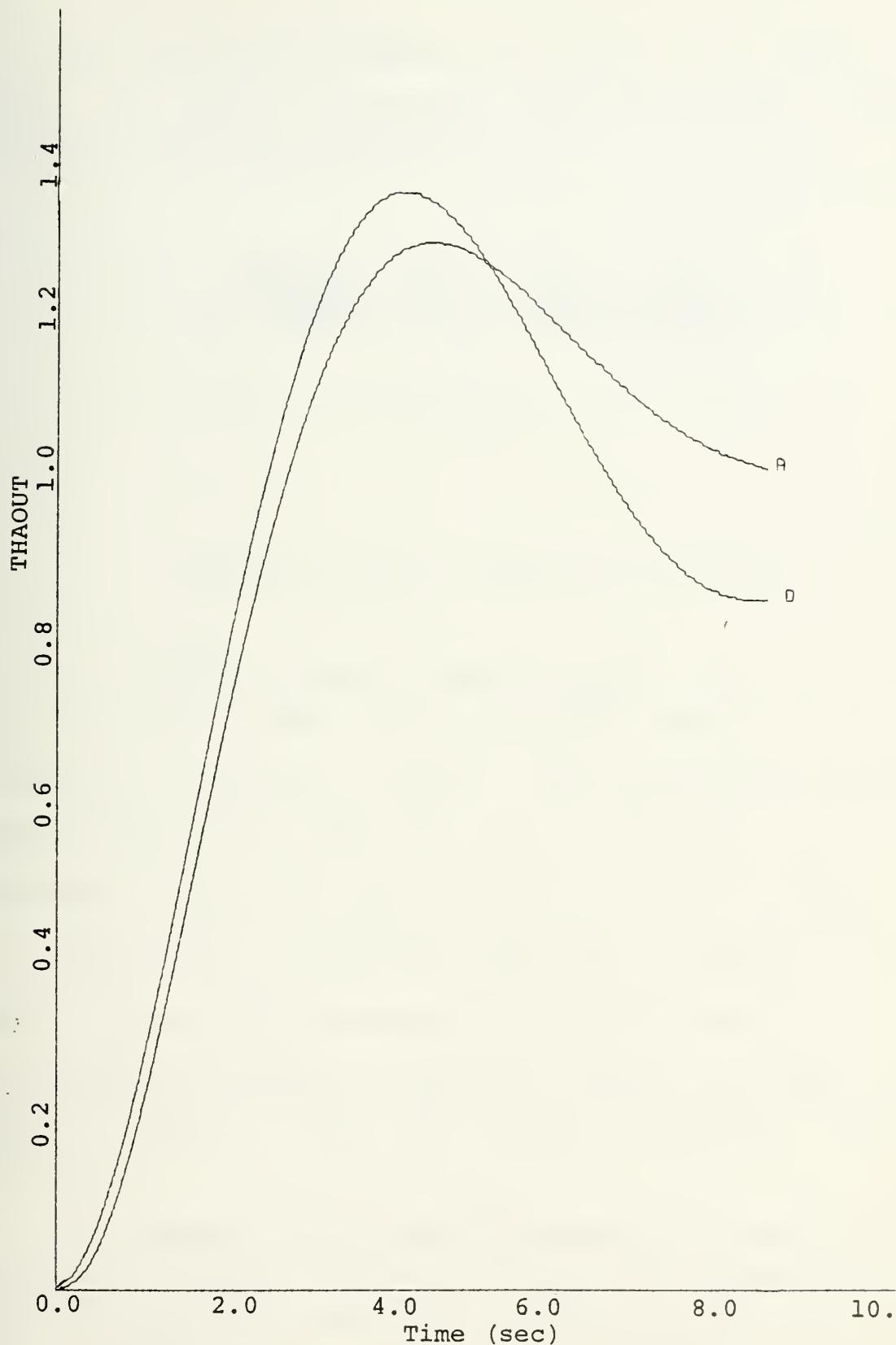
FIGURE 13 Conventionally Compensated System Response
