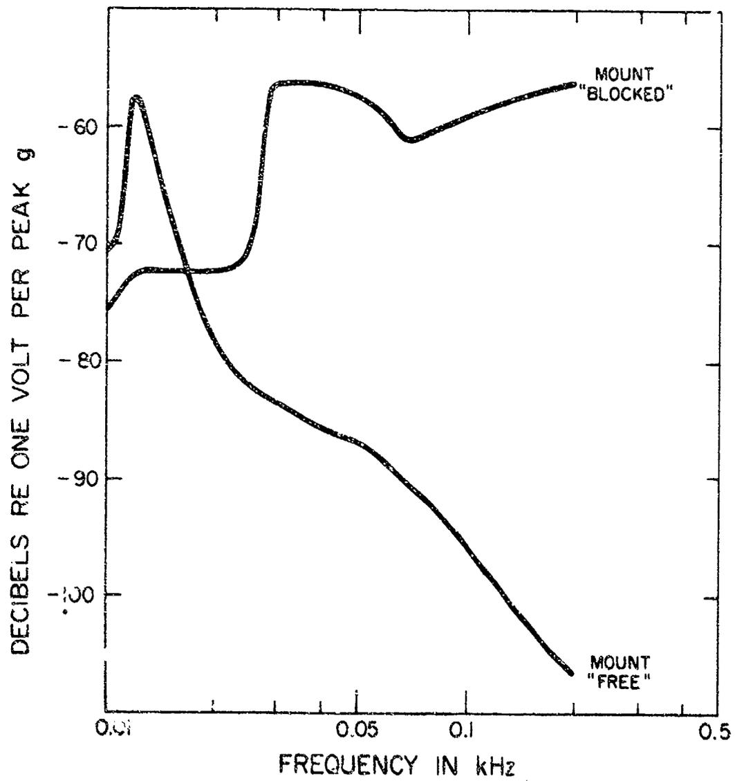
Fig. 4 - Hydrophone acceleration sensitivity
