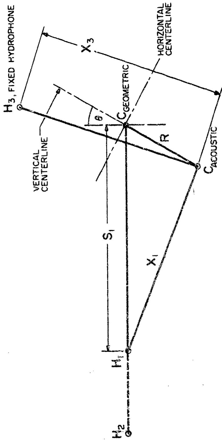
Fig. 3 -- Geometry, one towed, one fixed hydrophone
