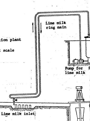
Waste water neutralization plant Schematic view without scale
