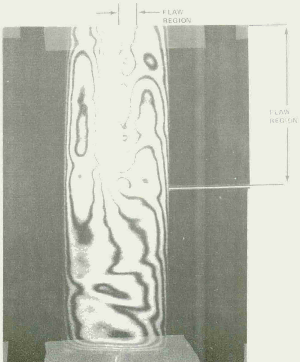
Figure 16. Fringe pattern for the cylinder with a longitudinal flaw.
