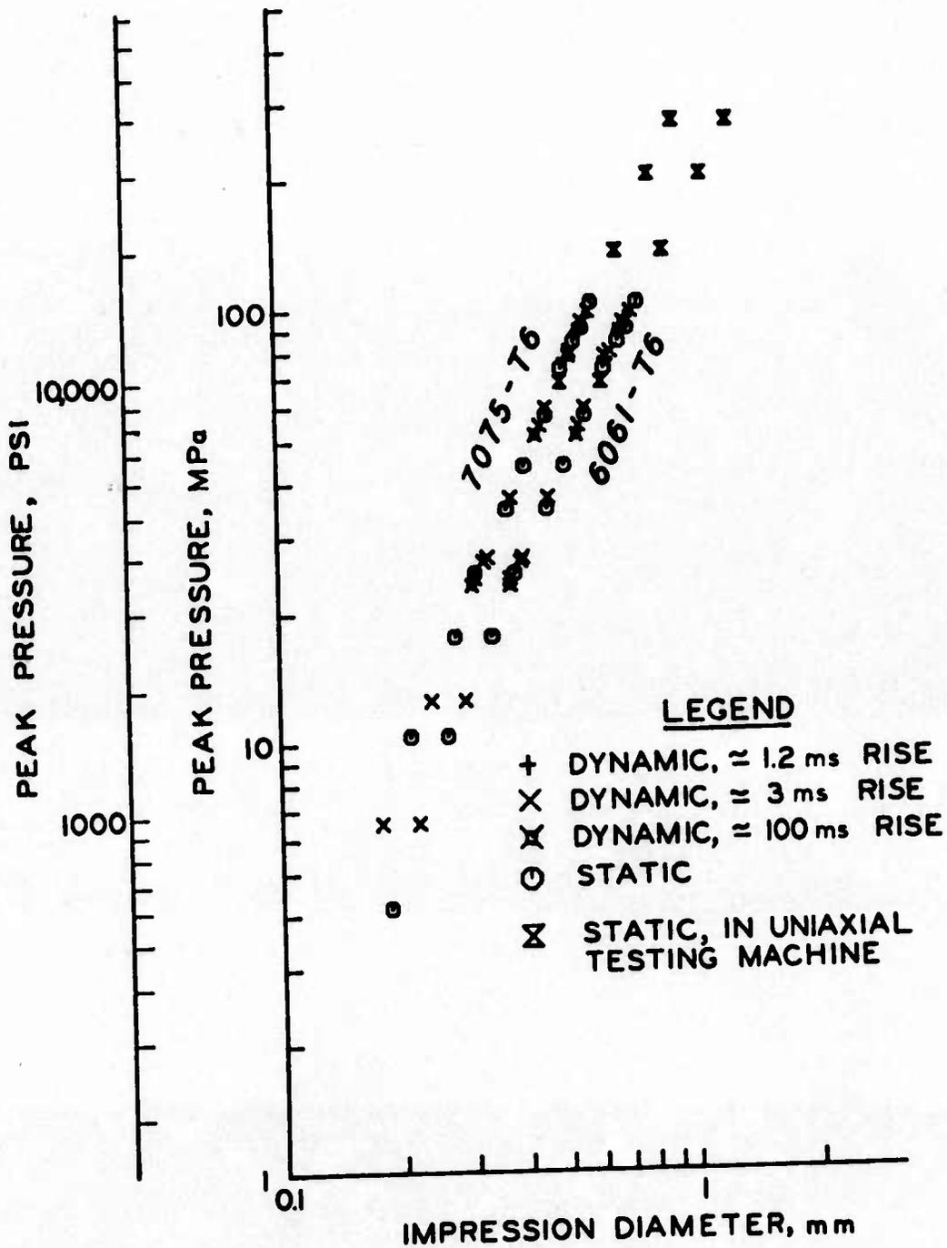
Figure 4. Calibrations in hydraulic fluid for the high-ranged Brinell Sandwich soil stress gage, with the steel balls closely packed.
