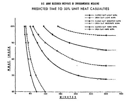
'Fig. 1 Prediction graph for 50 per cent unit survival time for CB protective uniforms with reduced water vapor permeability. "Light work" is 200 kcal/hr., and "hard work" is 300 kcal/hr.
