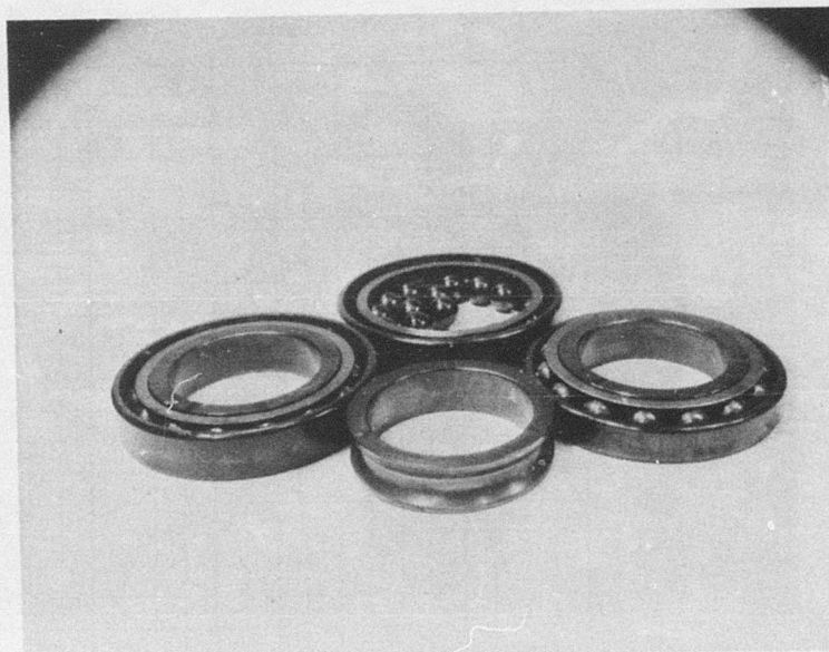
Figure 75. Main input triplex bearing following 4.0-hour emergency lubrication run.
