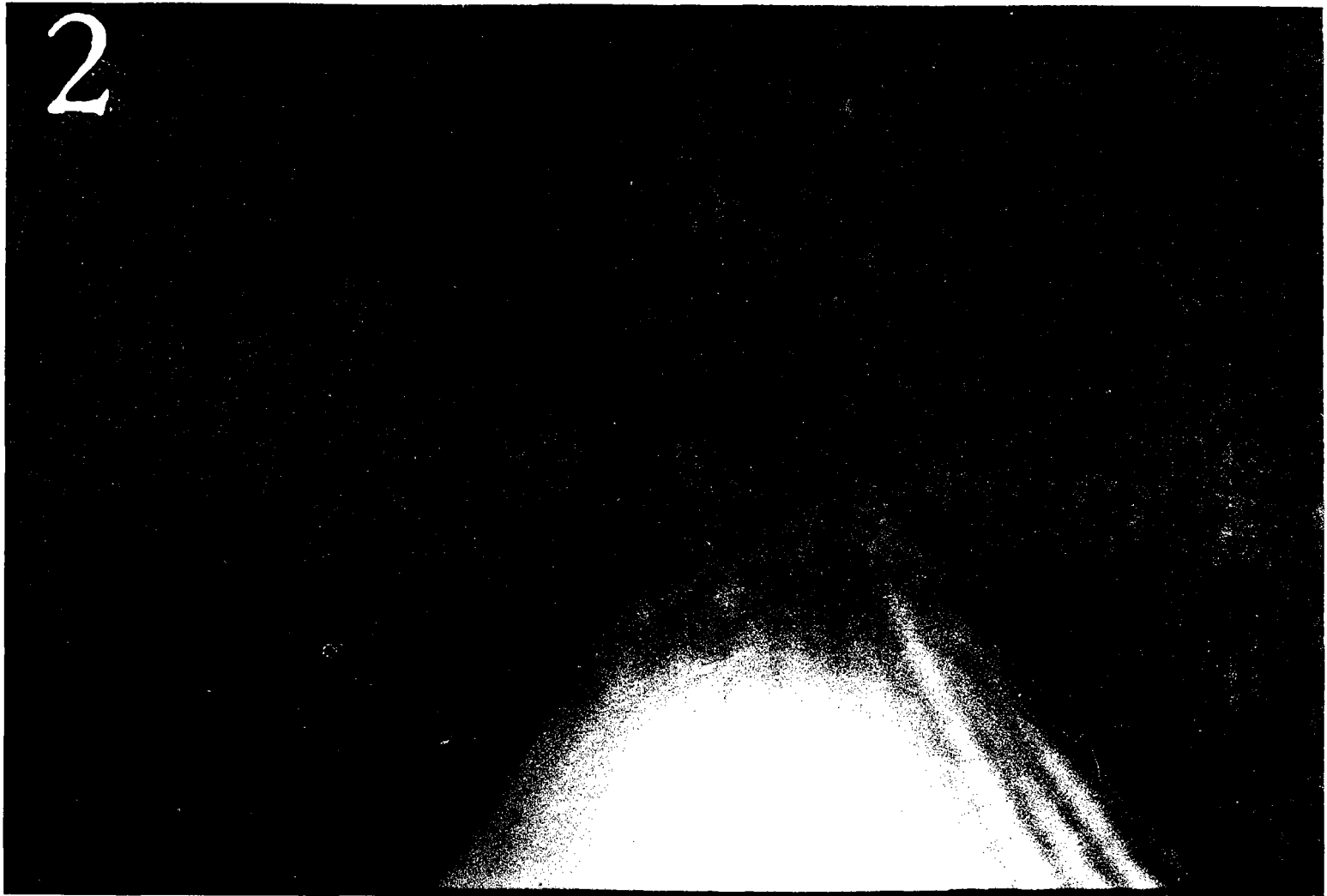
FIGURE 5. Windscreen glare with Solution 1 (metal shield beneath landing light) applied. Aircraft is over white runway markers (rectangular stripes in background).
