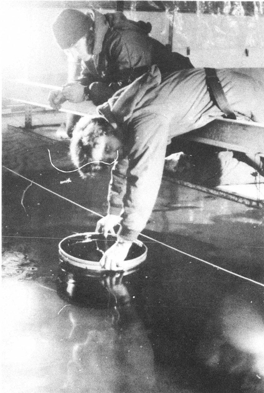
FIGURE 16. PHOTOGRAPH OF THE CRUDE OIL OPEN WATER SPREADING TEST JUST PRIOR TO RELEASE OF THE OIL .
