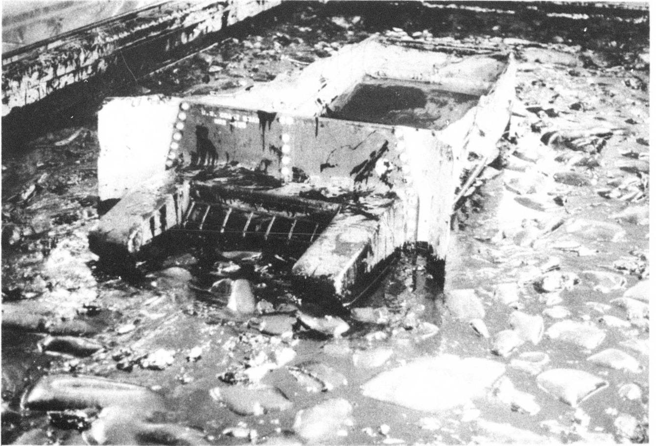
FIGURE 32. PHOTOGRAPH OF THE OSI SKIMMER READIED FOR TESTING IN ICE INFESTED WATER AND CRUDE OIL.
