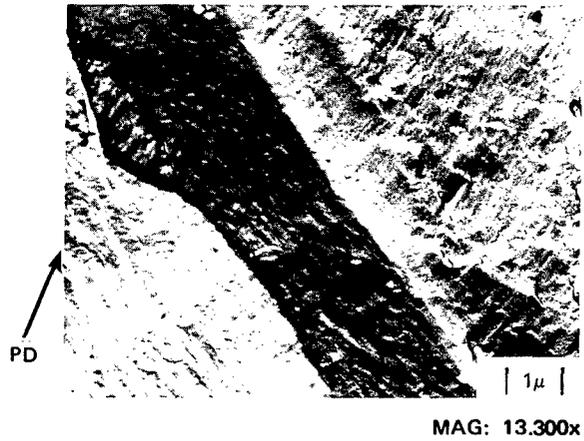
Peak load plastic zone showing well-defined fatigue striations before and poorly defined striations after.
