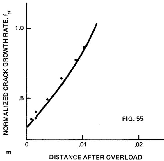
Figure 61 Comparison of Equation 14 with Data (Sheet 3 of 3)
