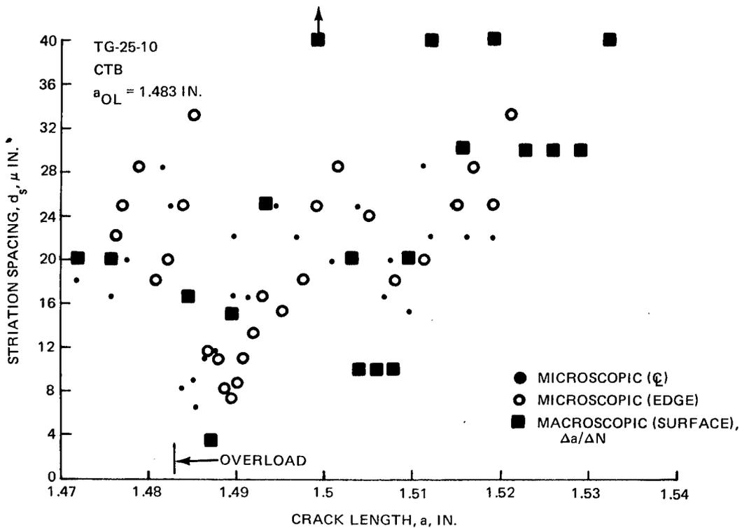
Figure 18 Striation Spacing and  $\Delta a/\Delta N$  vs Crack Length, Ti 6Al-4V Titanium, O/L = 1.5
