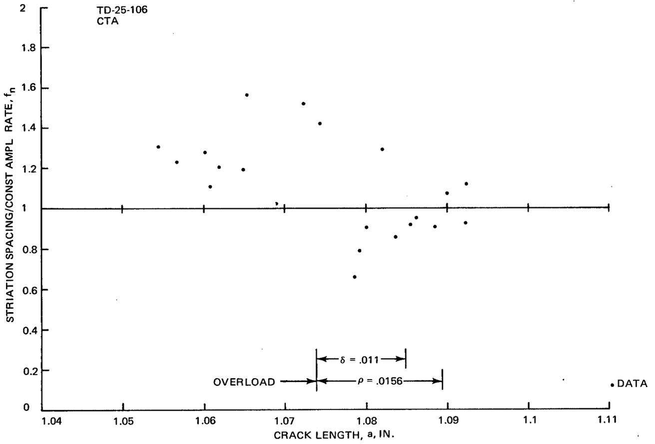
Figure 53 Delayed Retardation,  $a_{OL} = 1.074$  In., Centerline, O/L = 1.8, Ti 6Al-4V Titanium
