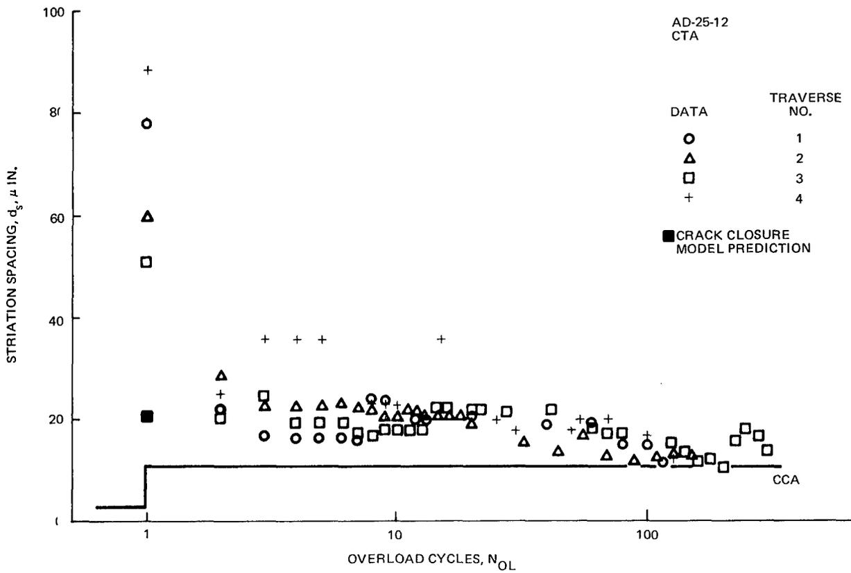
Figure 68 Acceleration,  $a_{OL} = 1.069 \text{ in.}$ ,  $O/L = 1.5$ , 2219-T851 Aluminum
