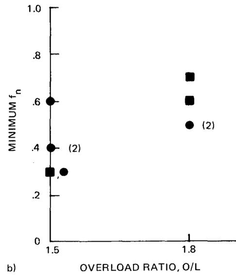
Figure 56 Delayed Retardation Parameters (Sheet 1 of 2)
