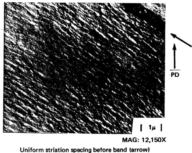
Figure A-14 Single Periodic Overloads,  $a_{ref} = 1.44$  In., Centerline,  $O/L = 1.25$ ,  $N_{OL}/N = 1/50$ , 2219-T851 Aluminum
