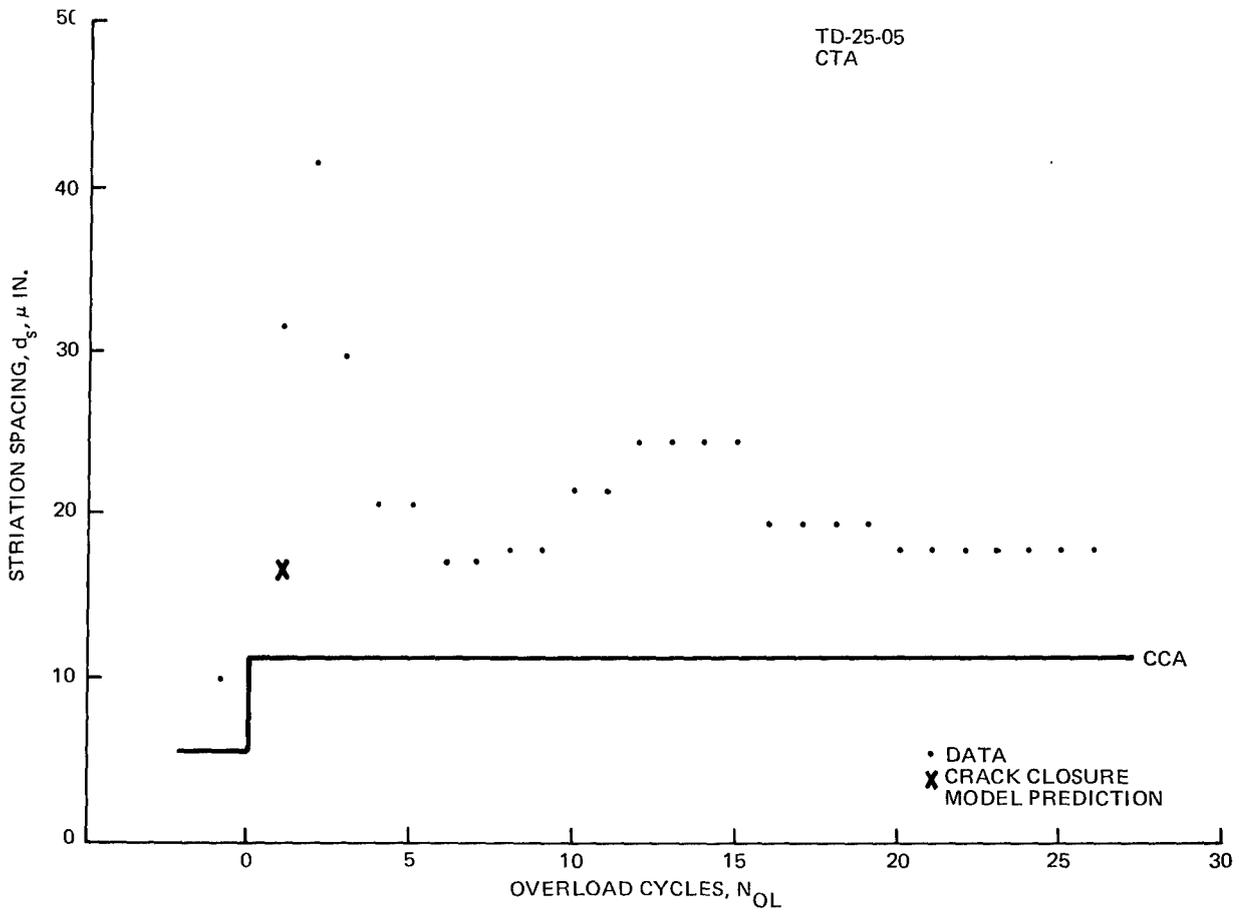
Figure 70 Acceleration,  $a_{OL} = 1.418$  In., O/L = 1.25, Ti 6Al-4V Titanium
