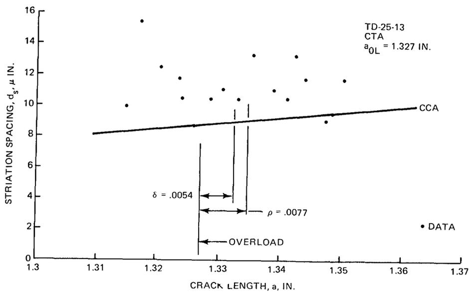
Figure 26 Affected Crack Length, Centerline, O/L = 1.25, Ti 6Al-4V Titanium
