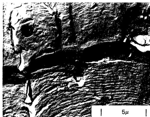
Peak load plastic zone showing well-defined fatigue striations before and poorly defined striations after.
