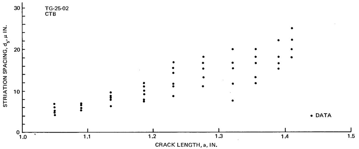
Figure 9 Striation Spacing vs Crack Length, Ti 6Al-4V Titanium, Constant Amplitude, R = 0.05
