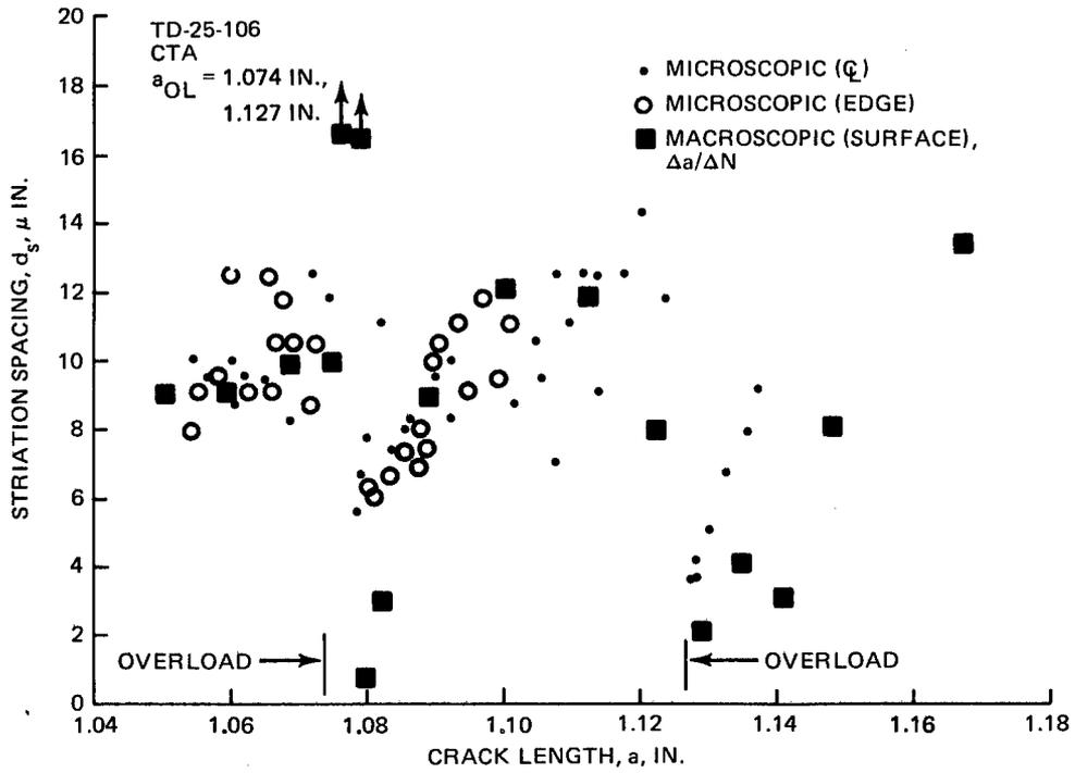
Figure 19 Striation Spacing and  $\Delta a/\Delta N$  vs Crack Length, O/L = 1.8, Ti 6Al-4V Titanium
