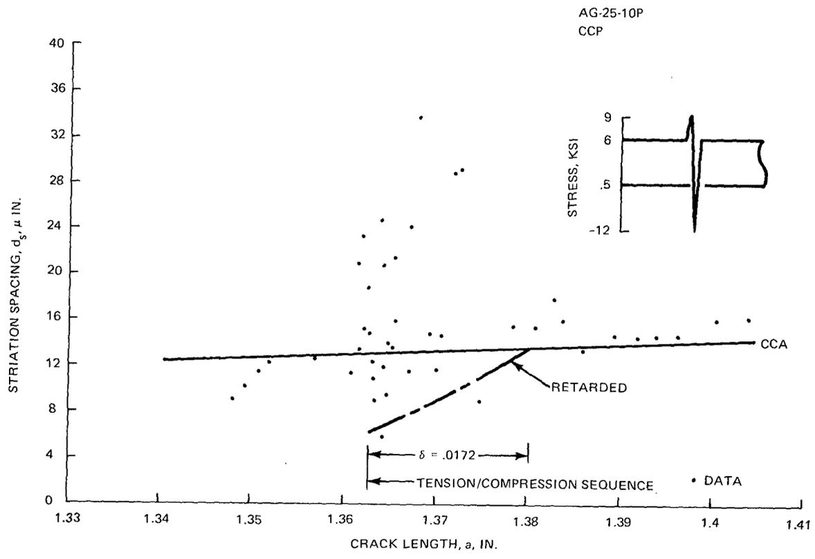
Figure 82 Tension/Compression,  $O/L = 1.5$ ,  $R_C = -2$ ,  $a_{ref} = 1.363$  In., 2219-T851 Aluminum
