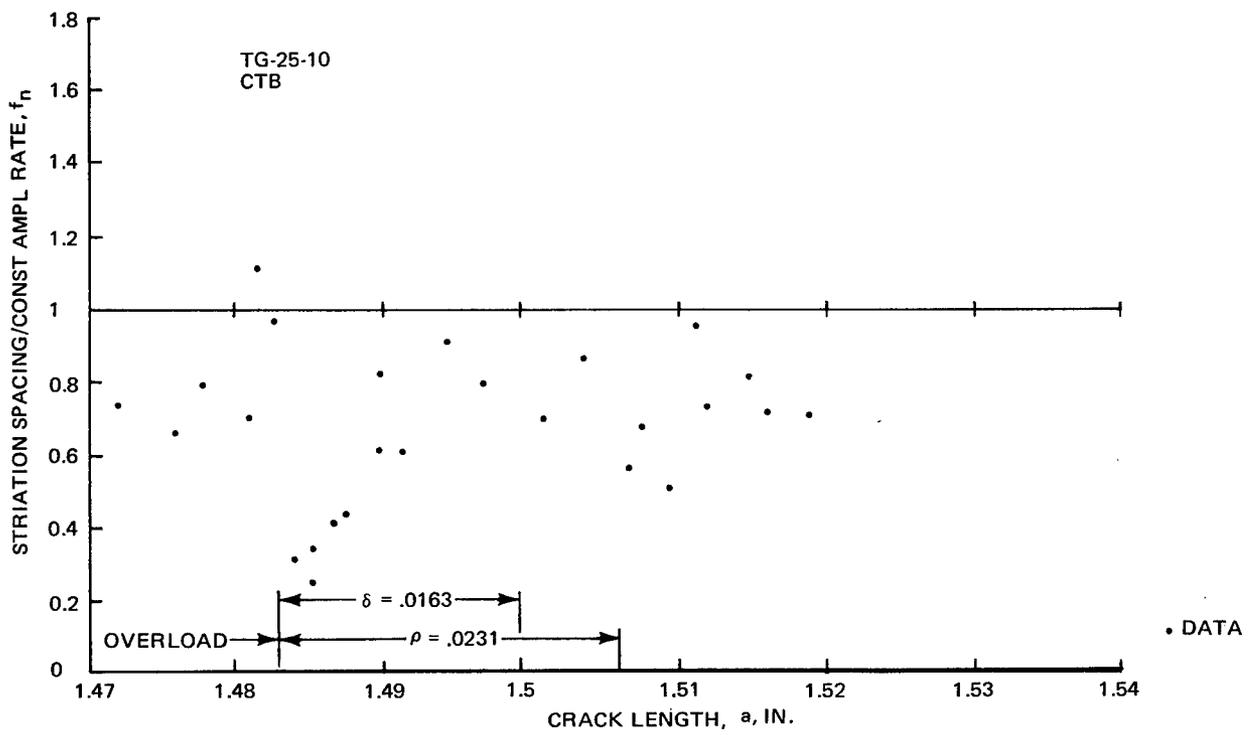
Figure 49 Delayed Retardation,  $a_{OL} = 1.483$  In., Centerline, O/L = 1.5, Ti 6Al-4V Titanium
