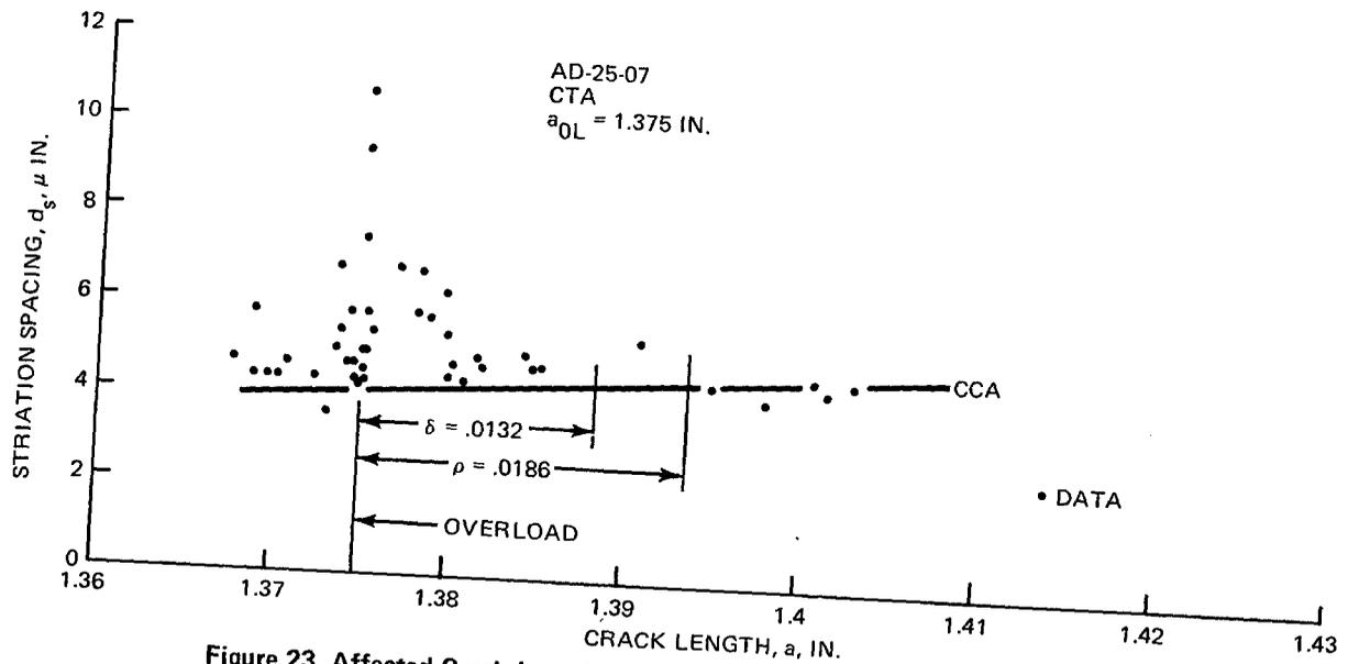
Figure 23 Affected Crack Length, Centerline, O/L = 1.8, 2219-T851 Aluminum
