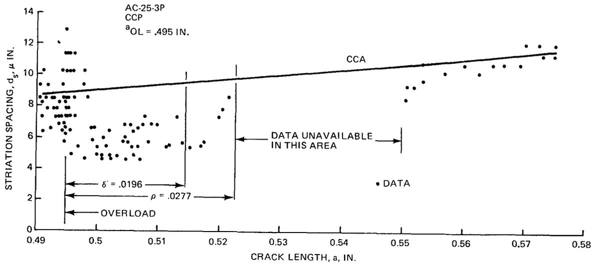
Figure 25 Affected Crack Length, Centerline, O/L = 1.8, 2219-T851 Aluminum
