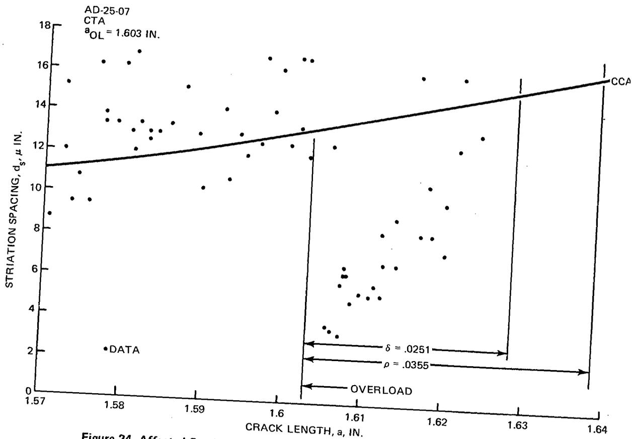
Figure 24 Affected Crack Length, Centerline, O/L = 1.8, 2219-T851 Aluminum
