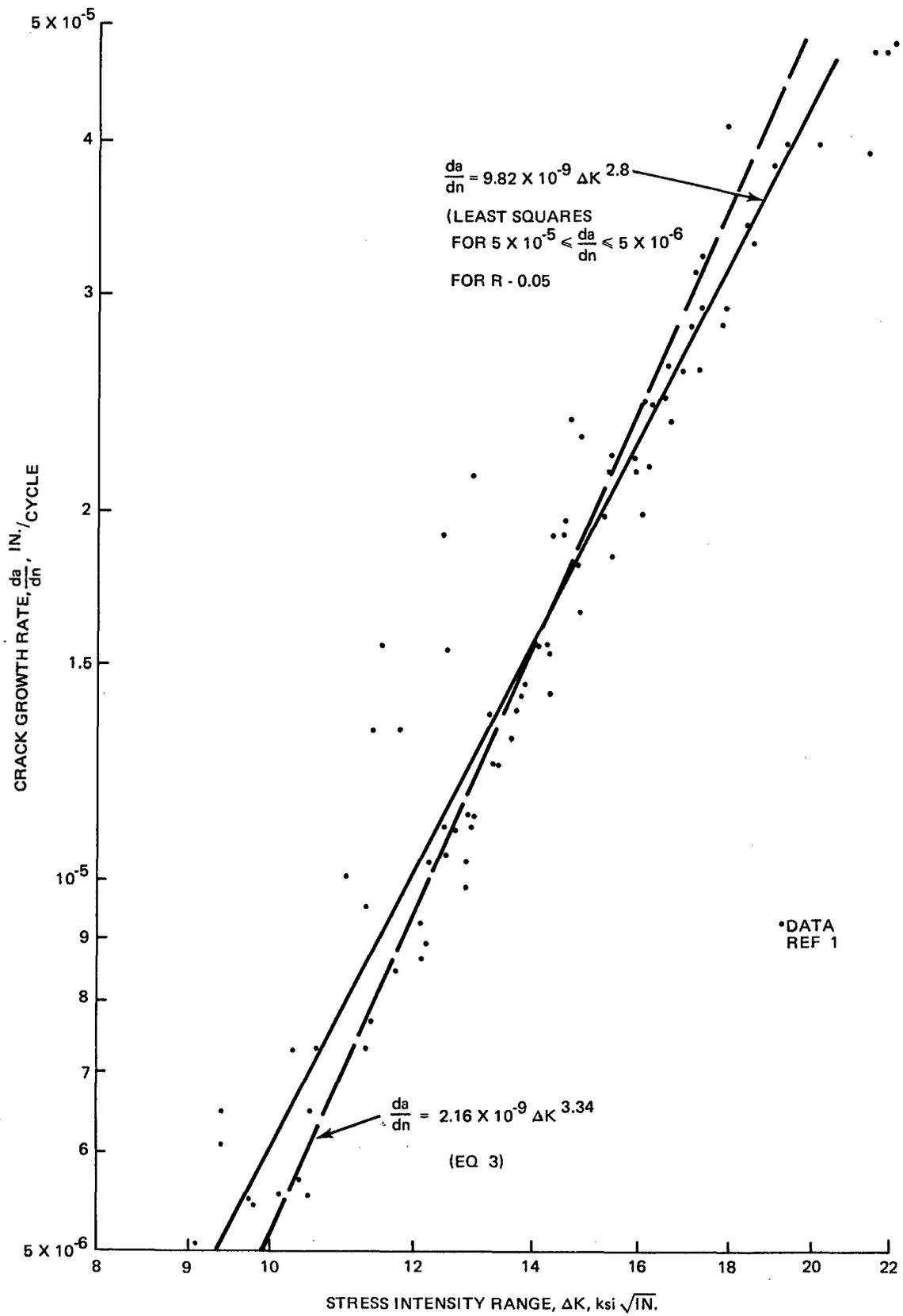
Figure 6 Crack Growth Rate vs Stress Intensity Range, 2219-T851 Aluminum, Constant Amplitude, R = 0.05
