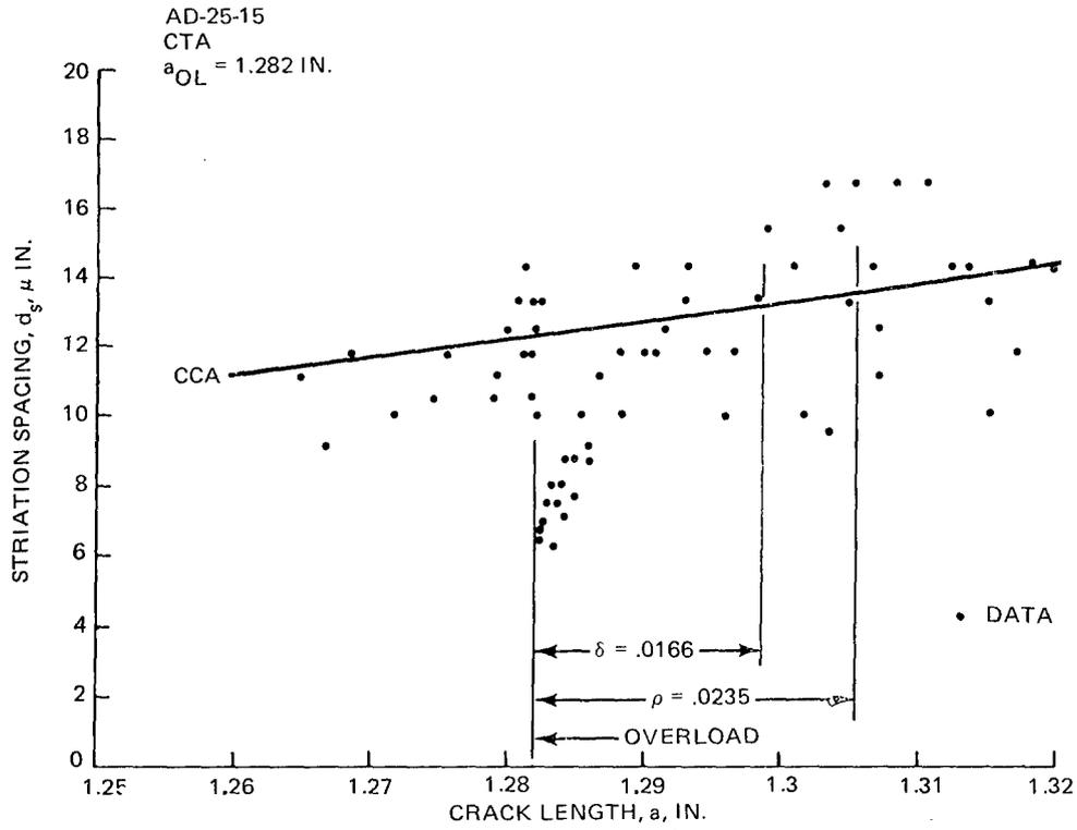
Figure 21 Affected Crack Length, Centerline, O/L = 1.5, 2219-T851 Aluminum
