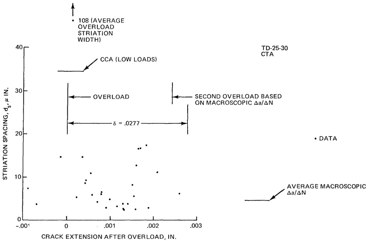
Figure 90 Single Periodic Overloads,  $a_{ref} = 1.5$  In.,  $O/L = 1.8$ ,  $N_{OL}/N = 1/500$ , Ti 6Al-4V Titanium
