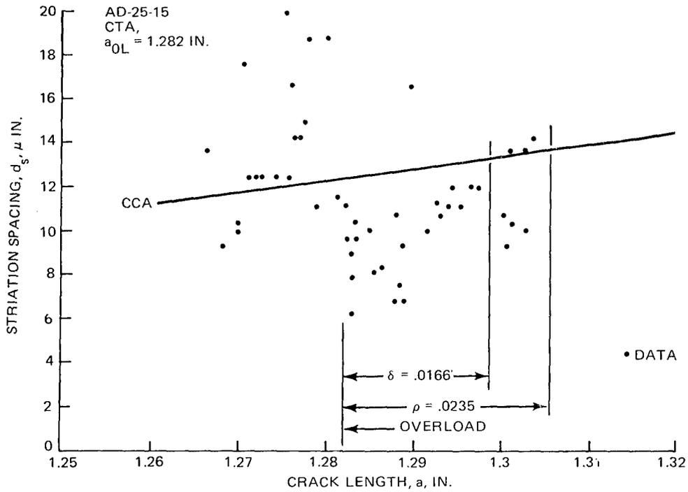
Figure 22 Affected Crack Length, Edge, O/L = 1.5, 2219-T851 Aluminum
