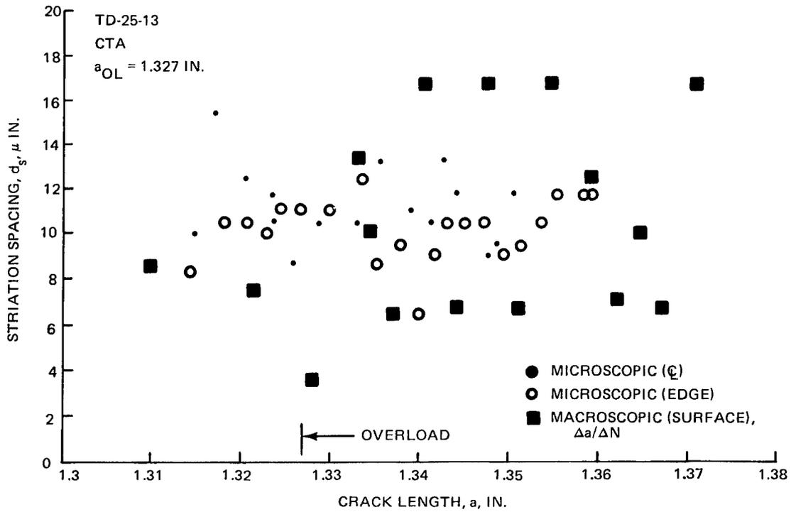
Figure 17 Striation Spacing and  $\Delta a/\Delta N$  vs Crack Length, Ti 6Al-4V Titanium, O/L = 1.25
