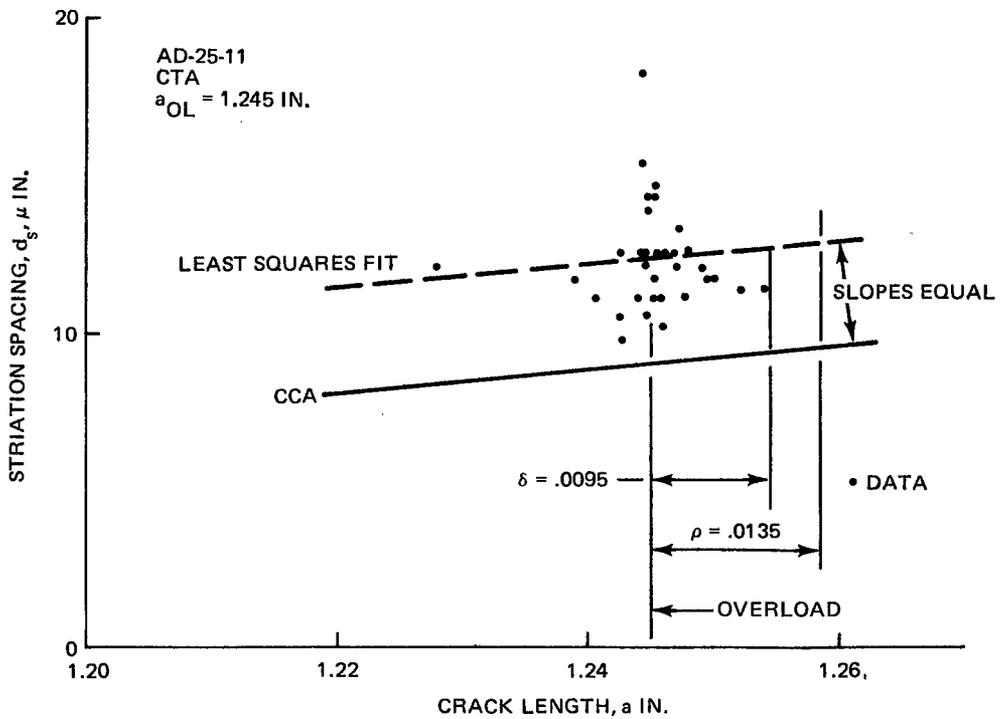
Figure 20 Affected Crack Length, Centerline, O/L = 1.25, 2219-T851 Aluminum
