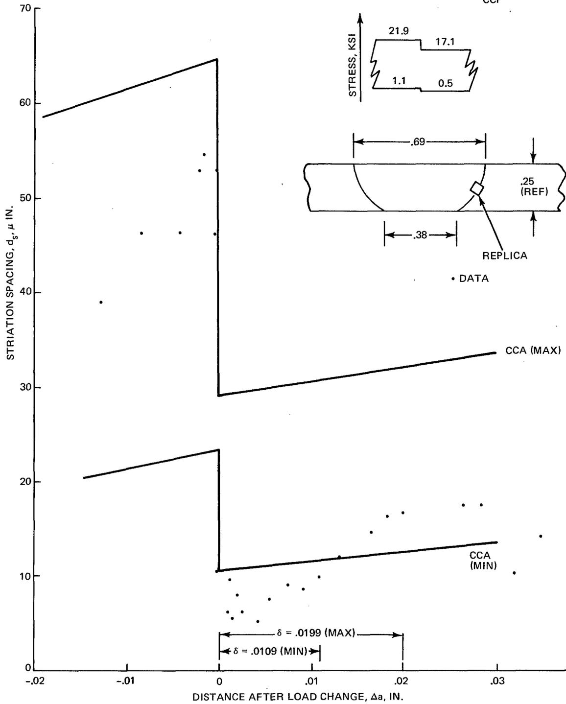
Figure 95 Transition Crack, High-Low Load,  $a_{ref} = 0.345$  In., 2219-T851 Aluminum
