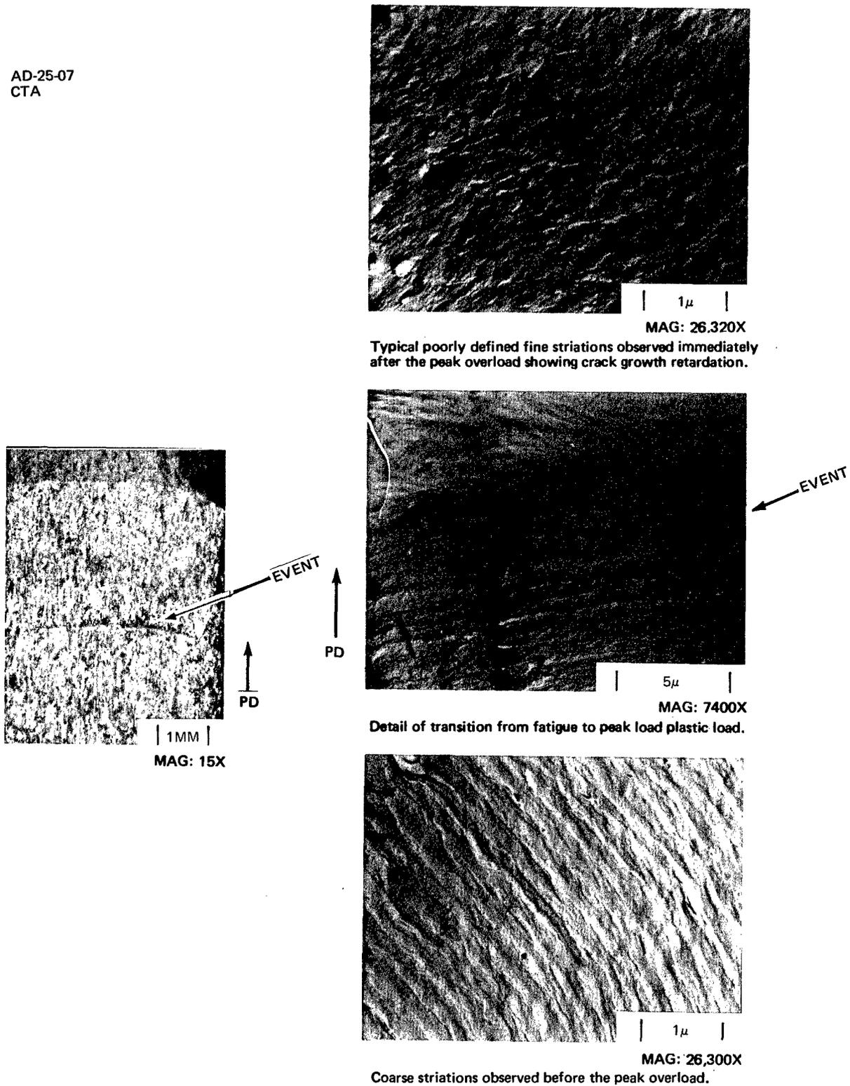
Figure A-2 Single Overload,  $a_{OL} = 1.375$  In., Centerline, O/L = 1.8, 2219-T851 Aluminum
