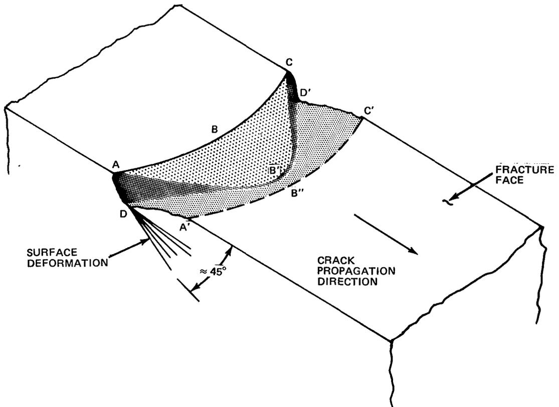
c. Schematic of Fracture Face in Vicinity of Overload Application
