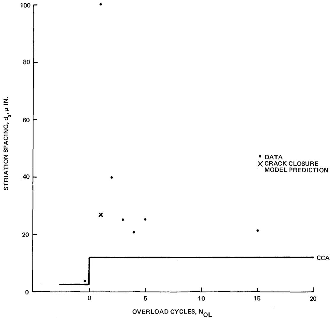
Figure 71 Acceleration,  $a_{OL} = 0.692$  In., O/L = 1.8, Ti 6Al-4V Titanium
