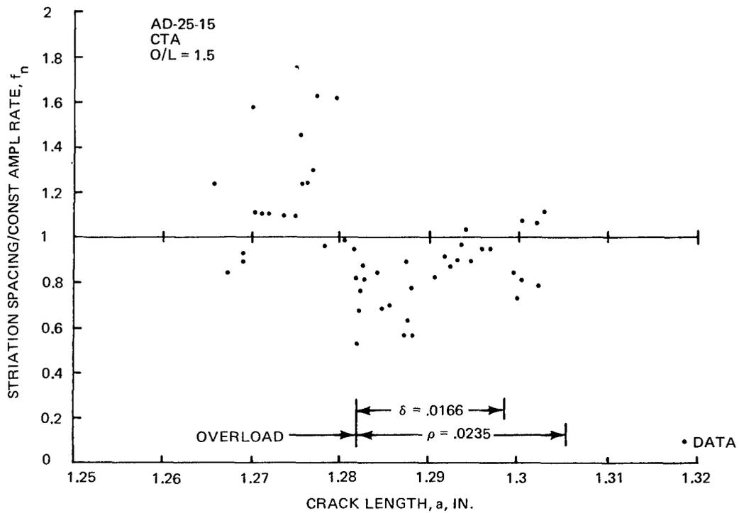
Figure 33 Typical Plot of  $f_n$  vs Crack Length
