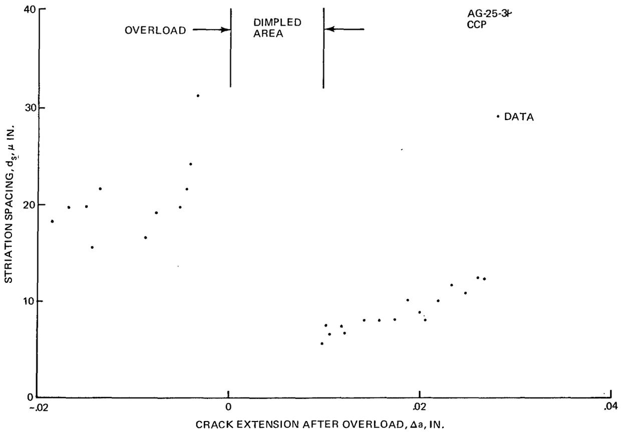
Figure 62 Striation Spacing vs Distance After Overload,  $a_{OL} = 1.263$  In., Centerline, O/L = 1.8, 2219-T851 Aluminum
