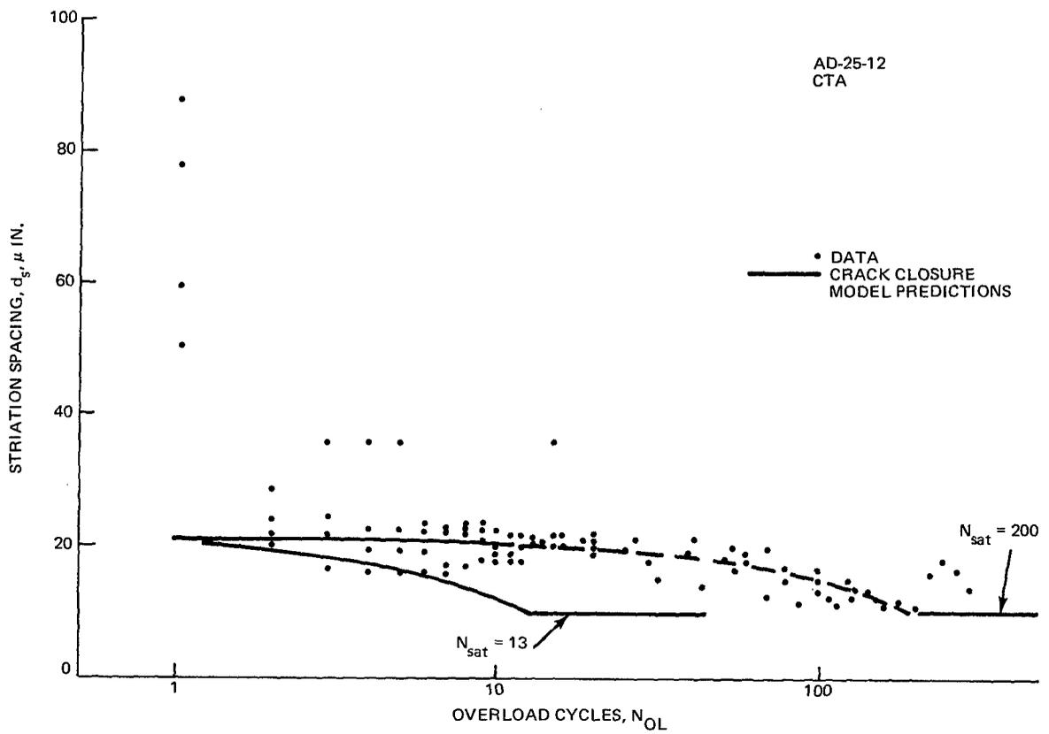
Figure 75 Crack Closure Model Predictions for 2219-T851 Aluminum
