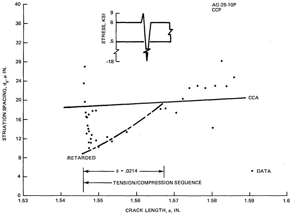
Figure 81 Tension/Compression,  $O/L = 1.5$ ,  $R_C = -3$ ,  $a_{ref} = 1.546$  In., 2219-T851 Aluminum
