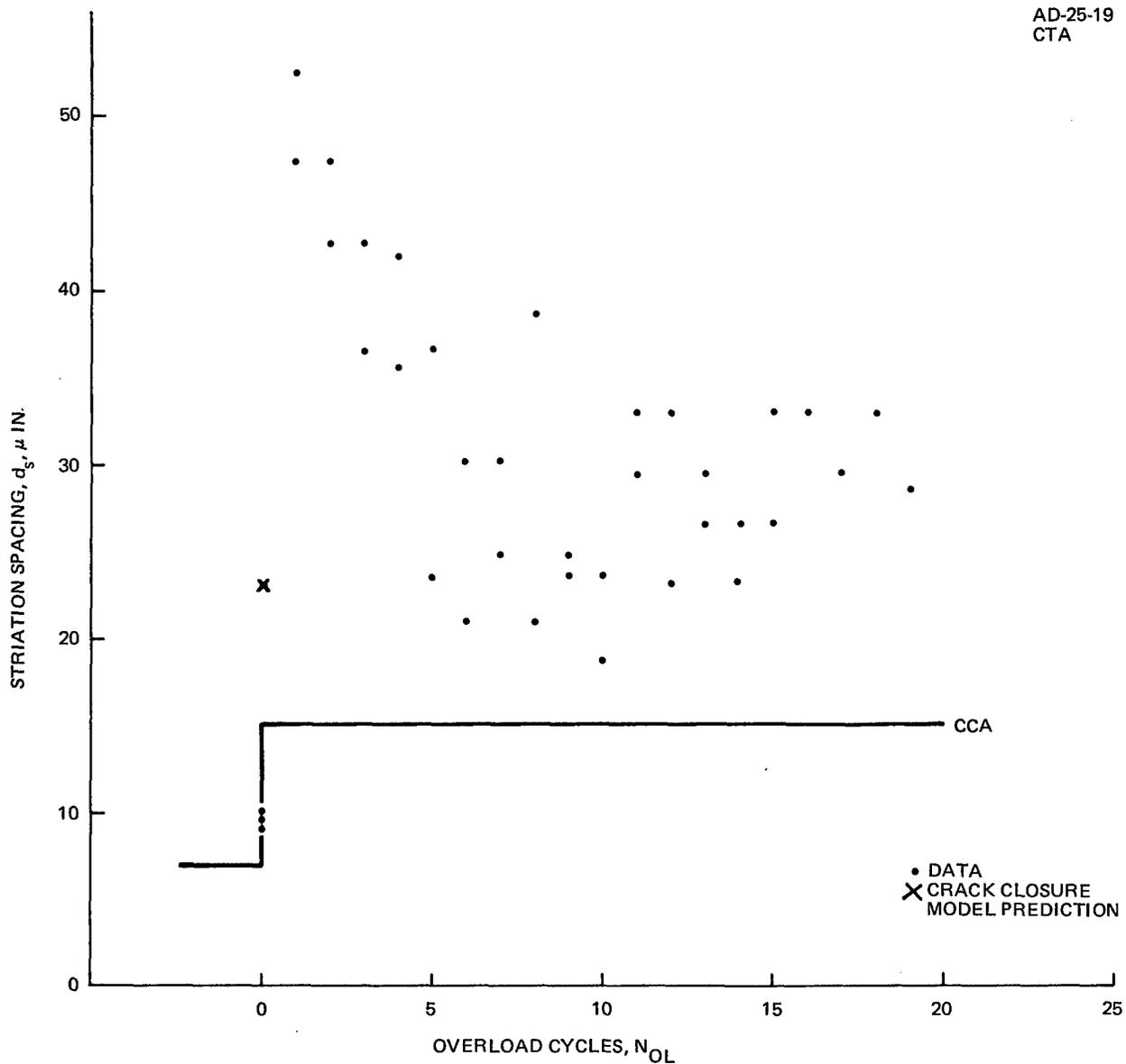
Figure 69 Acceleration,  $a_{OL} = 1.396$  In.,  $O/L = 1.25$ , 2219-T851 Aluminum
