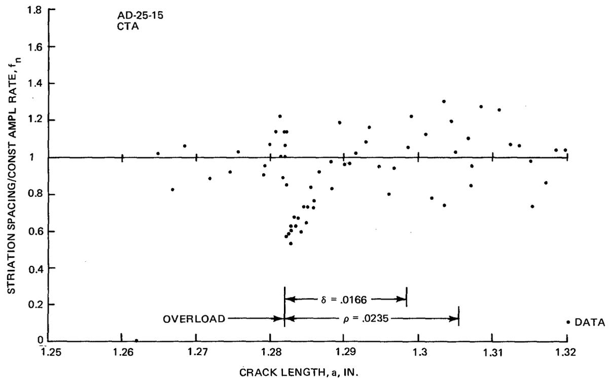
Figure 36 Delayed Retardation,  $a_{OL} = 1.282$  In., Centerline, O/L = 1.5, 2219-T851 Aluminum
