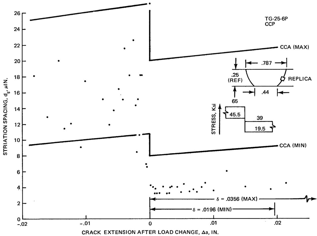
Figure 97 Transition Crack, High-Low Load,  $a_{ref} = .394$  In., Ti 6Al-4V Titanium
