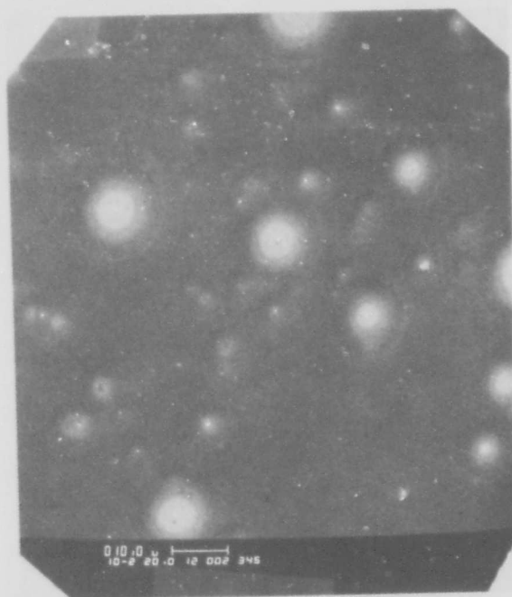
Figure 20 SEM pictures of vapor deposited Al after exposure to 96°C water (left) and 50°C water (right) for 1/2 hr.
