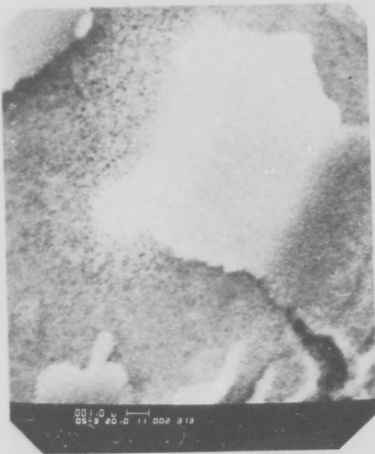
Figure 24 SEM pictures of vapor deposited Al after exposure to 96°C water (left) for 46.7 hrs and 50°C water (right) for 70 hrs.
