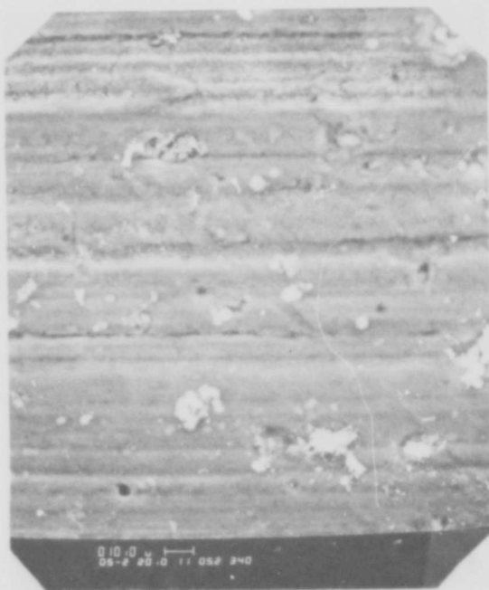
Figure 31 SEM pictures for vapor degreased Al 2024-T3 as received (top) after 50°C water exposure for 21 hrs (bottom).
