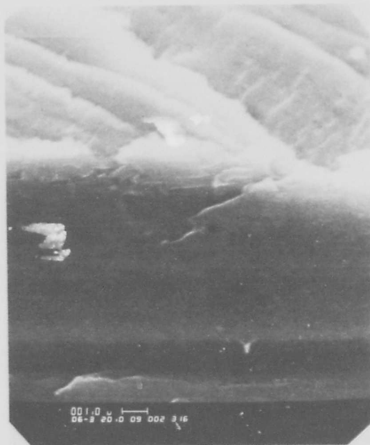
Figure 39 SEM pictures of phosphoric-anodized Al 2024-T3 after electropolished.
