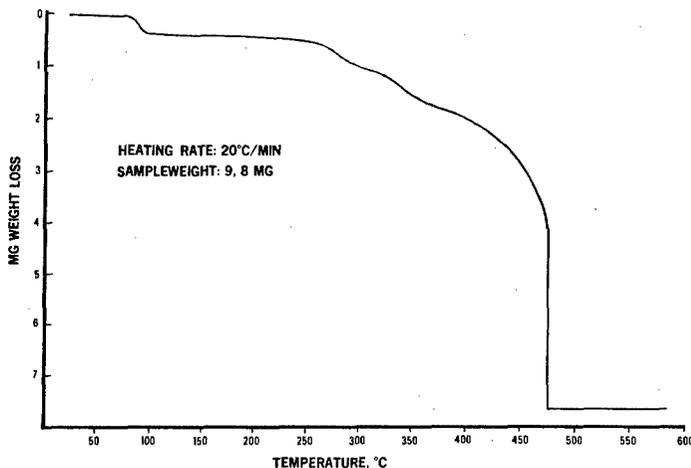
Figure 12. TGA trace for fluomine in air.
