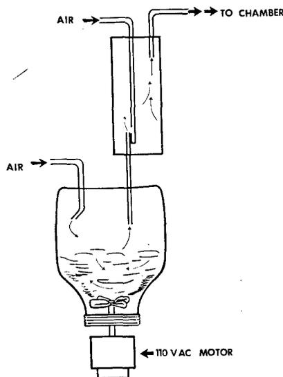
Figure 1. Alumina dust generator.
