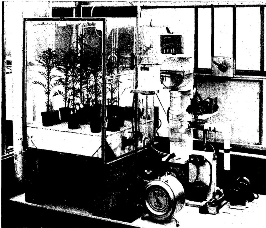
Figure 1. Plant exposure chamber for gas/aerosol studies.
