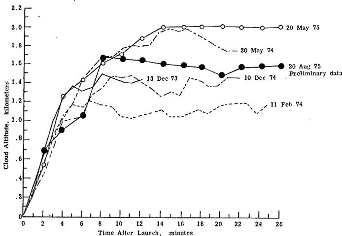
Figure 6. Measured Titan III cloud rise to stabilization in the atmosphere - KSC launches.
