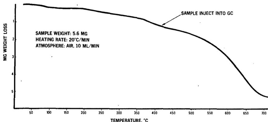
Figure 9. TGA trace of Aramid fabric with finish.
