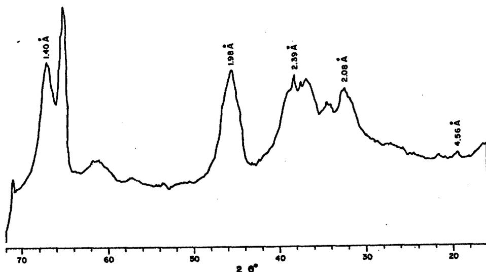
Figure 3. X-ray powder diffractogram of aluminum oxide (gamma form).
