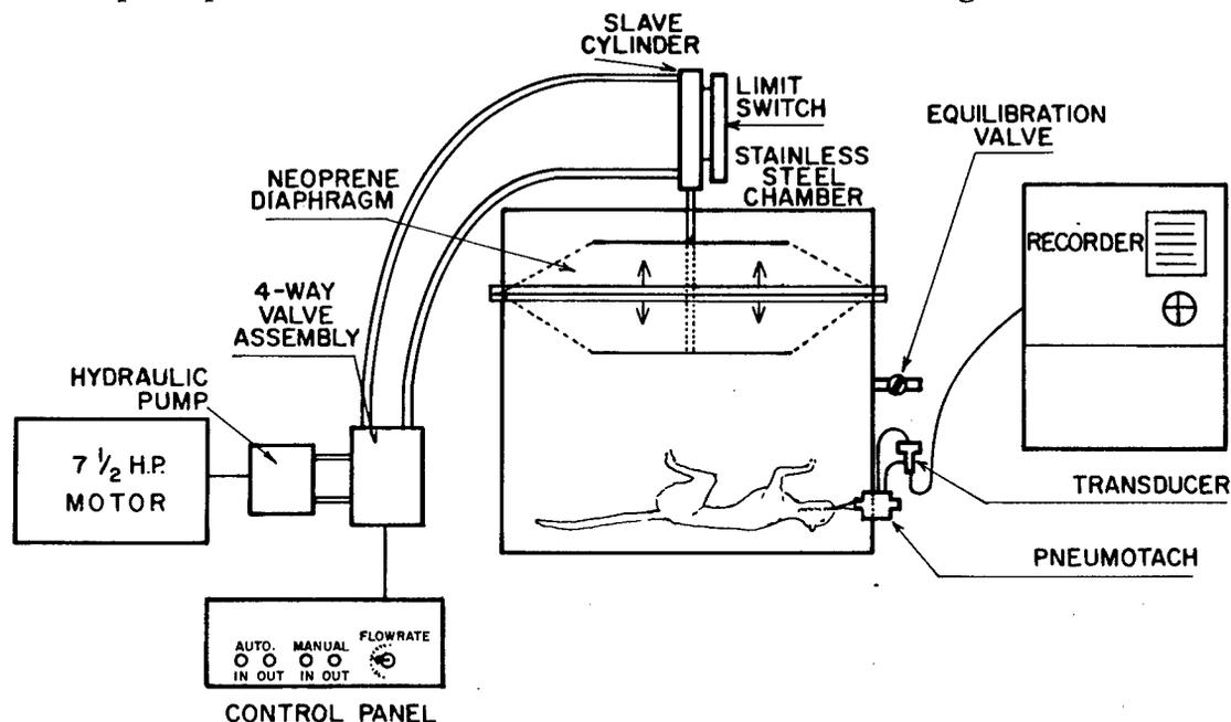
Figure 1. Diagram of Plethysmograph-respirator.
