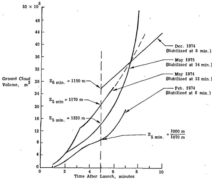
Figure 7. Measured Titan III ground cloud growth.
