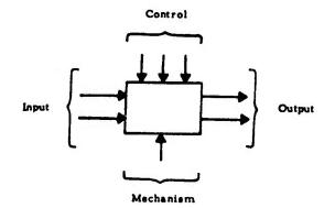
The input data (on the left) are transformed into output data (on the right). Controls (on the top) govern the way the transformation is done. Mechanisms (on the bottom) indicate the means by which the function is performed. A "mechanism" might be a person, a committee, a machine, or a process.
