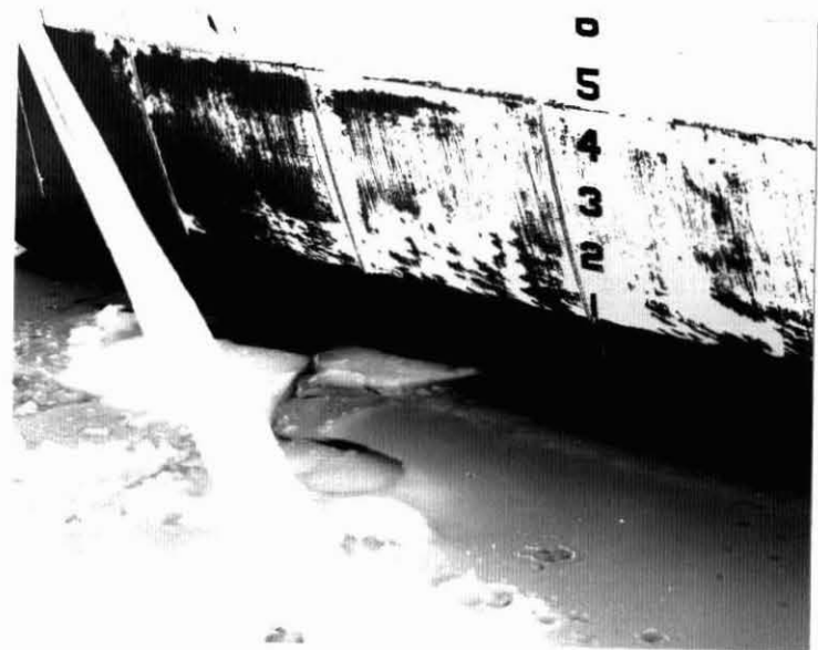
Figure II-15 Photographs of the Ice Line of the Hull of the Cutter Mackinaw after Icebreaking Service
