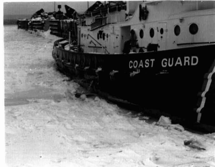
134 Figure II-20 Water Line Area of the Hull of the USCG Cutter Raritan after Icebreaking Service. Photographs taken during March 75 before the end of the icebreaking season.
