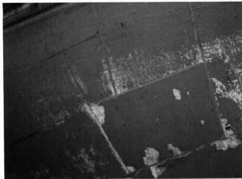
169 Figure II-27 Condition of the Hull of the USCG Cutter West Wind after Icebreaking Service. Areas shown are from the bow to midship.
