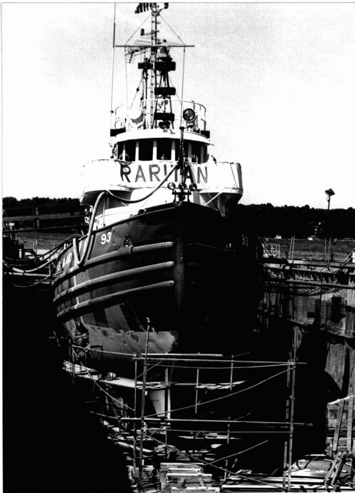
Figure II-23 Condition of the Hull of the Cutter Raritan after Grit Blasting the Damaged Areas for Repair
