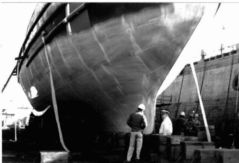
Figure II-6 Appearance of the Hull of the USCG Cutter Sauk after Grit Blasting and Priming
