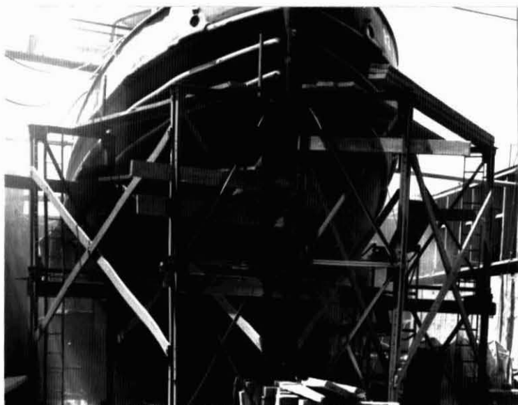
Figure II-19 Photographs of the Hull of the Cutter Raritan after Application of a Nonsolvent Polyurethane
