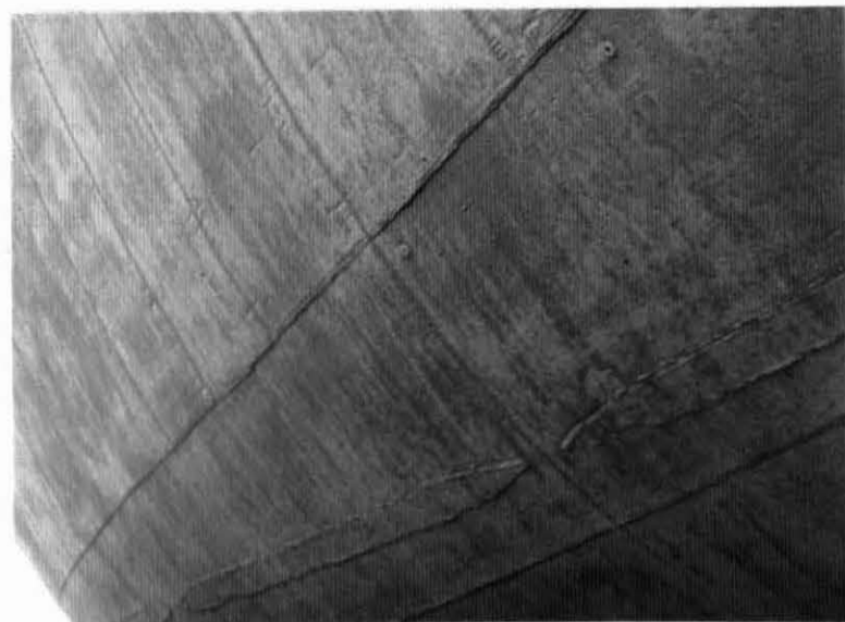
Figure II-28 Condition of the Hull of the USCG Cutter West Wind after Icebreaking Service. Areas shown are the stern and underside portion of the hull.
