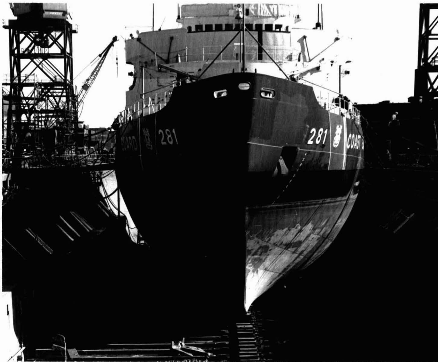
168 Figure II-26 Condition of the Bow of the USCGC Cutter West Wind after Icebreaking Service. The white areas are the glass flake polyester coating. The grey areas are the steel surface where the coating was removed.
