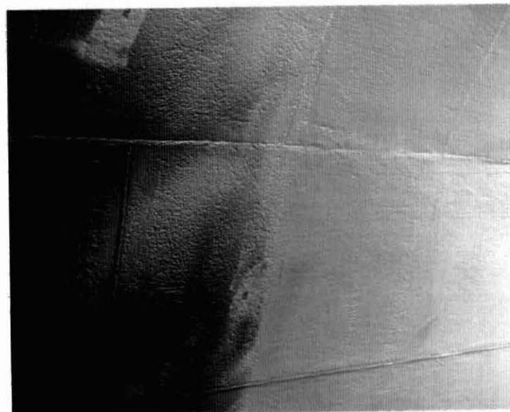
Figure II-17 Typical Hull Appearance of the USCG Cutter Mackinaw after Coating with Nonsolvented Urethane. Note the base metal showing the pits in the metal before application.
