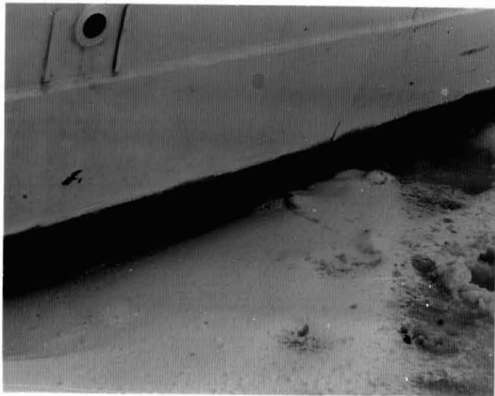
Figure II-15 Photographs of the Ice Line of the Hull of the Cutter Mackinaw after Icebreaking Service
