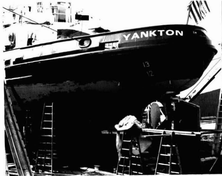
Figure II-1a Condition of the Hull of the US Cutter Yankton before Recoating
