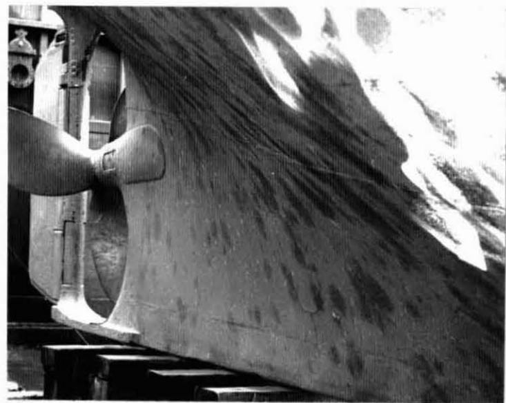
Figure II-21 Condition of Hull of the USCG Cutter Raritan before Cleaning
