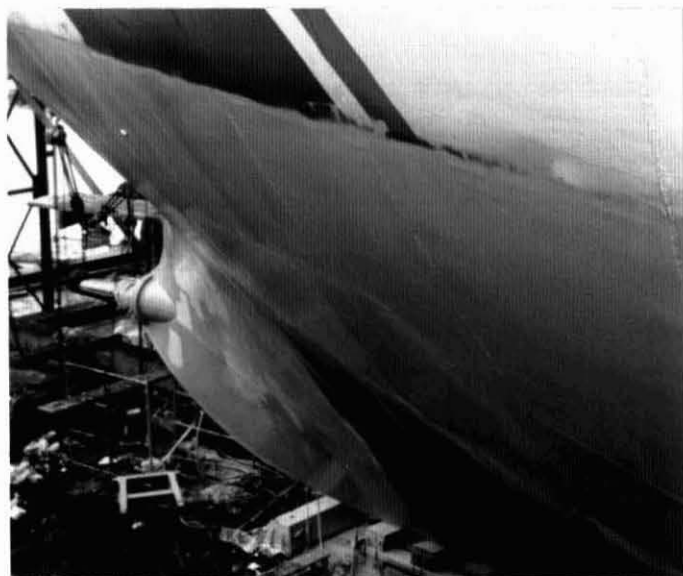
Figure II-18 Overall View of the Hull of the USCG Cutter Mackinaw after Applying the Nonsolvented Urethane
