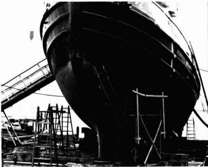
Figure II-1b Condition of the Hull of the US Cutter Yankton after Reactivation of the Primer but before Polyurethane Coating
