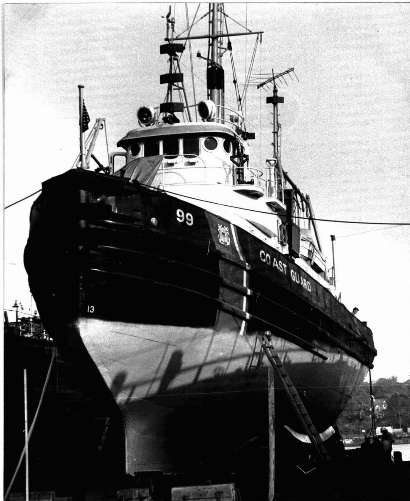
Figure II-5 Hull Appearance of the USCG Cutter Sauk after Grit Blasting
