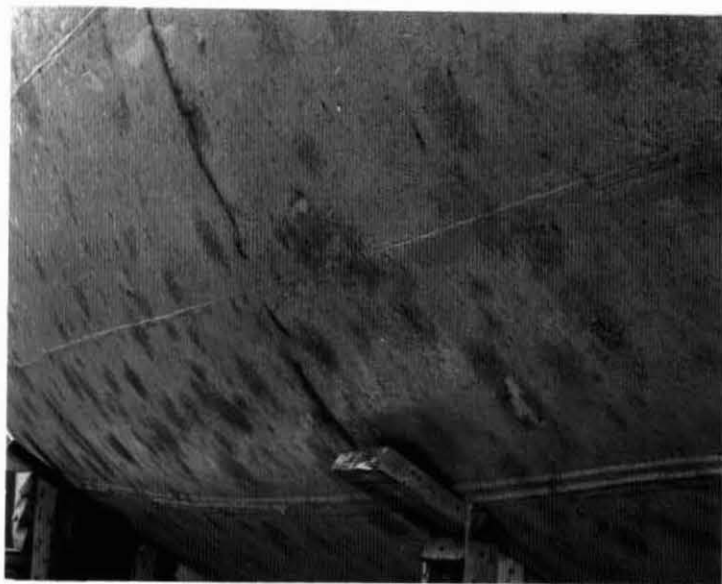
Figure II-21 Condition of Hull of the USCG Cutter Raritan before Cleaning
