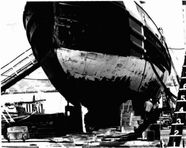
Figure II-1a Condition of the Hull of the US Cutter Yankton before Recoating
