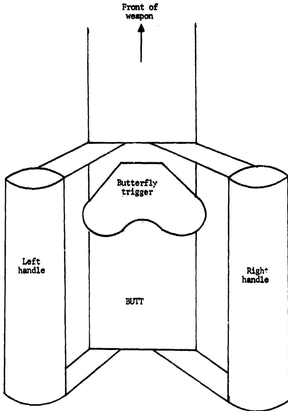
Figure 14. Trigger location
