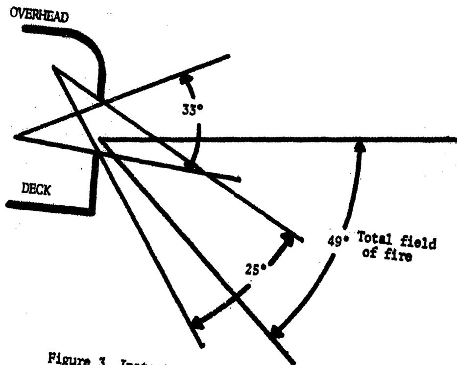
Figure 3. Instantaneous field of view: Vertical
