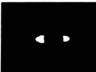
Fig. 4. Small angle X-ray scattering photographs for AS, HTS, HMS and Morganite I carbon fibers.
