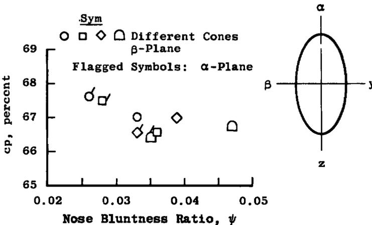
Figure 8. Variation of center of pressure with bluntness.
