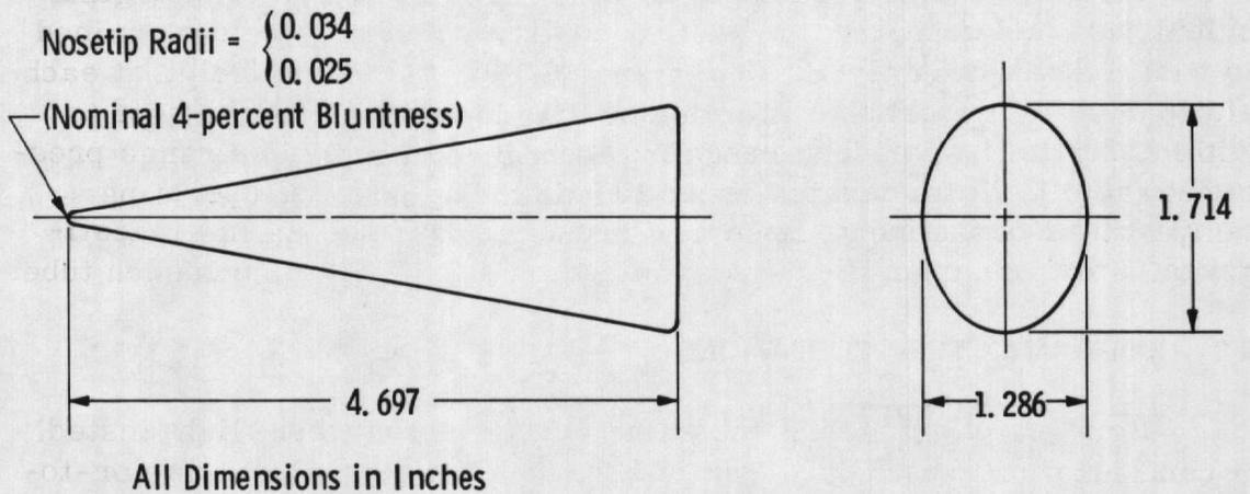
Figure 3. Elliptic cone.
