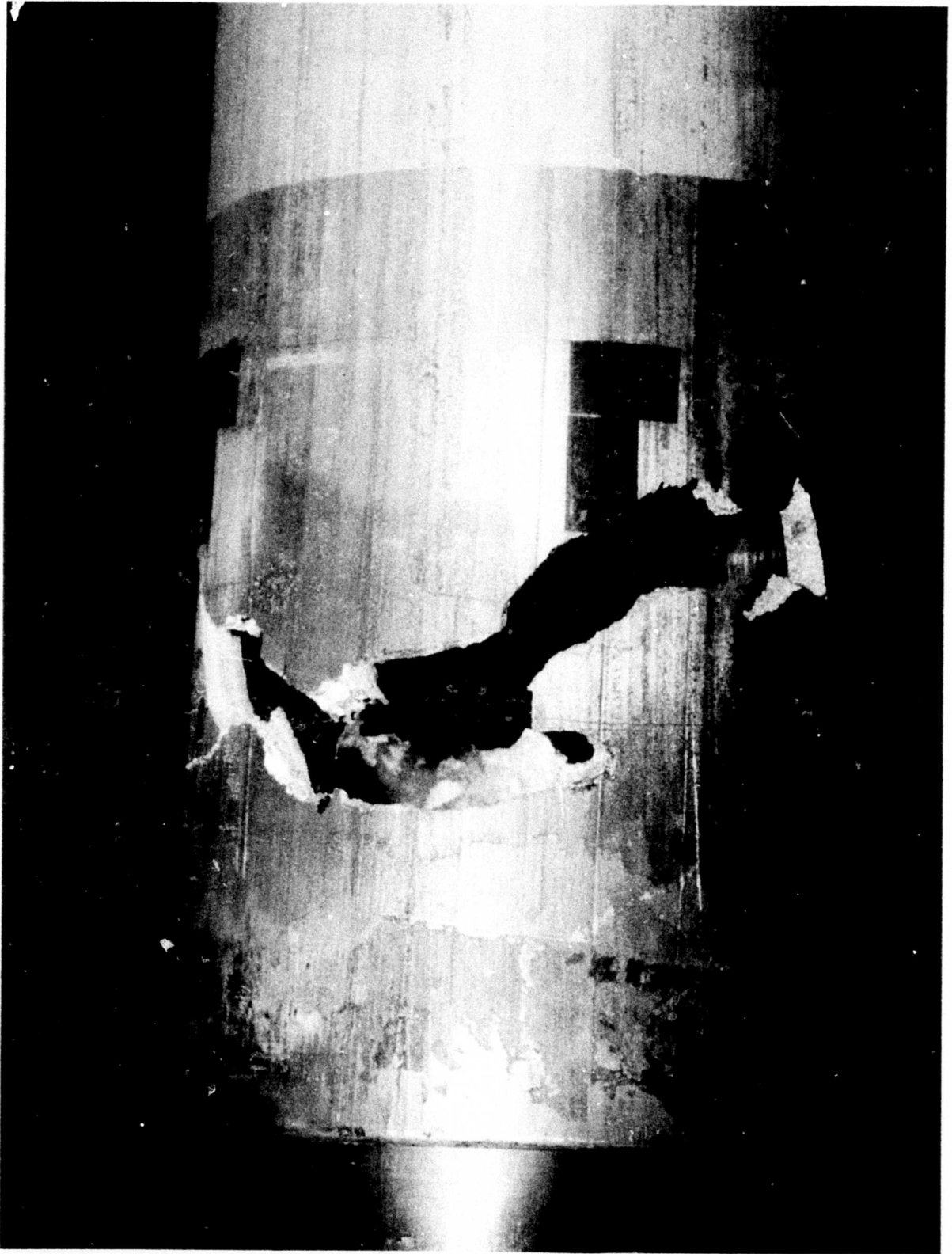
FIGURE 110. BALLISTIC SPECIMEN NUMBER 2 FATIGUE TEST FRACTURE, 180° TO 300° OF REVOLUTION
