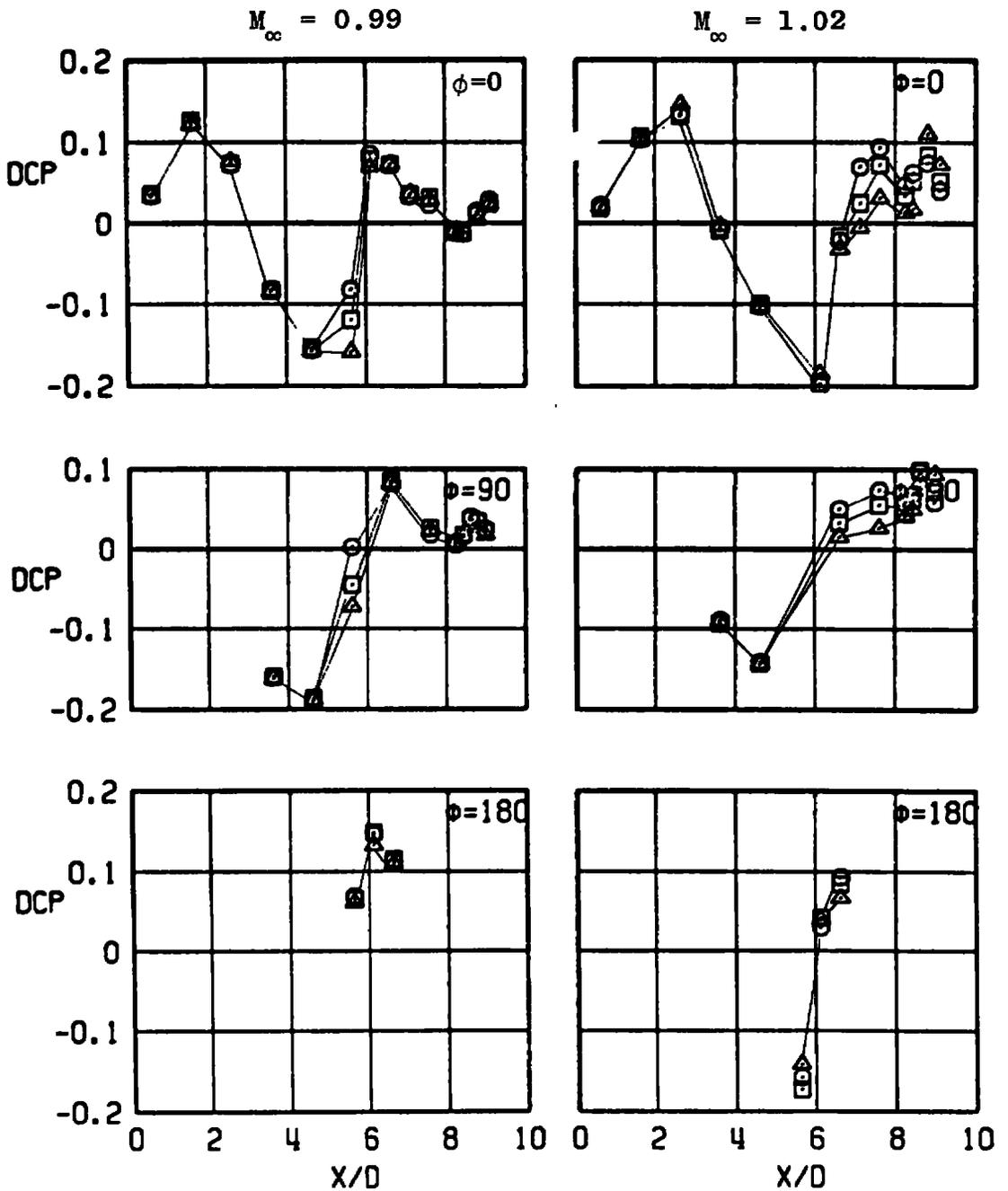
Figure 43. Effect of local wall porosity on body pressure interference coefficient.
