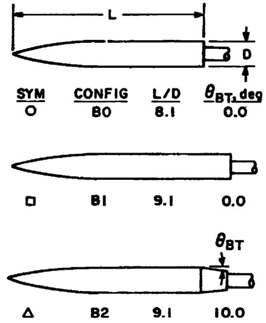
Figure 12. Effect of boattail angle and body length on base pressure coefficient.
