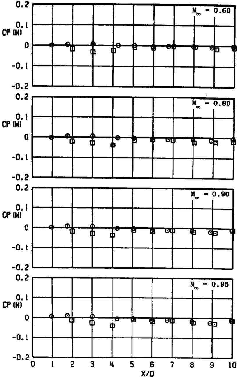
d. CP(W) versus X/D (30-deg swept strut, 10-deg boattail,  $\phi = 0$ )
