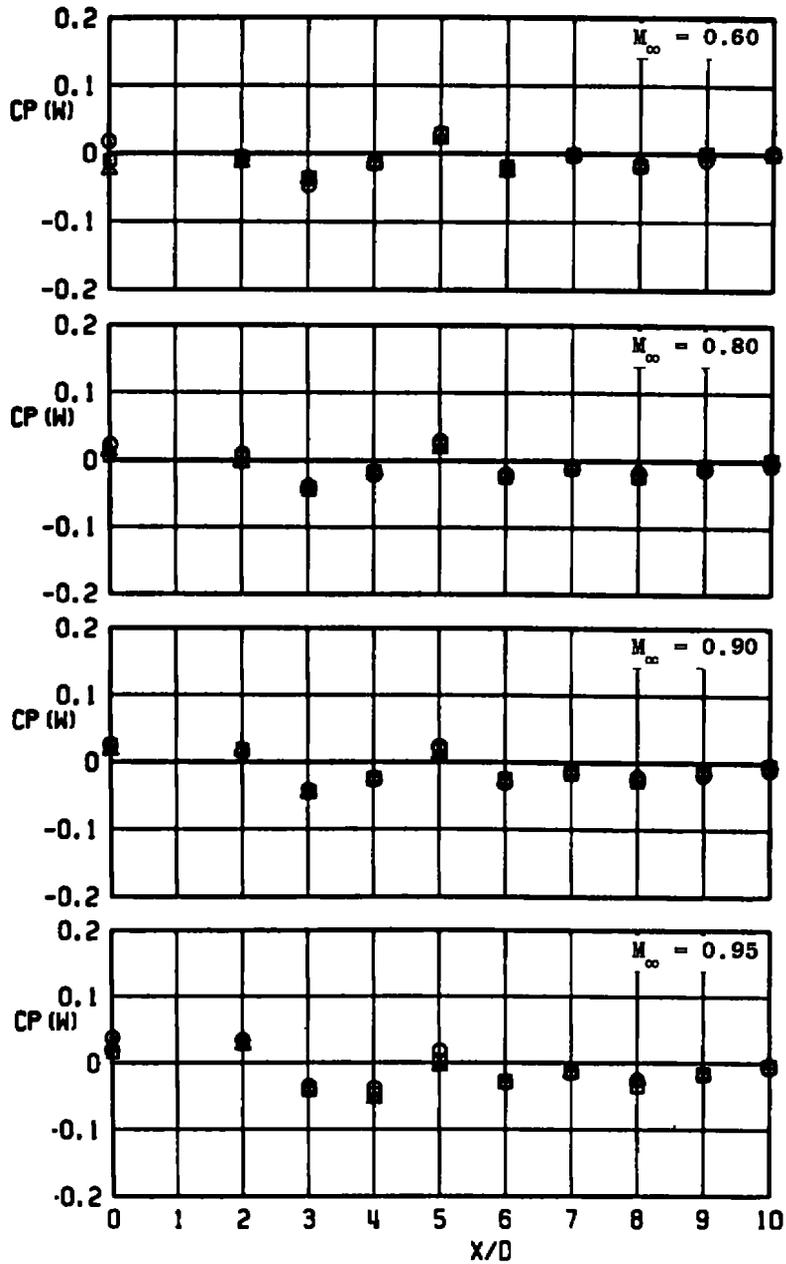
d.  $CP(W)$  versus  $X/D$  (straight strut, 10-deg boattail,  $\phi = 90$  deg)
