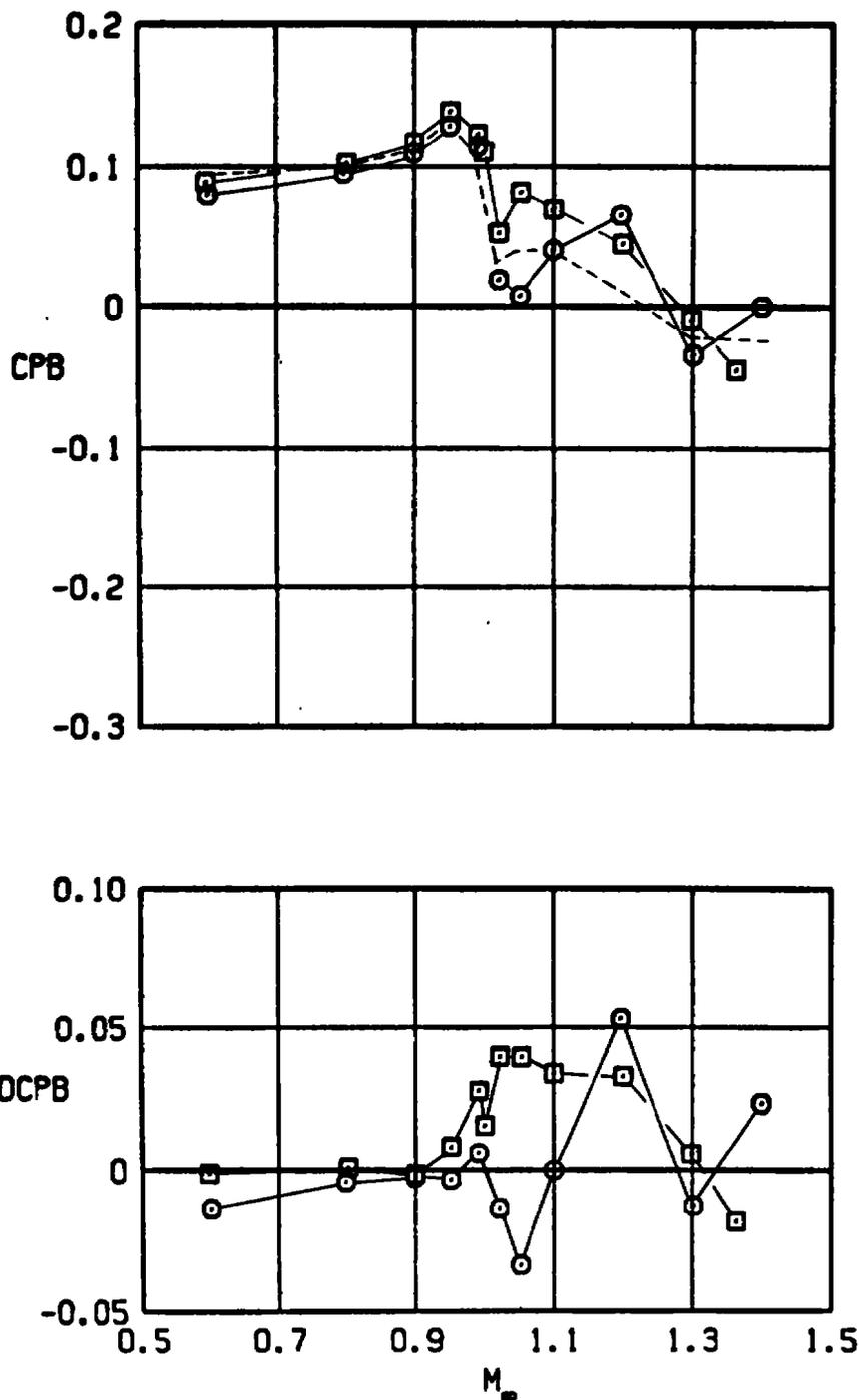
Figure 23. Effect of straight strut location on base pressure coefficient.
