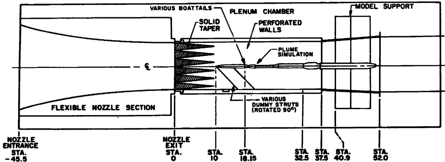
a. Schematic of model installation
