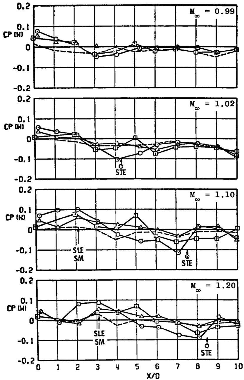
Figure 21. Effect of strut sweep angle on wall pressure coefficient.
