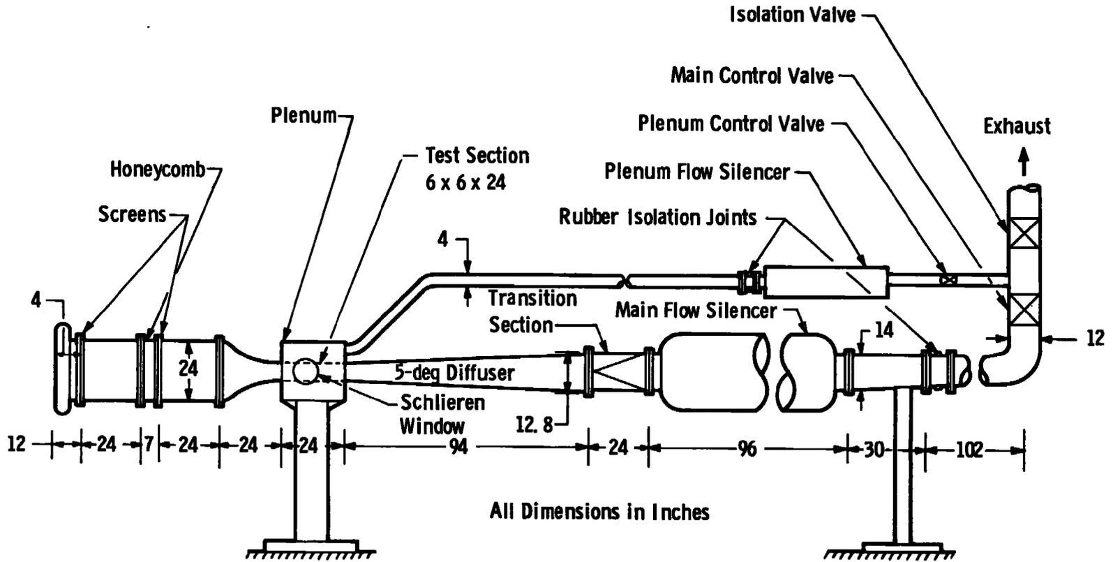
Figure 2. Model installation in PWT Acoustic Research Tunnel.
