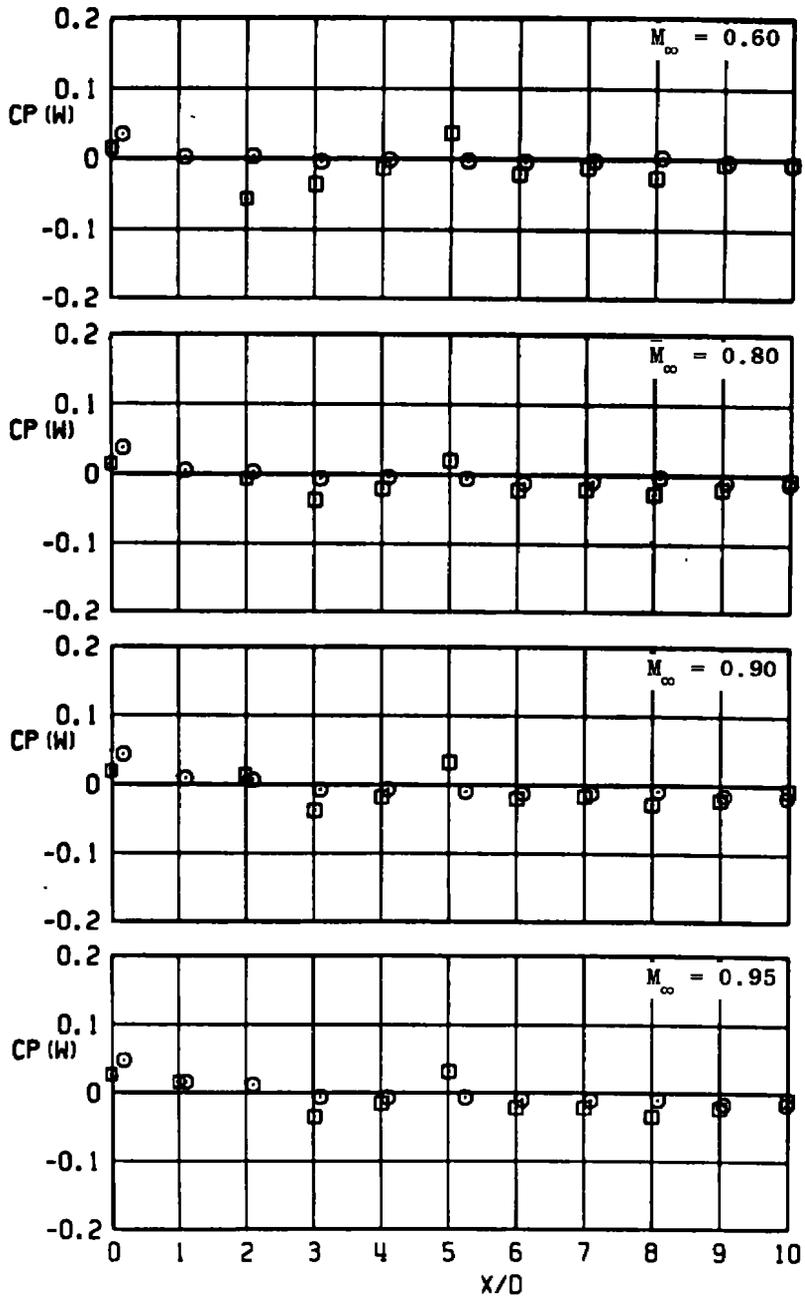
e. CP(W) versus X/D (30-deg swept strut, 10-deg boattail,  $\phi = 90$  deg)
