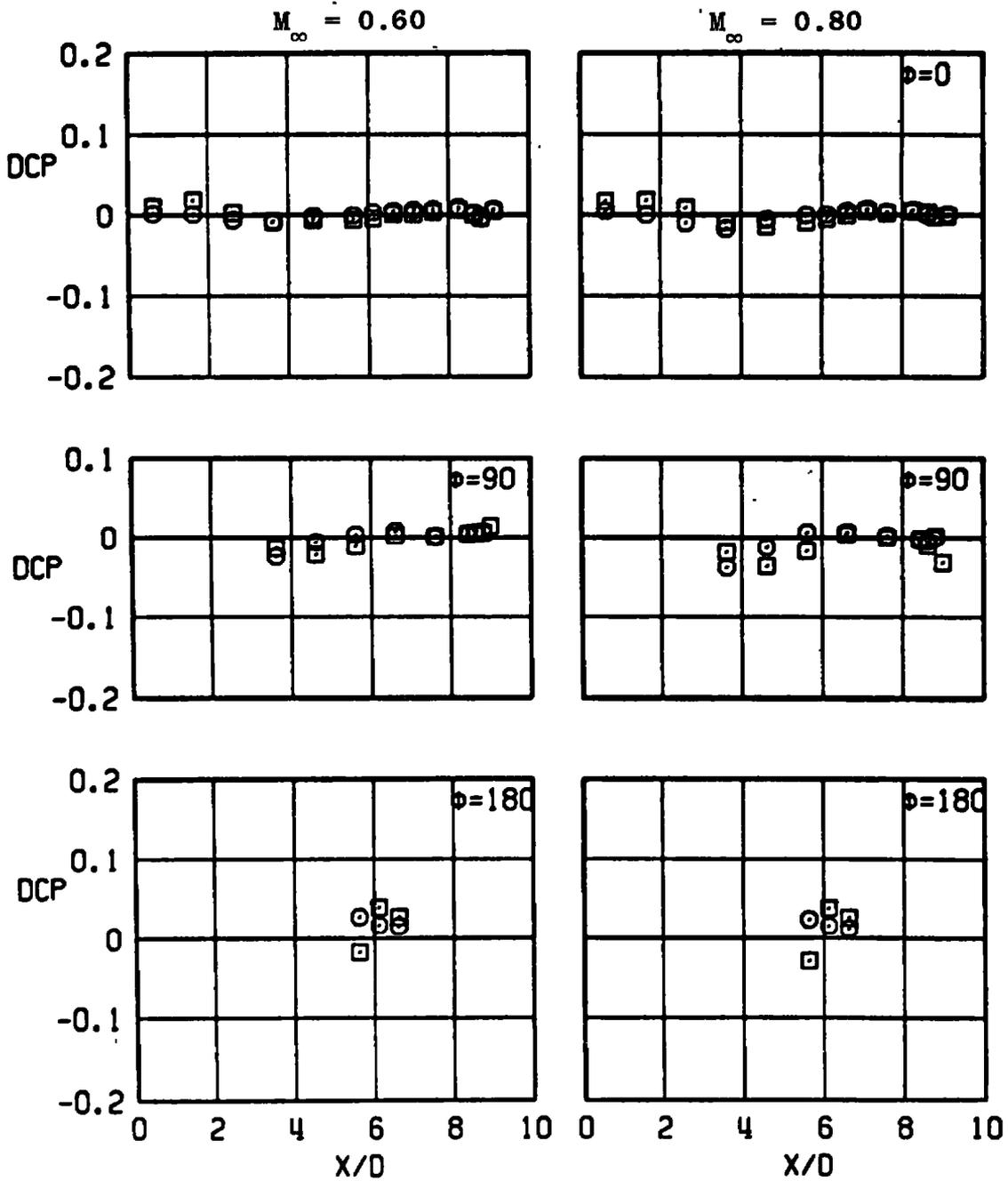
e. DCP versus X/D (30-deg swept strut, cylindrical afterbody)
