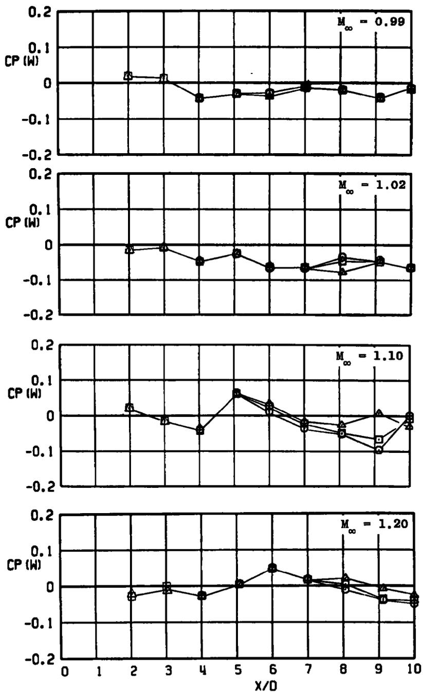
Figure 45. Effect of local wall porosity on wall pressure coefficient.
