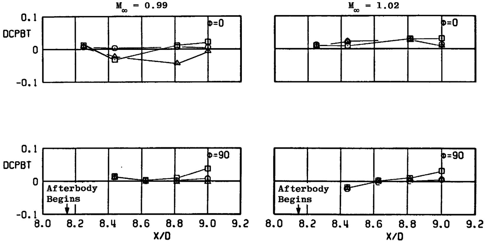
Figure 15. Effect of sting flare location on interference coefficient for cylindrical afterbody.
