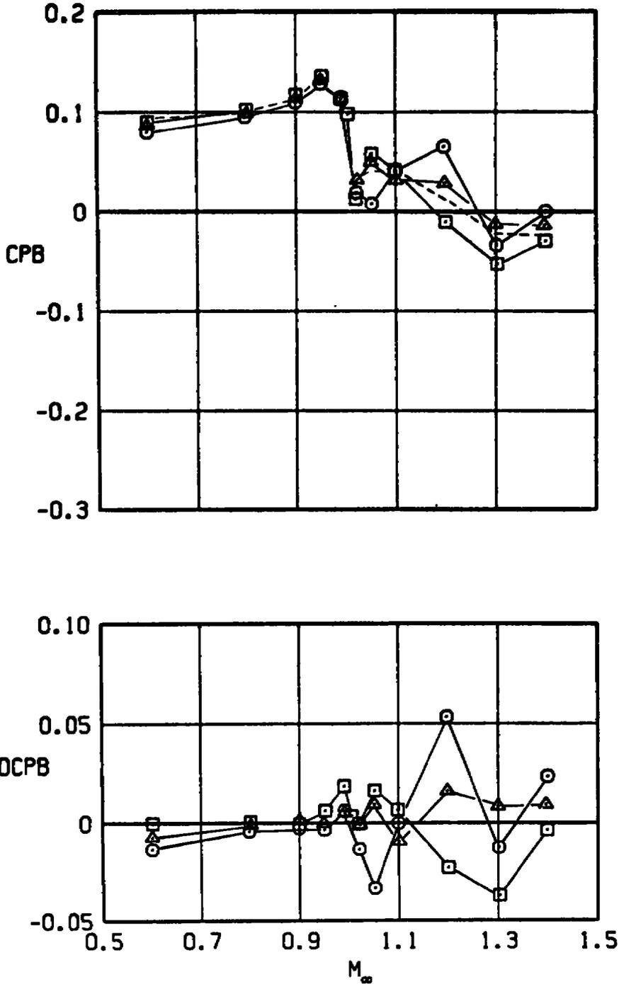
Figure 17. Effect of strut sweep angle on base pressure coefficient.
