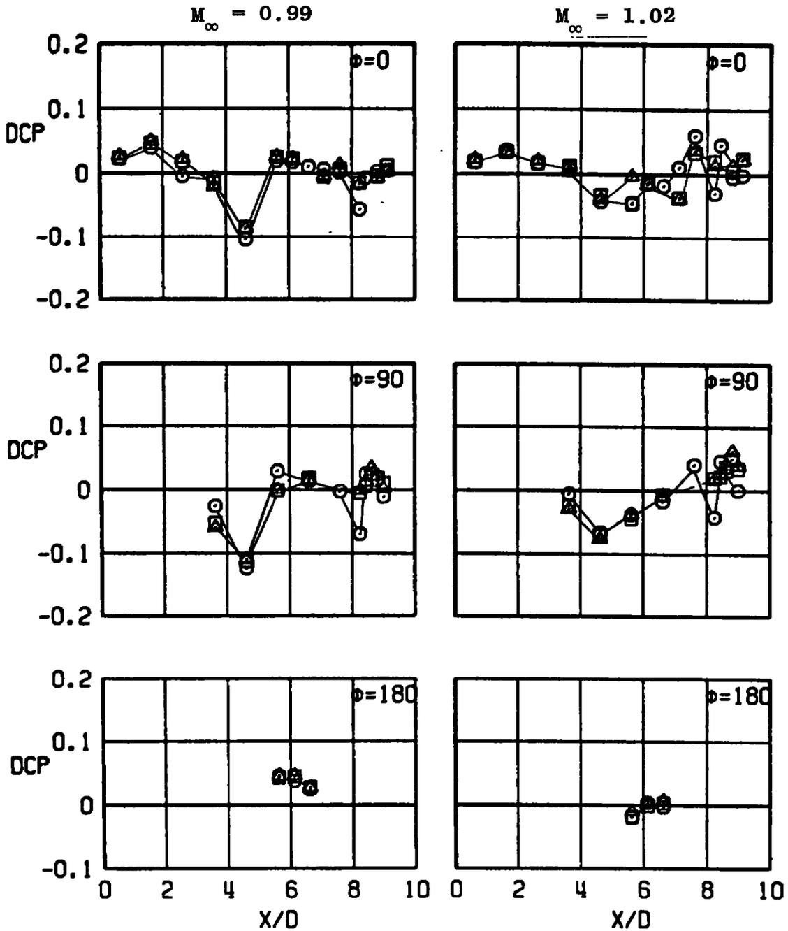
Figure 48. Effect of local wall porosity on body pressure interference coefficient for swept strut, S3L1.
