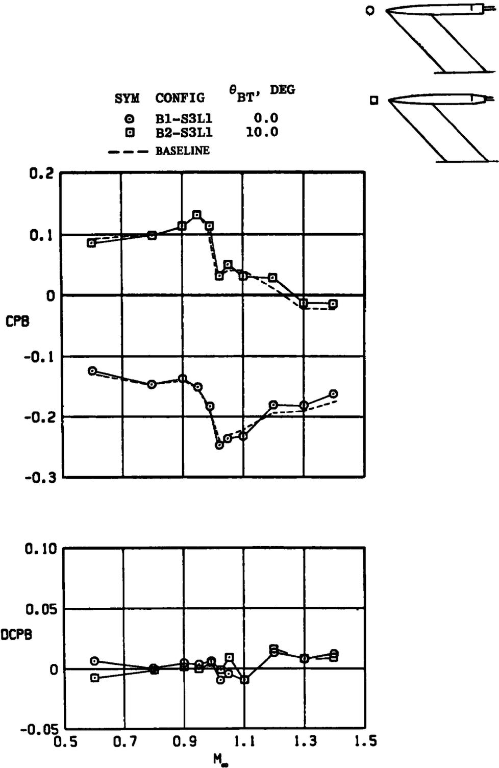
Figure 22. Effect of boattail angle on base pressure interference coefficient for straight and swept support struts.
