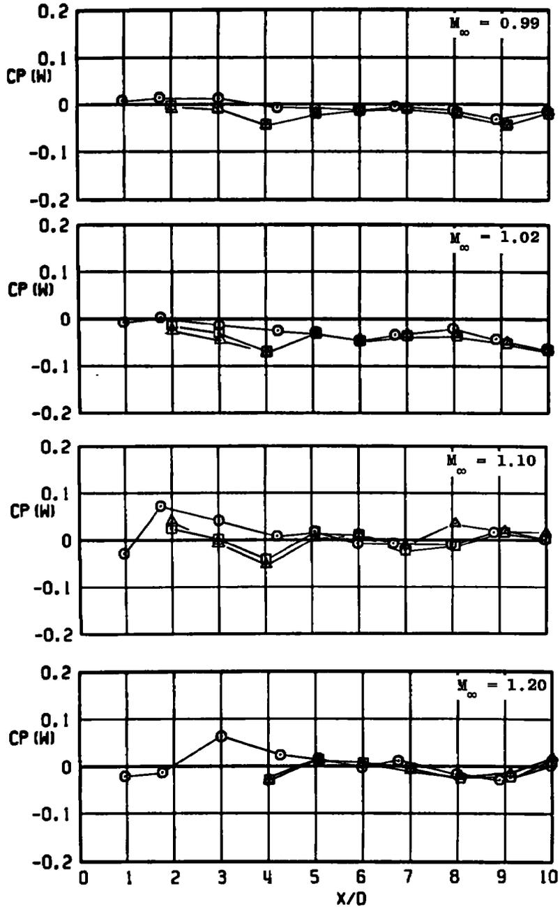
Figure 49. Effect of local wall porosity on wall pressure coefficient with swept strut, S3L1.
