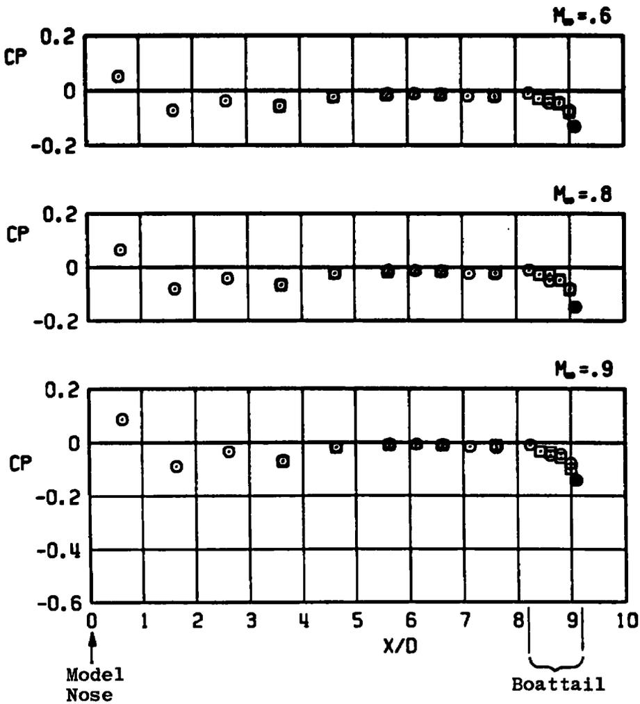
a. Model surface pressure coefficient distribution
