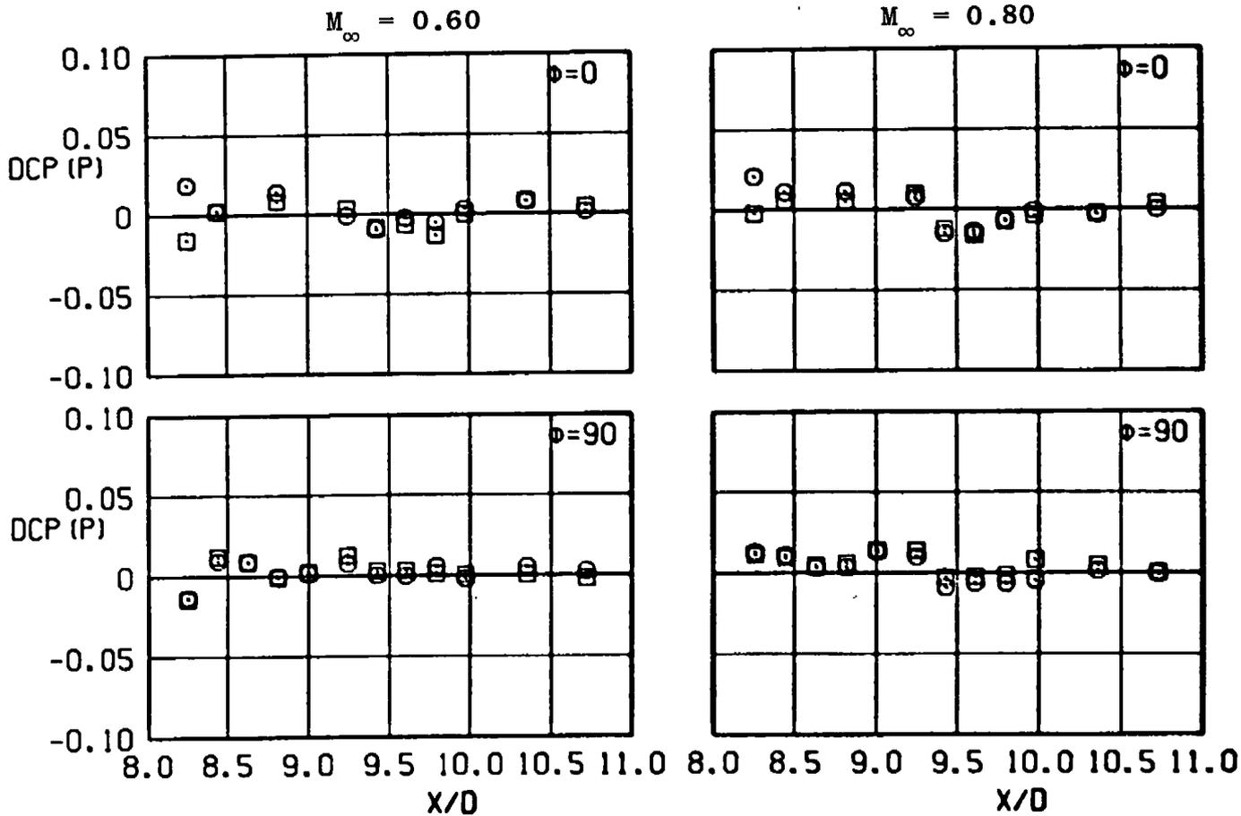
b. DCP(P) versus X/D (30-deg swept strut wity varying position)
