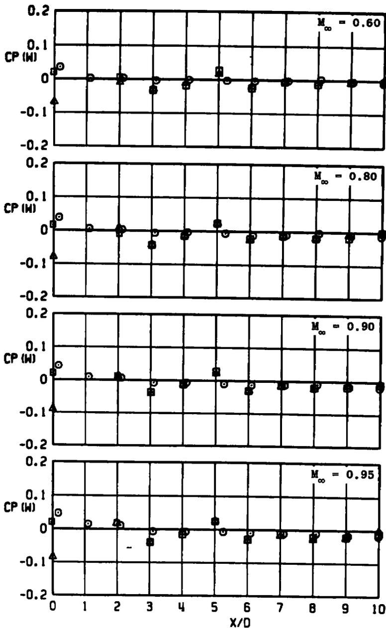
h. CP(W) versus X/D (30-deg swept strut, 10-deg boattail,  $\phi = 90$  deg)
