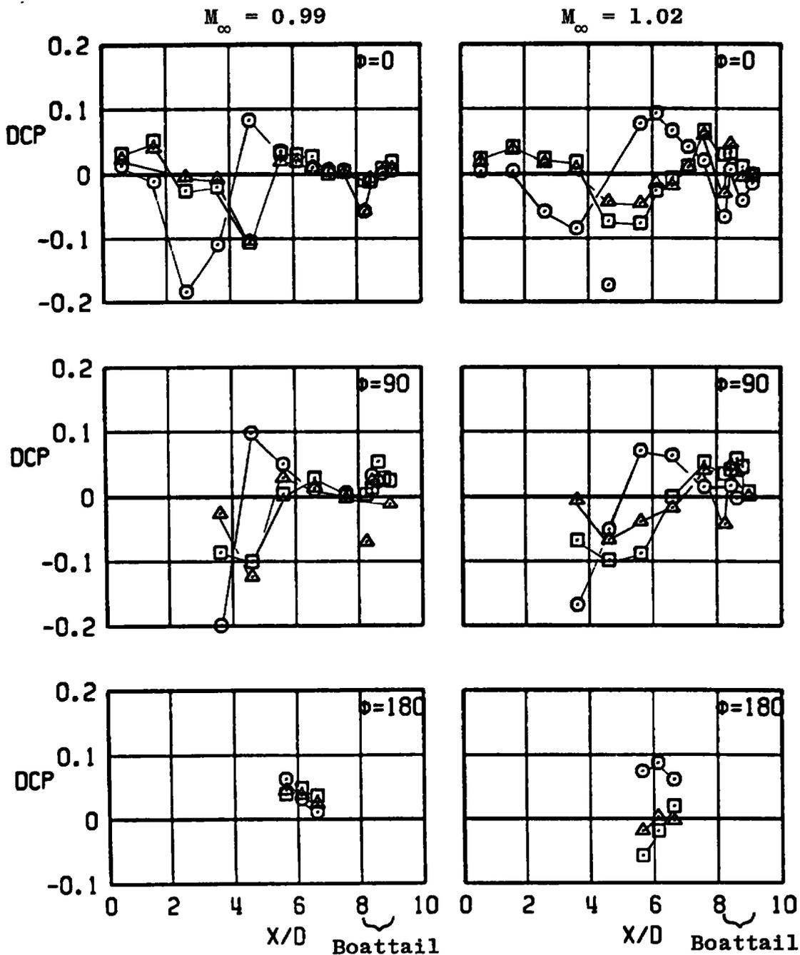
Figure 19. Effect of strut sweep angle on body interference coefficient.
