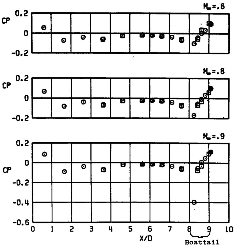
a. Model surface pressure coefficient distribution
