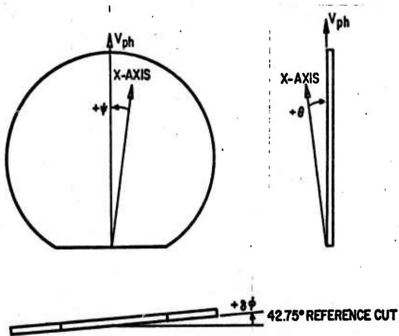
FIGURE 2.4.7(b) DEFINITION OF ANGLES FOR VELOCITY CALCULATIONS ON ST QUARTZ
