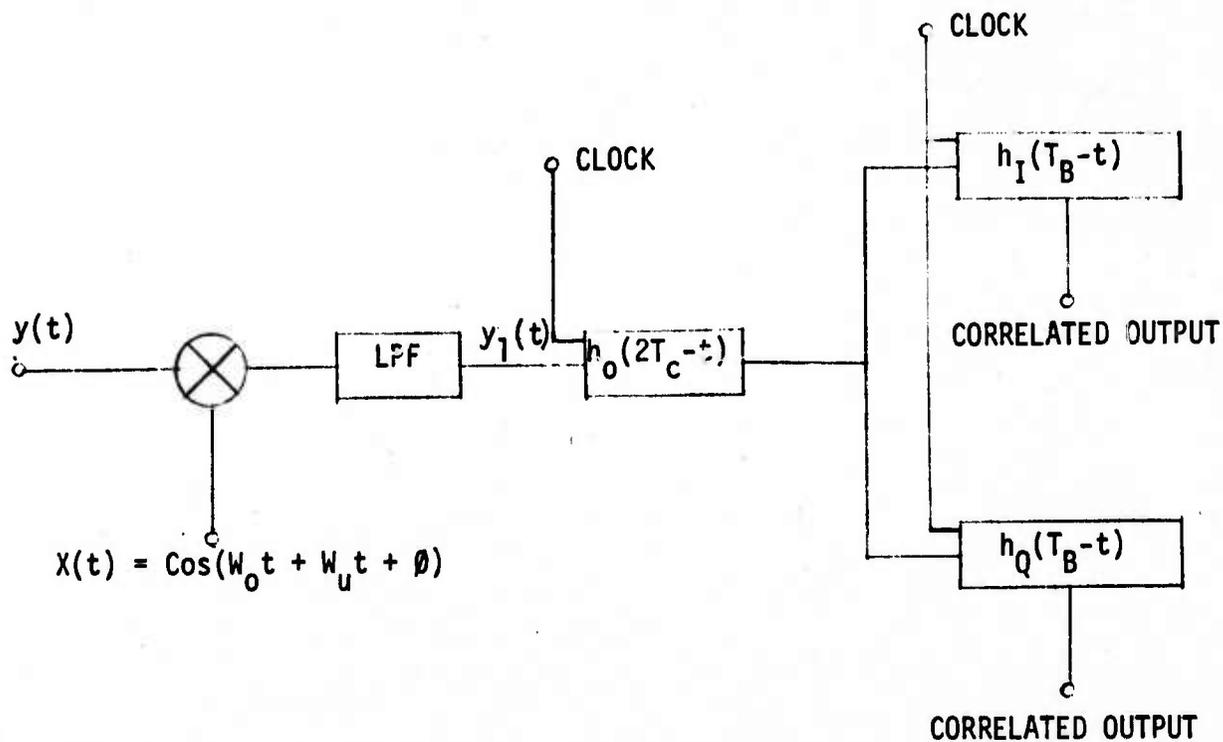
FIGURE 3.5.5 MSK DETECTION AT BASEBAND USING CCDs
