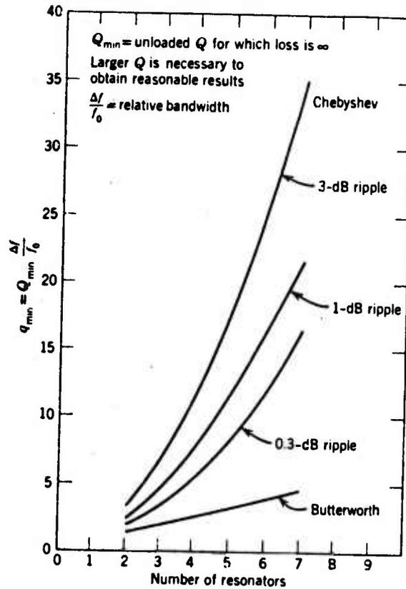
FIGURE 2.4.1 RELATIVE MINIMUM UNLOADED  $Q$  FOR BUTTERWORTH AND CHEBYSHEV FILTERS
