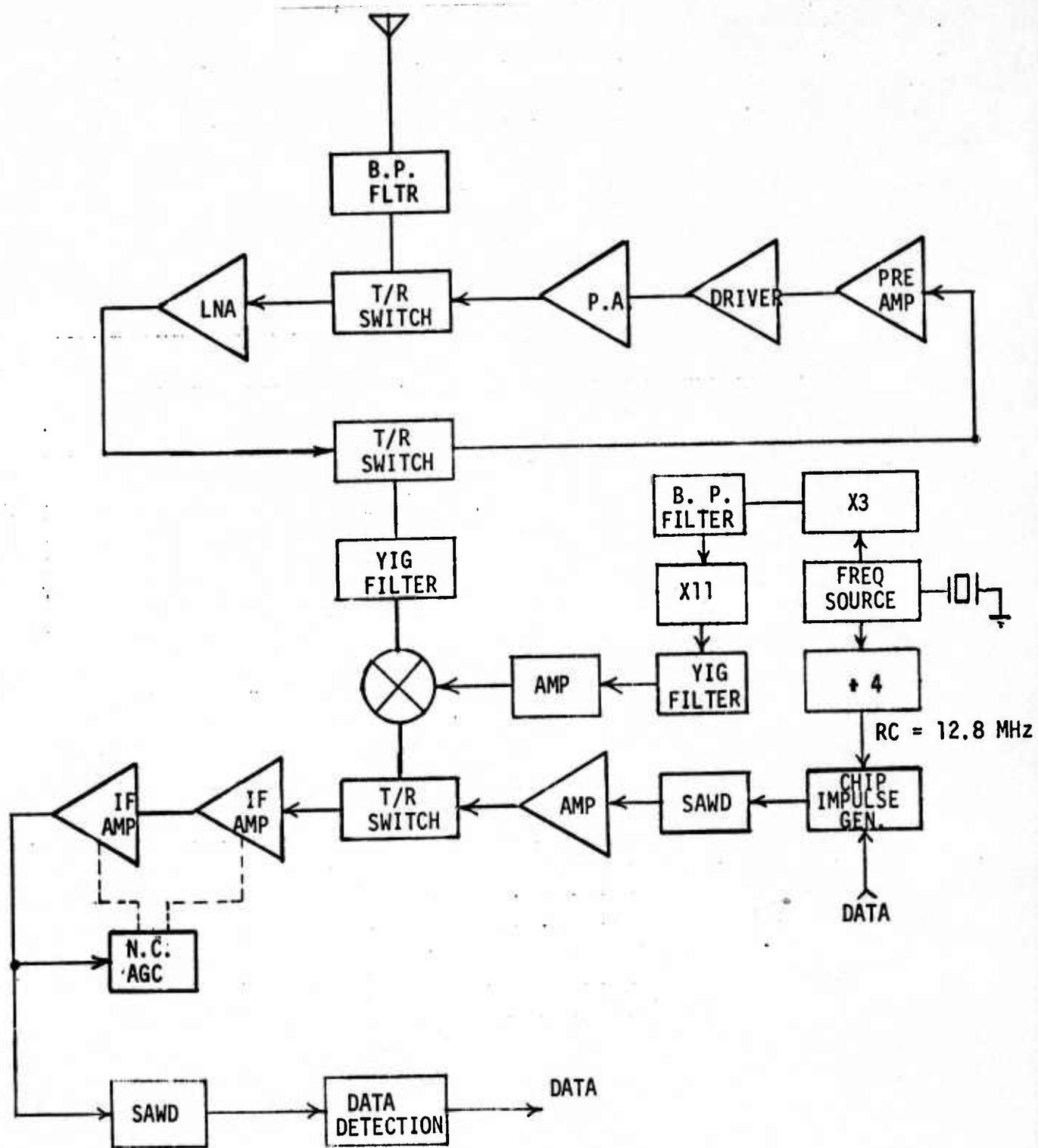
FIGURE 4.1.1 FUNCTIONAL BLOCK DIAGRAM OF RF SECTION
