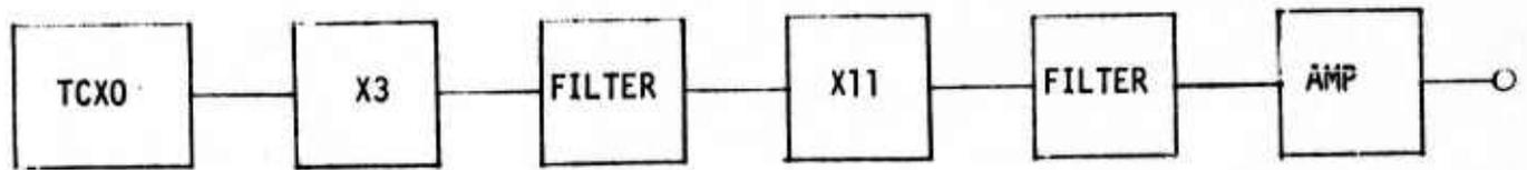
FIGURE 3.3.4 DIRECT MULTIPLICATION APPROACH TO FREQUENCY SYNTHESIS
