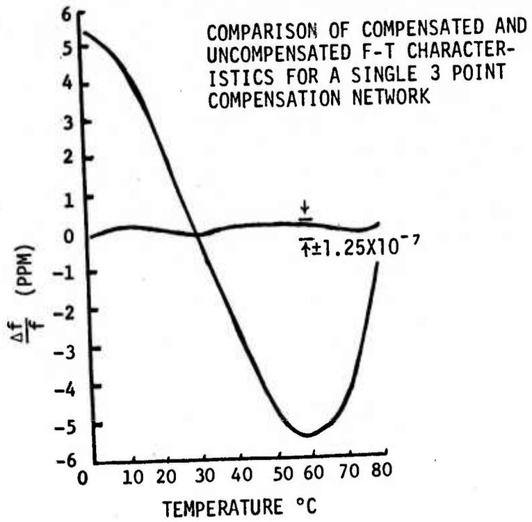
FIGURE 3.3.3 TEMPERATURE - COMPENSATED CRYSTAL OSCILLATOR STABILITY
