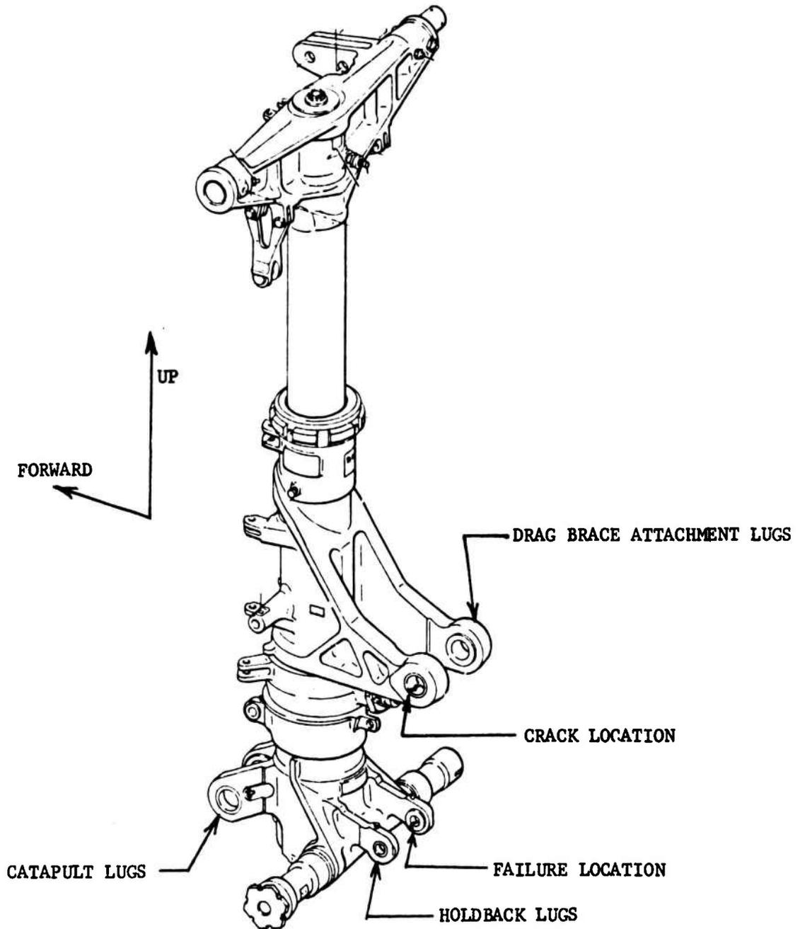
Figure 13. Location of Holdback Lug Failure and Drag Brace Attachment Lug Crack
