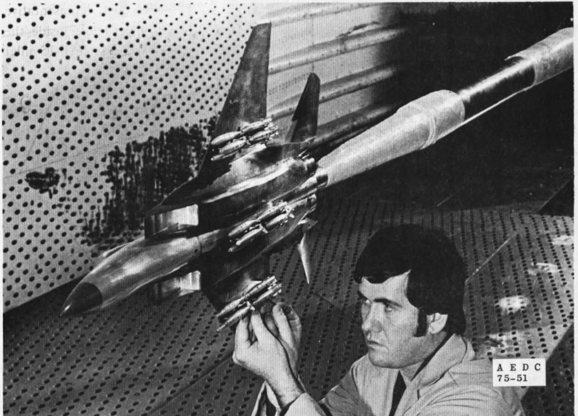
Figure 5. MK-82 bomb configuration.
