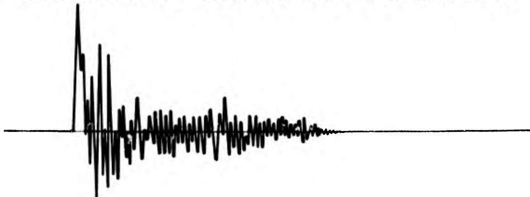
Figure 16. Typical Components of Impact Pressure for Bird Impacts
