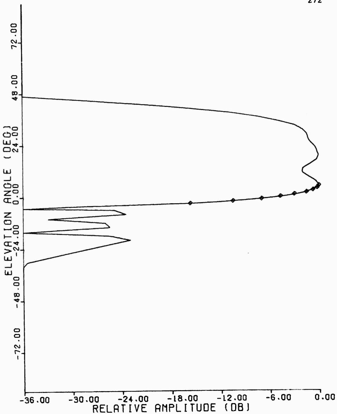
Figure C.37 1030 MHz Elevation Pattern, Westinghouse Antenna
