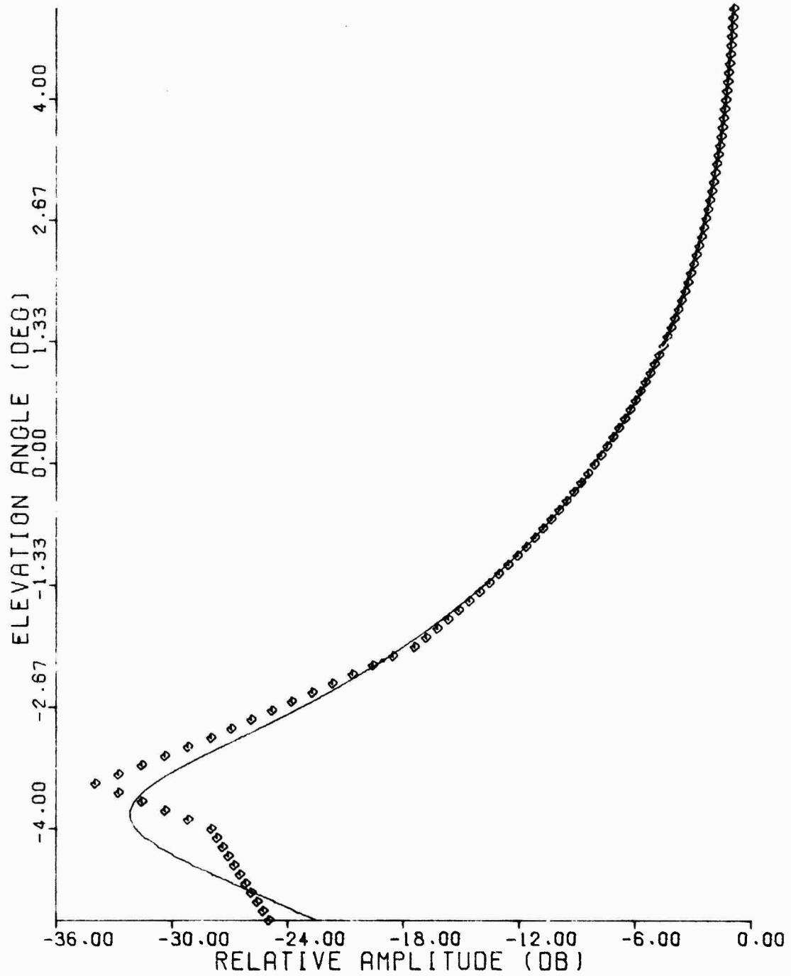
Figure C.56 Least-Squares Fit, 1090 MHz Elevation Pattern,
