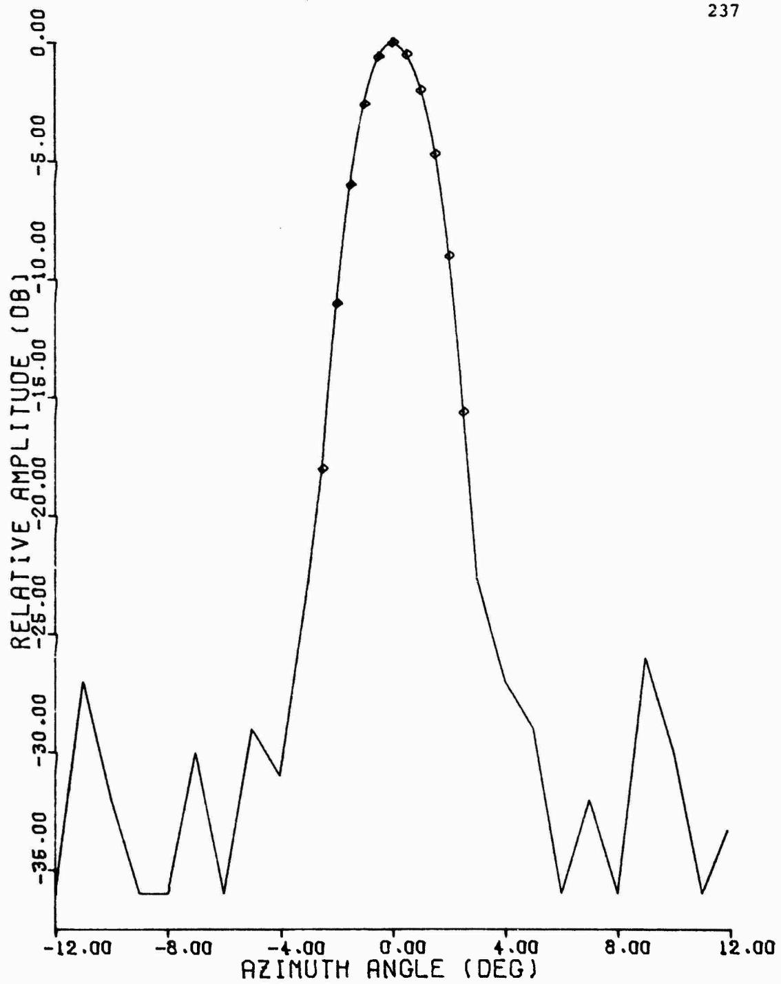
Figure C.2 1030 MHz Azimuth Pattern, FA-8043 Antenna,
