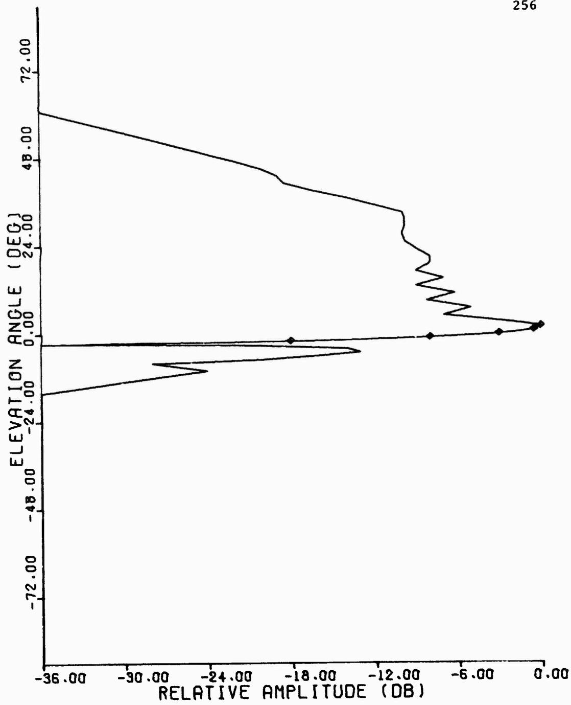
Figure C.21 1030 MHz Elevation Pattern, ARSR Beacon Feed
