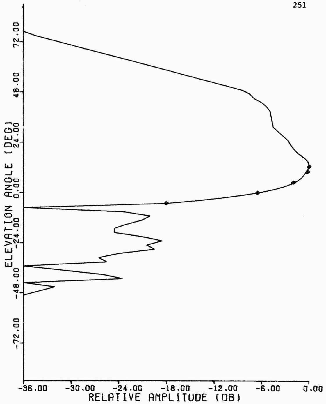
Figure C.16 1030 MHz Elevation Pattern, Hazeltine Omni Antenna
