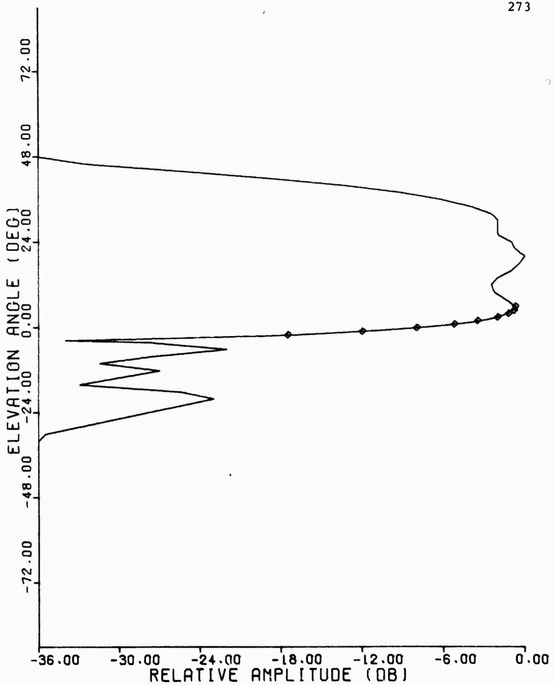
Figure C.38 1090 MHz Elevation Pattern, Westinghouse Antenna
