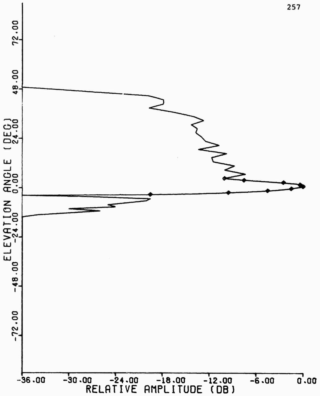
Figure C.22 1090 MHz Elevation Pattern, ARSR Beacon Feed
