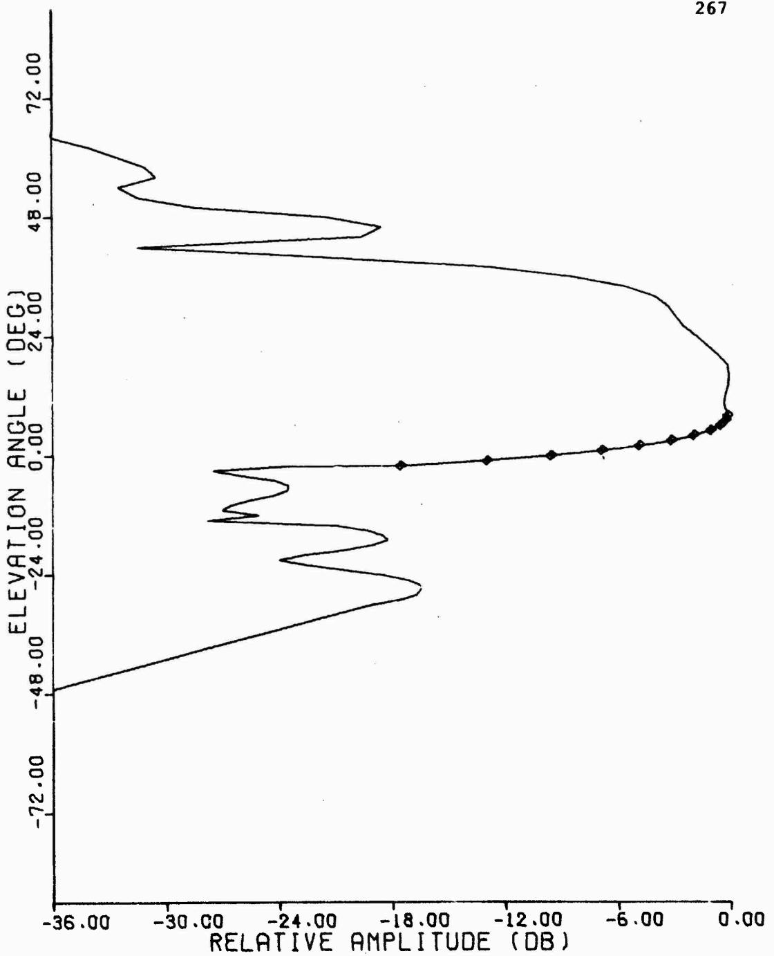
Figure C.32 1030 MHz Elevation Pattern, TI Separate Rotator Omni
