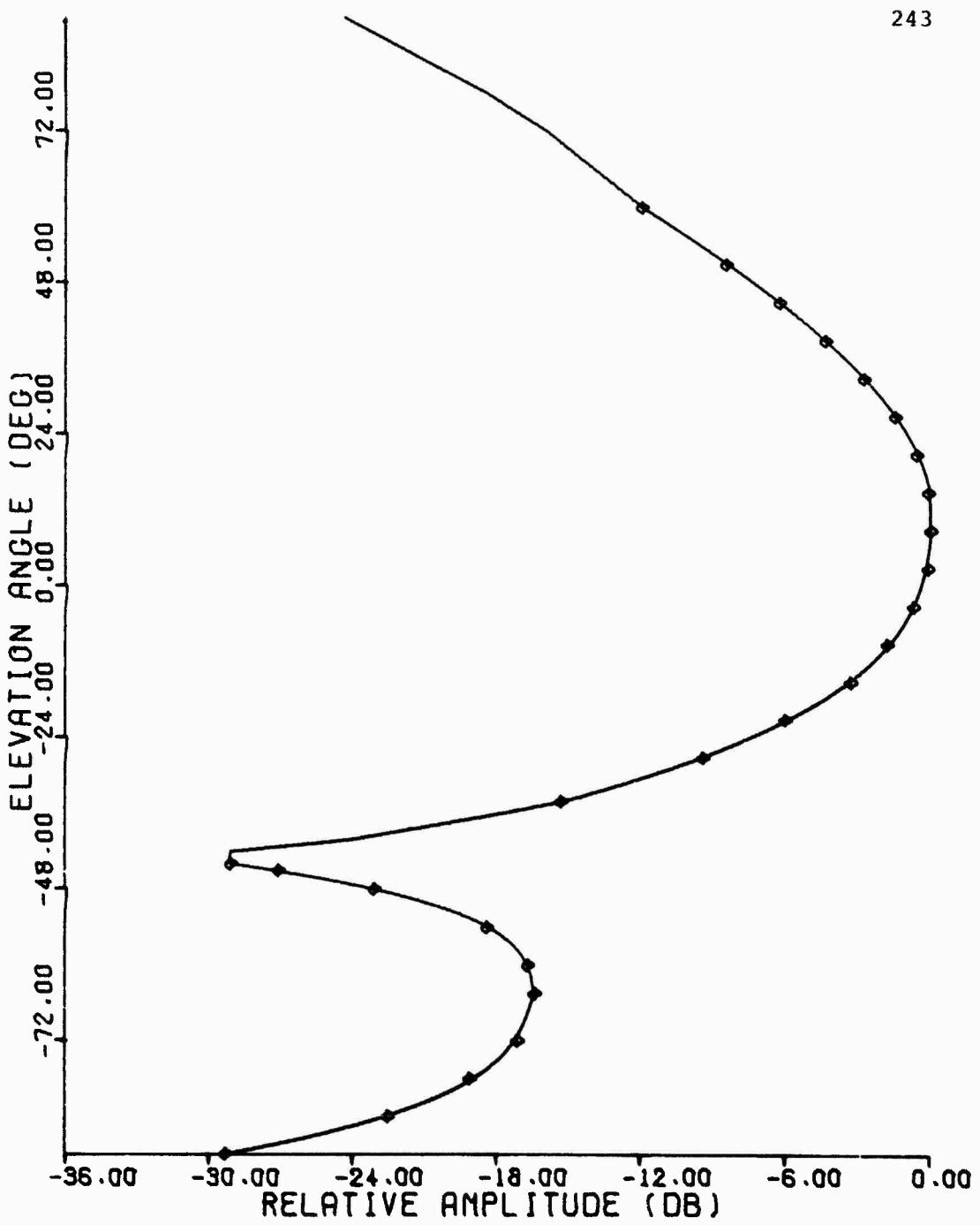
Figure C.8 1030 MHz Elevation Pattern, FA-8045 Antenna
