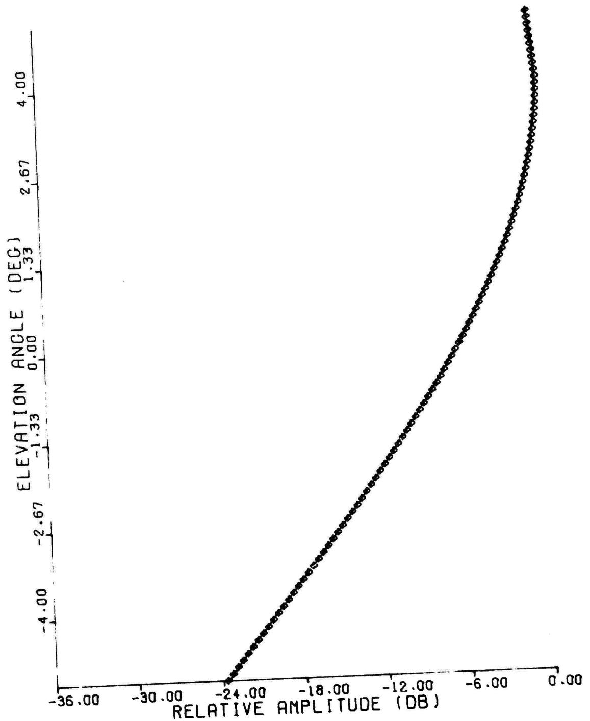
Figure C.53 Least-Squares Fit, 1090 MHz Elevation Pattern,
