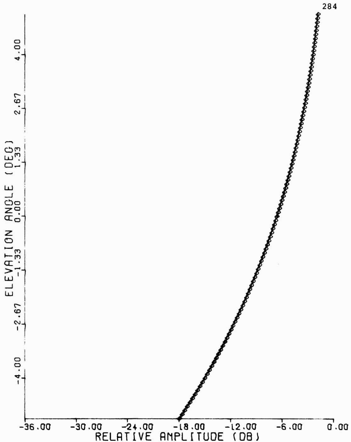
Figure C.48 Least-Squares Fit, 1030 MHz Elevation Pattern,
