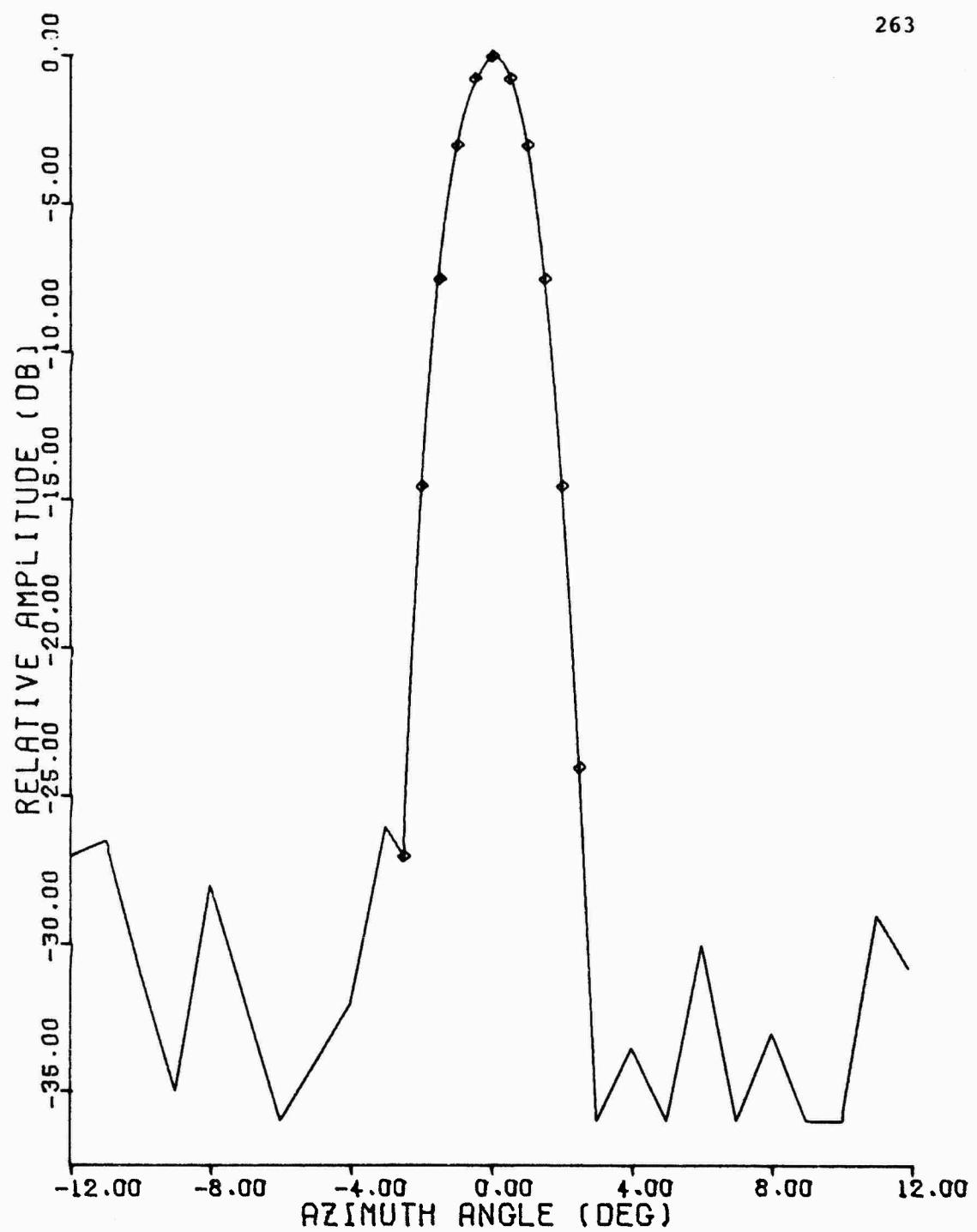
Figure C.28 1090 MHz Azimuth Pattern, TI Separate Rotator,
