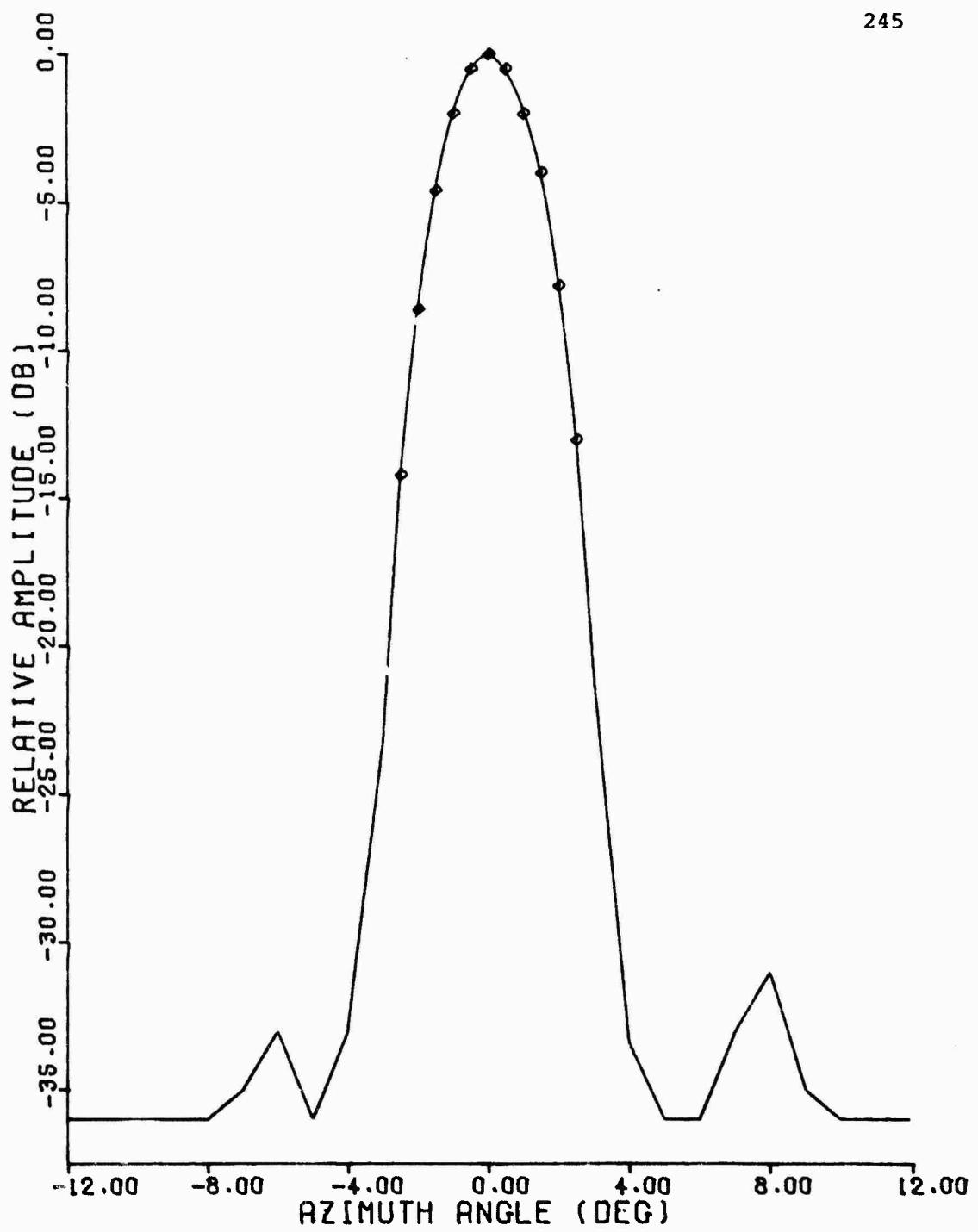
Figure C.10 1030 MHz Azimuth Pattern, Hazeltine Antenna,
