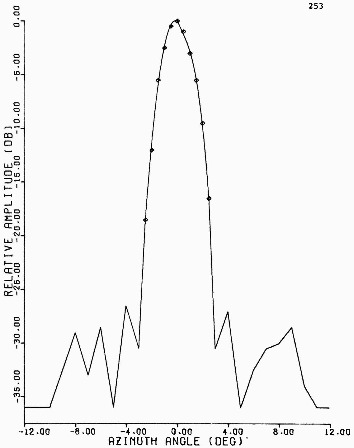
Figure C.18 1030 MHz Azimuth Pattern, ARSR Beacon Feed,
