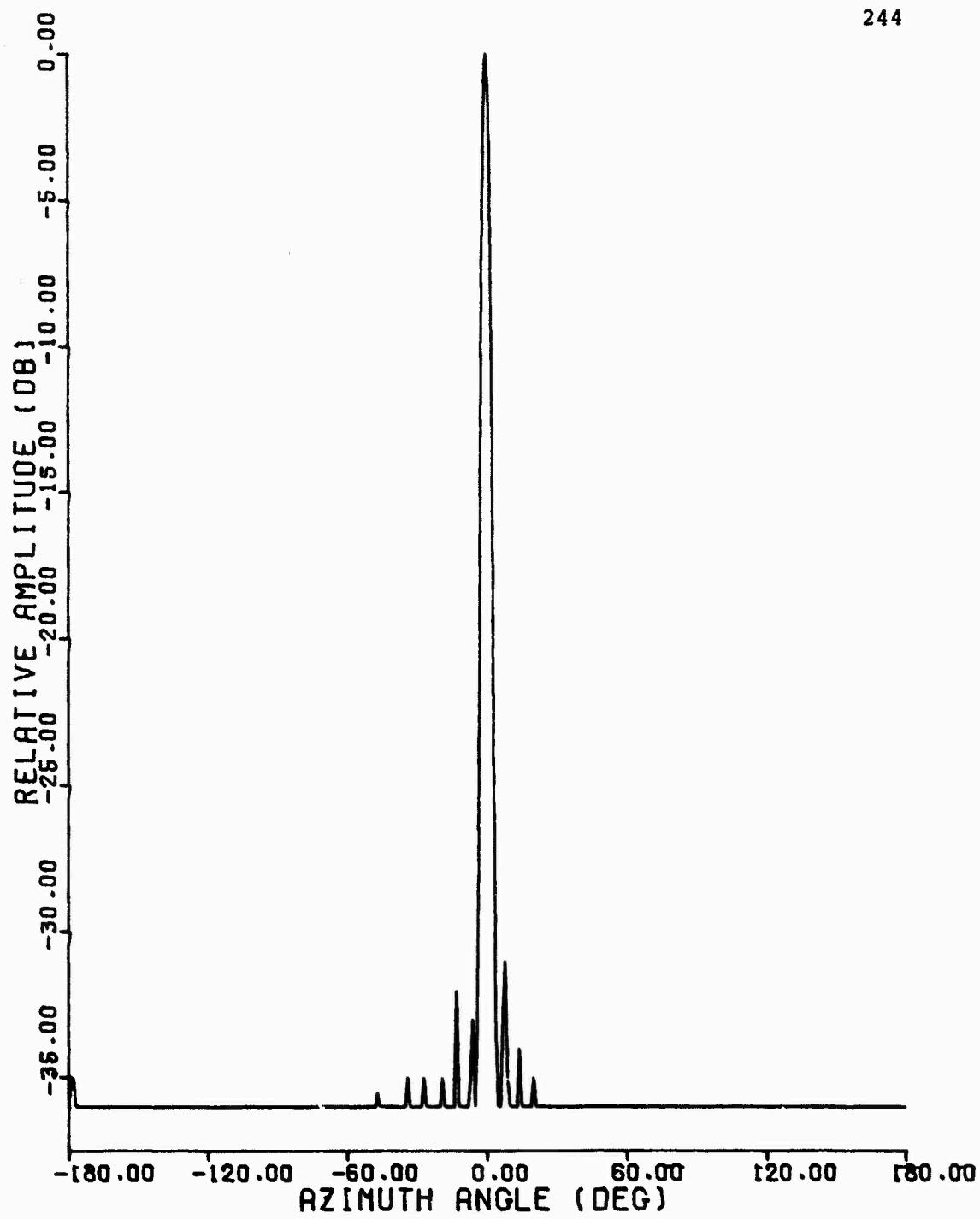
Figure C.9 1030 MHz Azimuth Pattern, Hazeltine Antenna,
