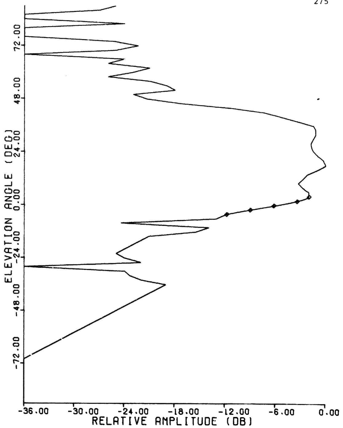
Figure C.40 1030 MHz Elevation Pattern, Westinghouse Omni
