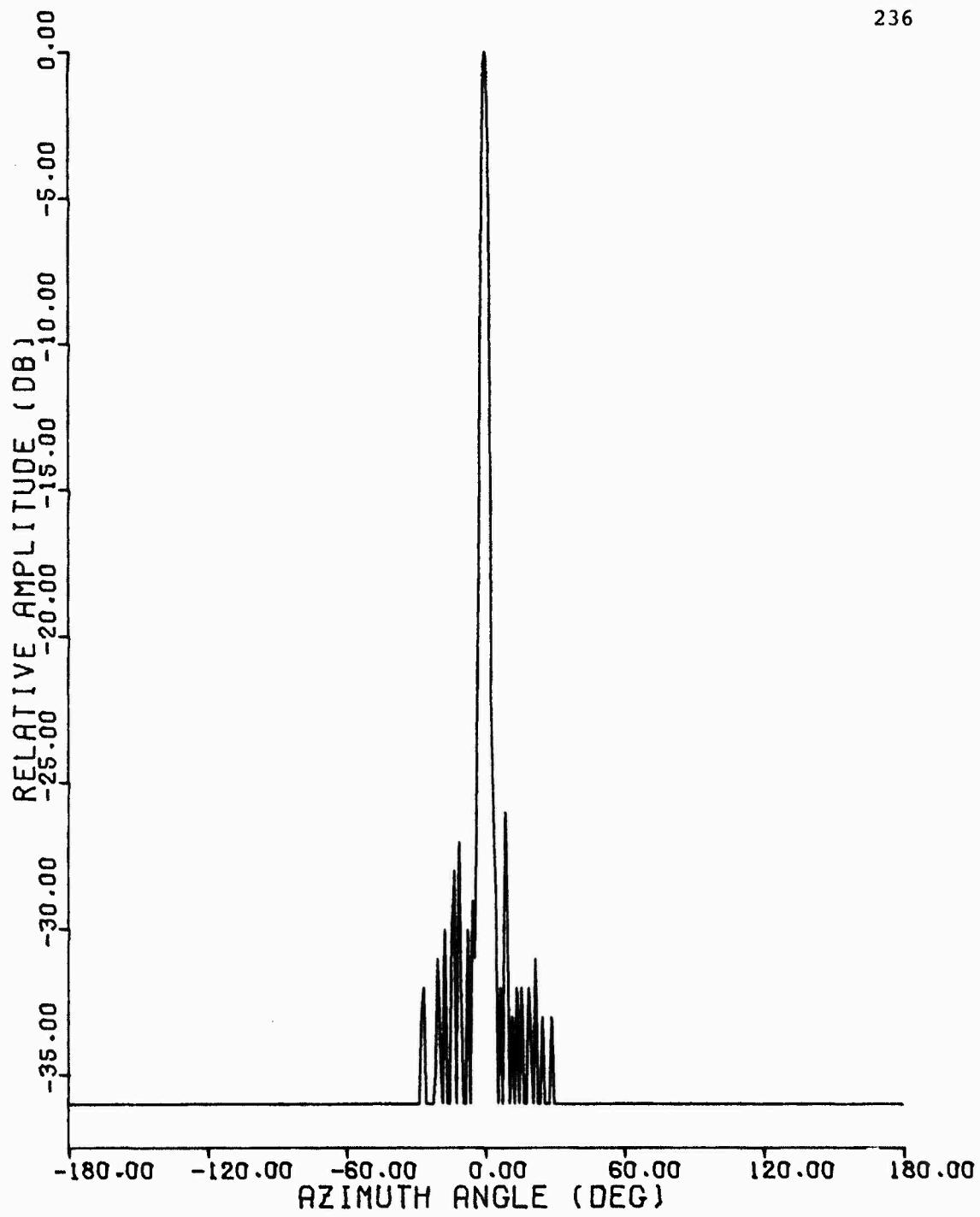
Figure C.1 1030 MHz Azimuth Pattern, FA-8043 Antenna,
