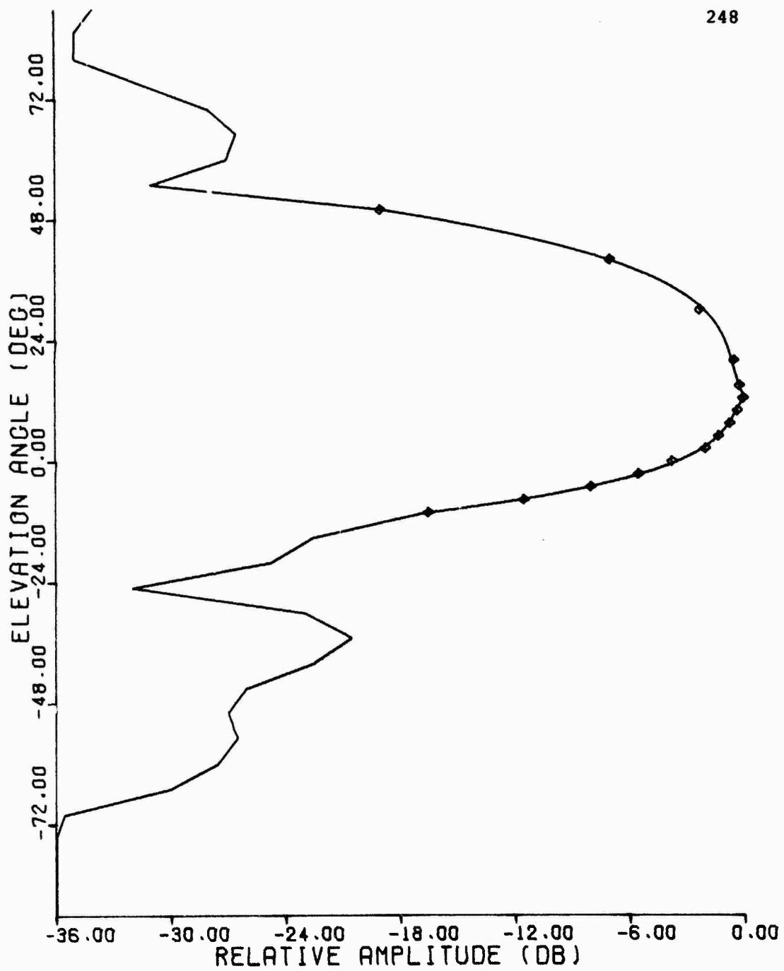
Figure C.13 1030 MHz Elevation Pattern, Hazeltine Antenna
