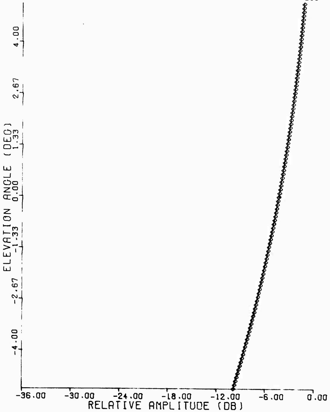
Figure C.47 Least-Squares Fit, 1090 MHz Elevation Pattern,
