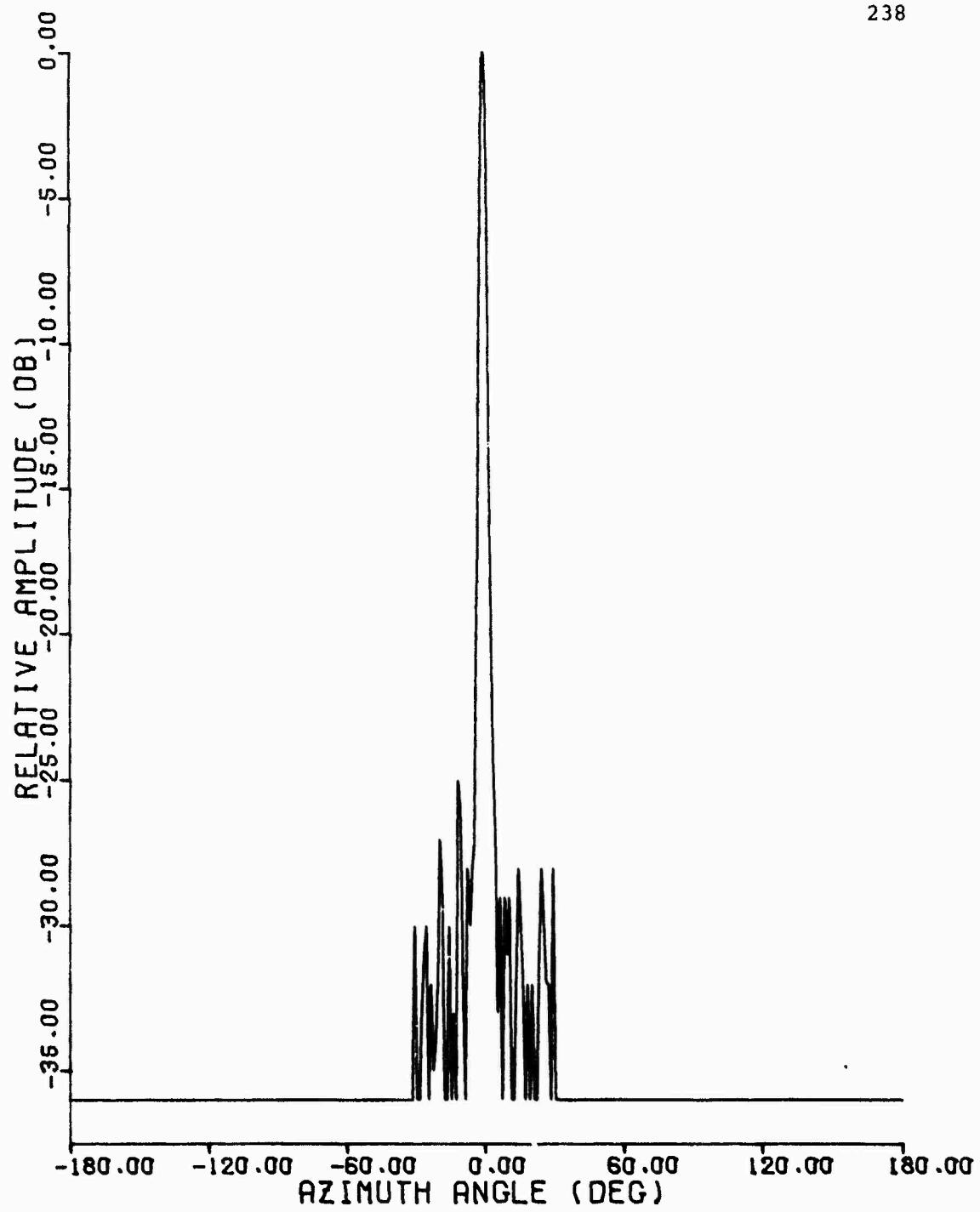
Figure C.3 1090 MHz Azimuth Pattern, FA-8043 Antenna,
