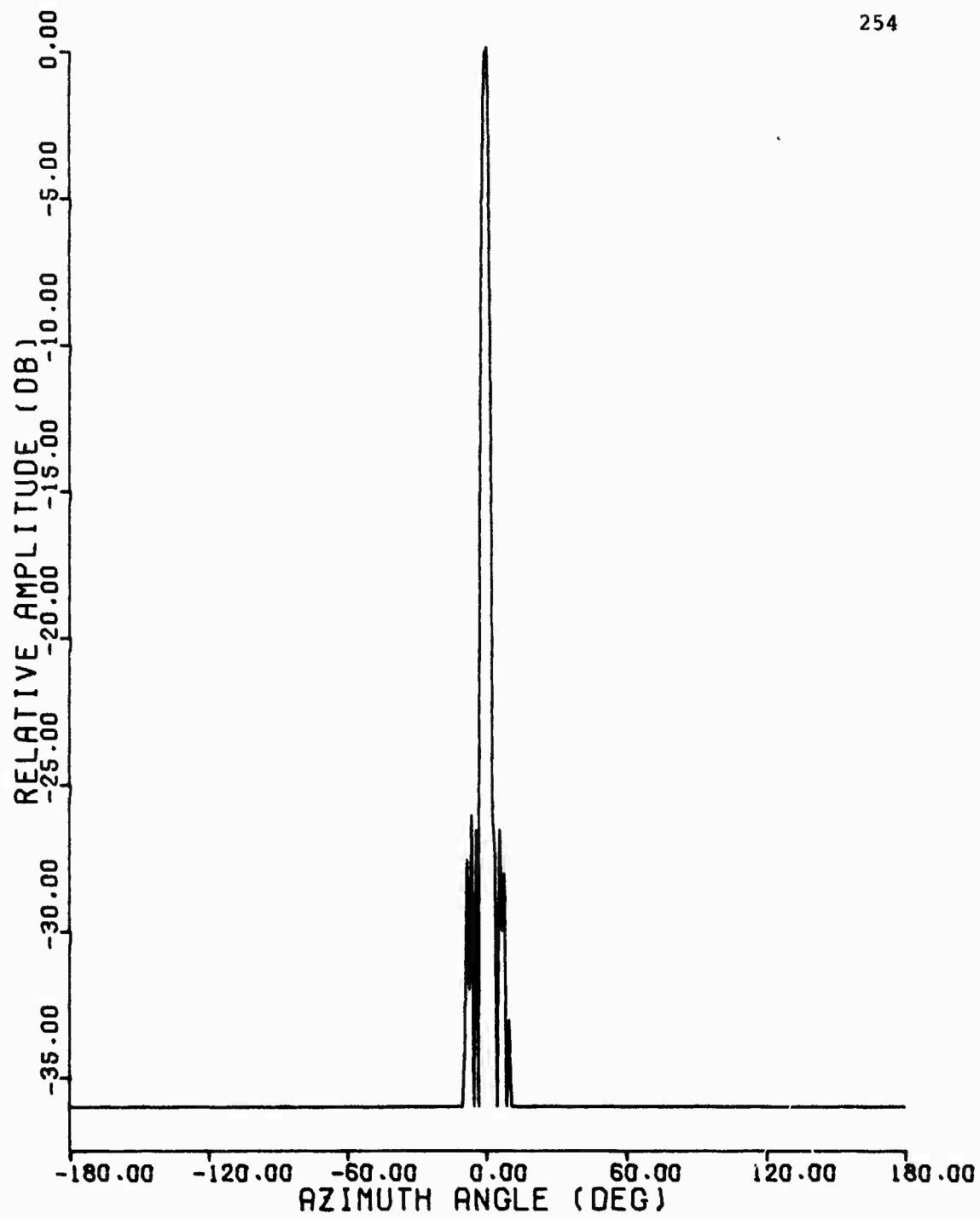
Figure C.19 1090 MHz Azimuth Pattern, ARSR Beacon Feed,
