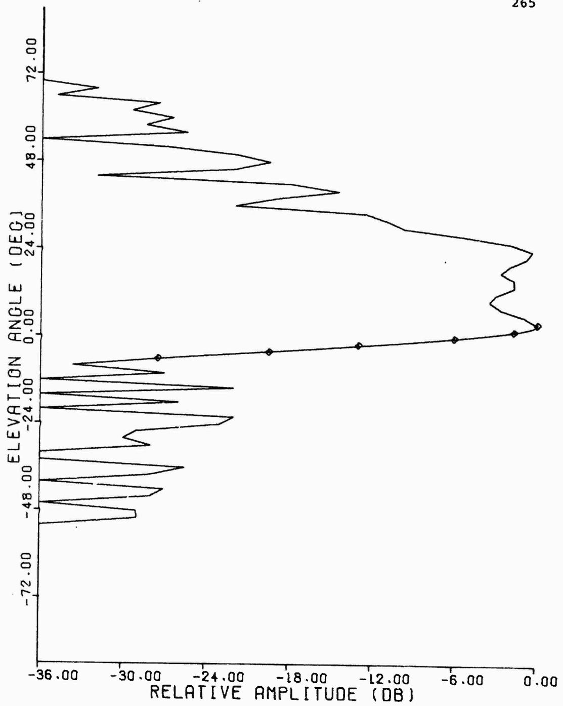
Figure C.30 1090 MHz Elevation Pattern, TI Separate Rotator
