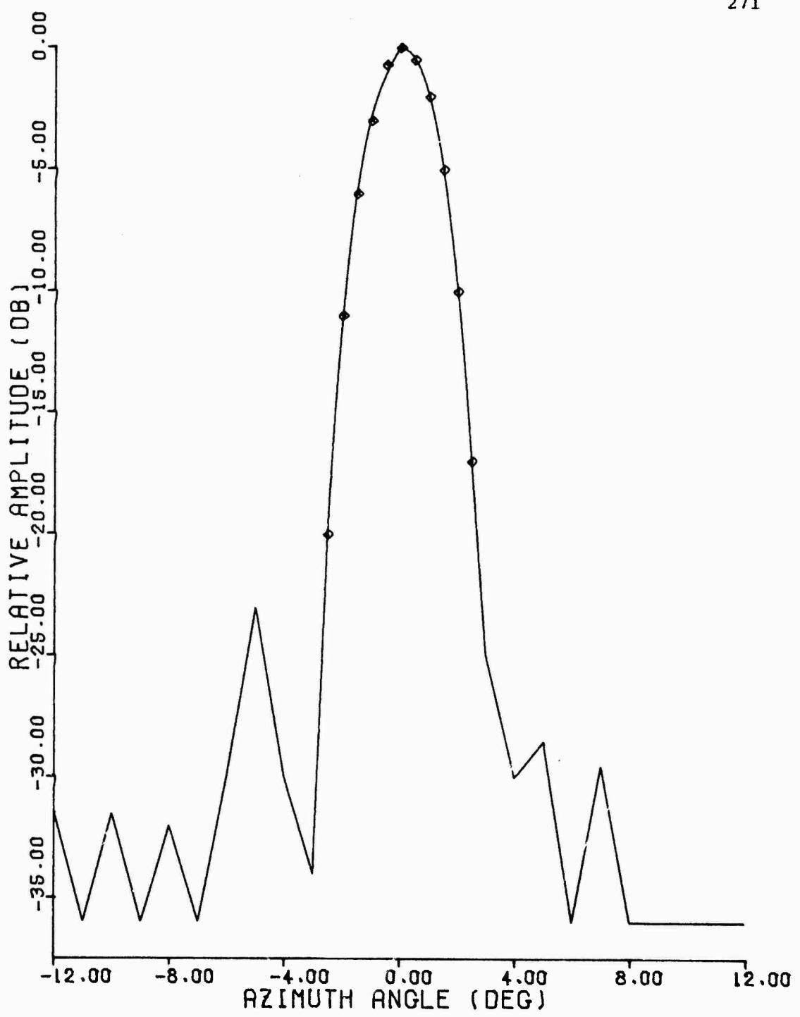
Figure C.36 1090 MHz Azimuth Pattern, Westinghouse Antenna,
