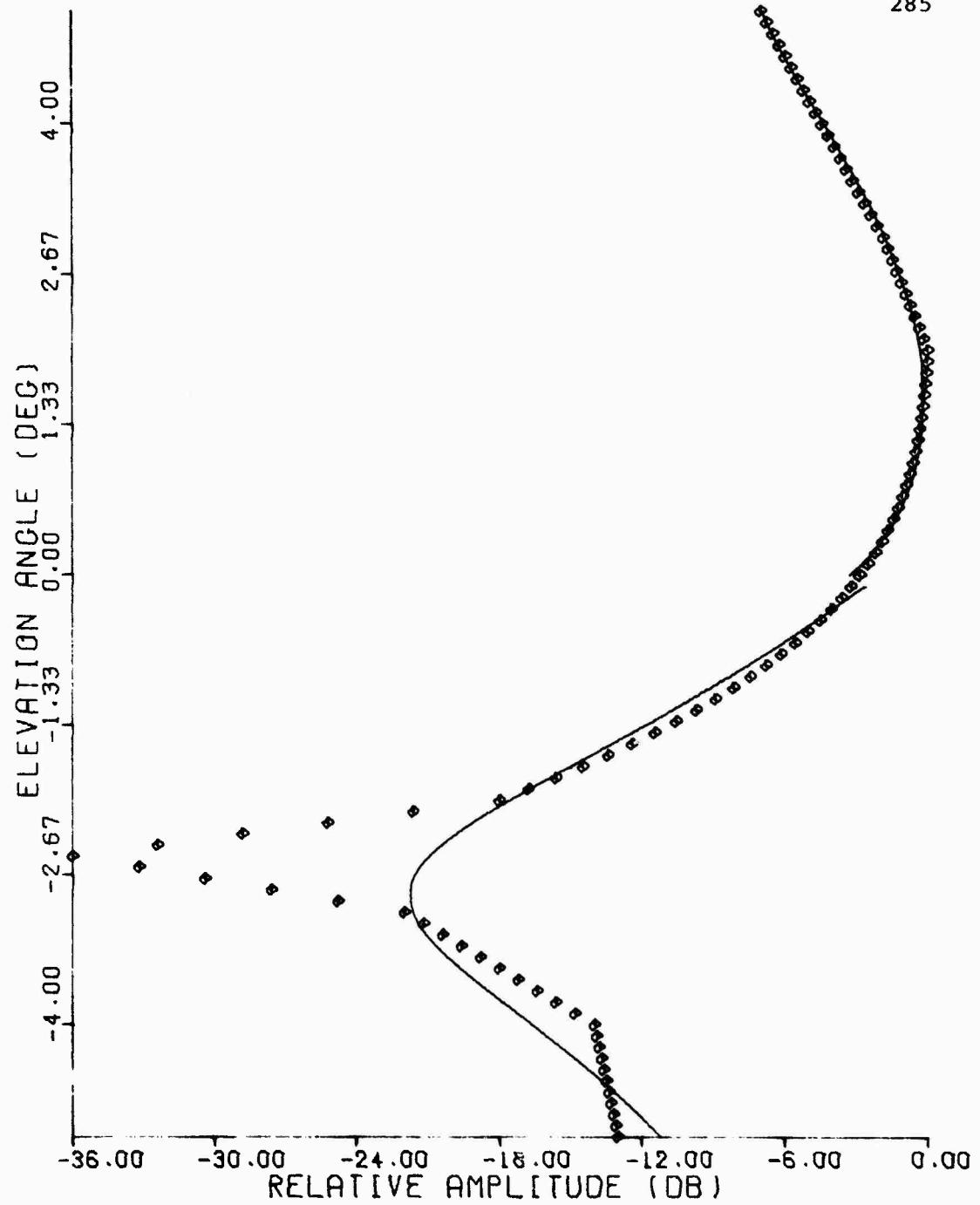
Figure C.49 Least-Squares Fit, 1030 MHz Elevation Pattern,
