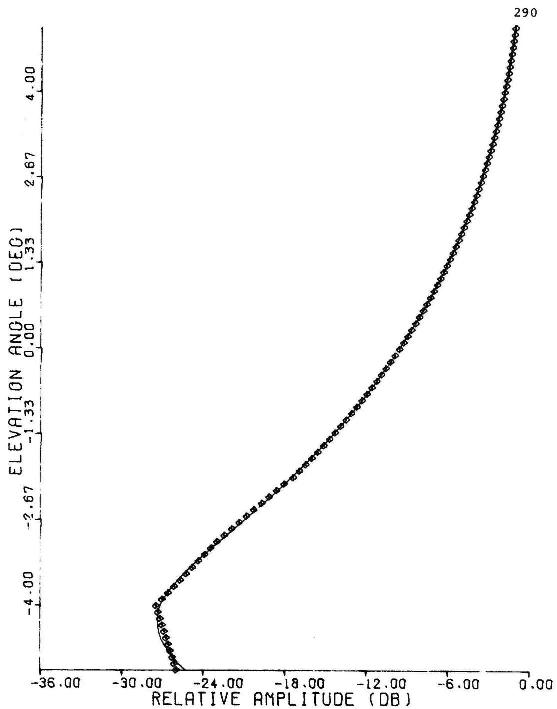
Figure C.54 Least-Squares Fit, 1030 MHz Elevation Pattern,
