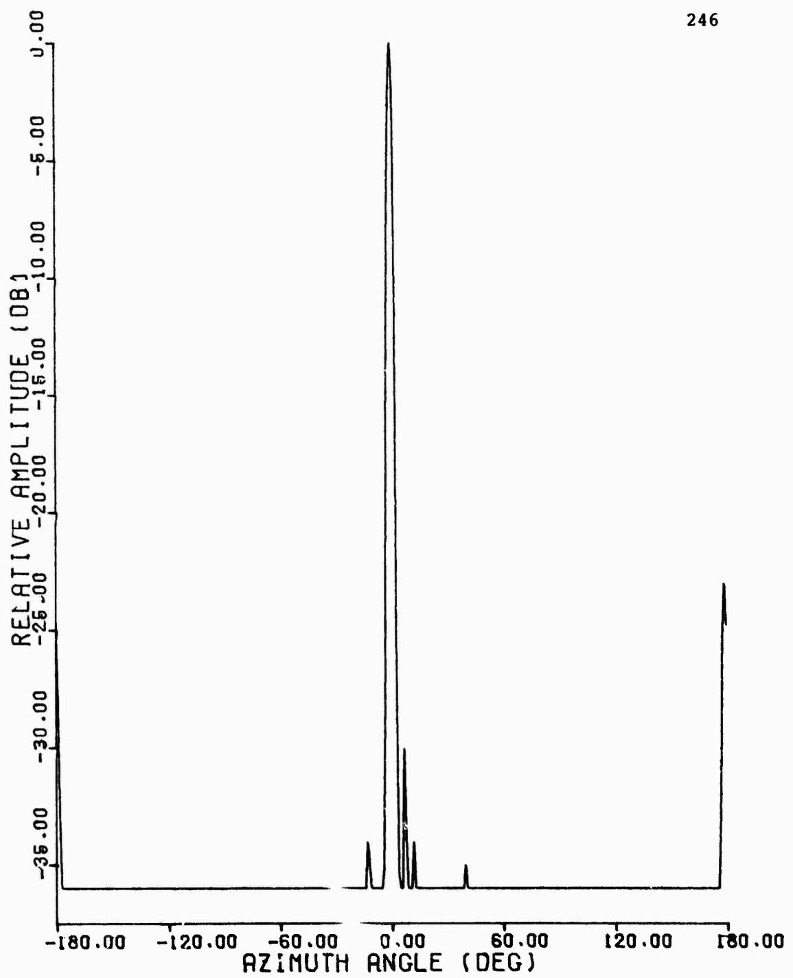
Figure C.11 1090 MHz Azimuth Pattern, Hazeltine Antenna,
