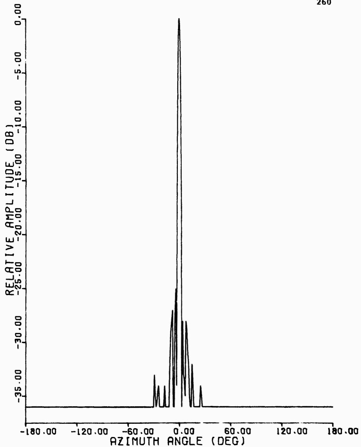
Figure C.25 1030 MHz Azimuth Pattern, TI Separate Rotator,
