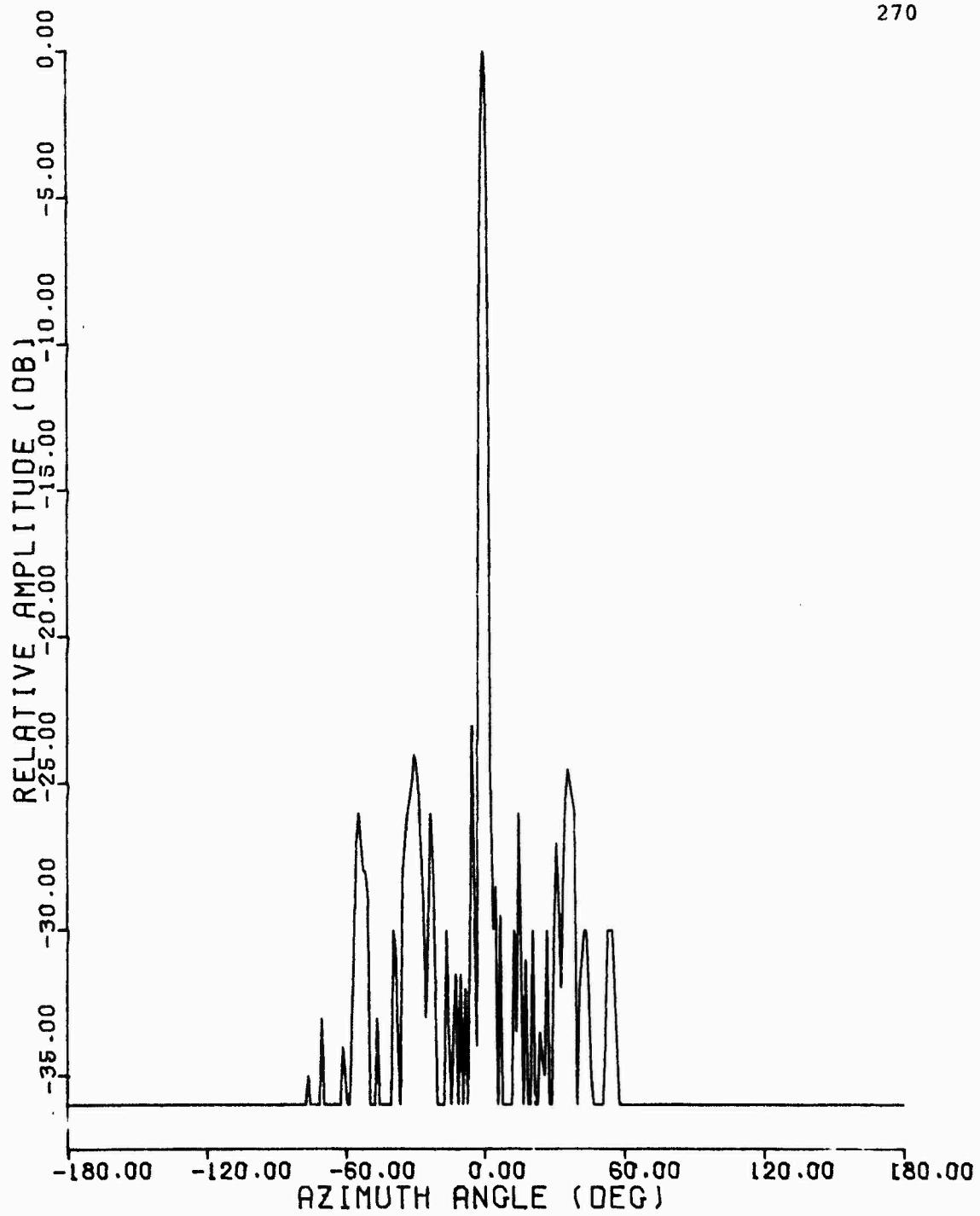
Figure C.35 1090 MHz Azimuth Pattern, Westinghouse Antenna,
