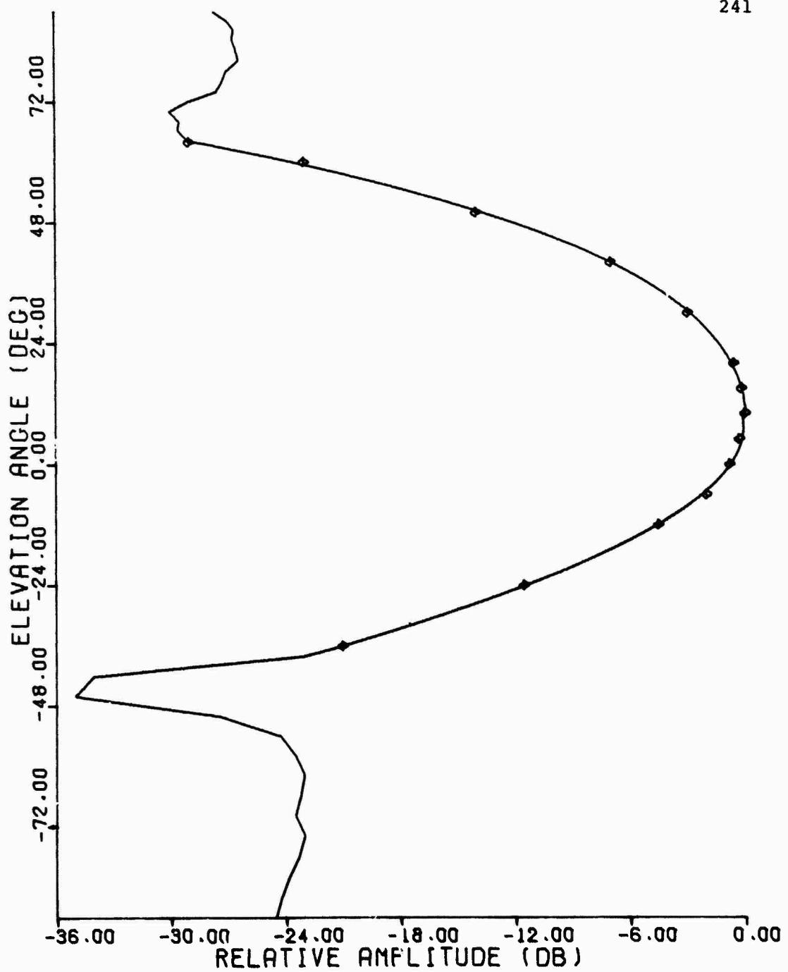
Figure C.6 1090 MHz Elevation Pattern, FA-8043 Antenna
