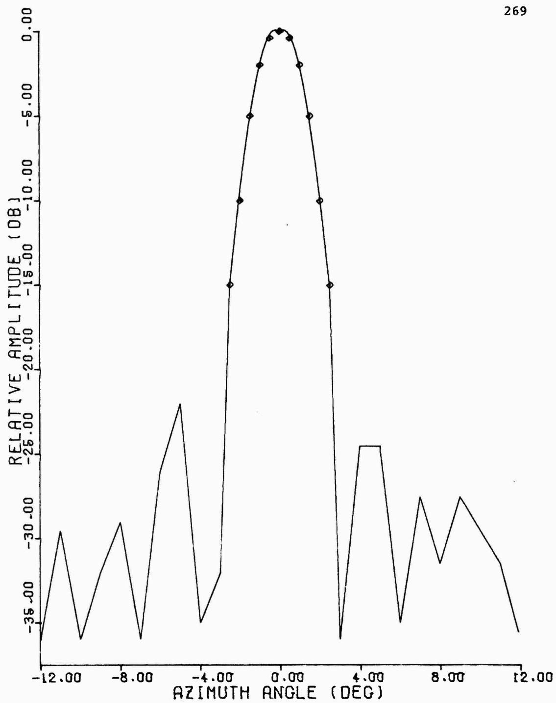
Figure C.34 1030 MHz Azimuth Pattern, Westinghouse Antenna,
