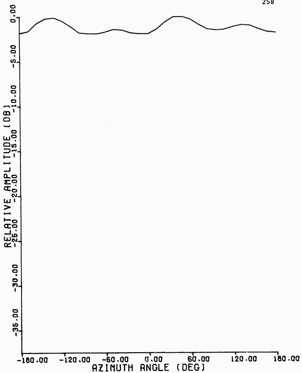
Figure C.23 1030 MHz Azimuth Pattern, ARSR Omni Antenna
