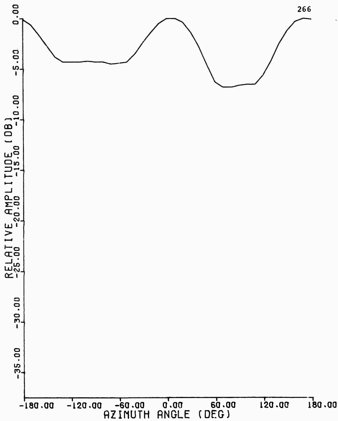
Figure C.31 1030 MHz Azimuth Pattern, TI Separate Rotator Omni
