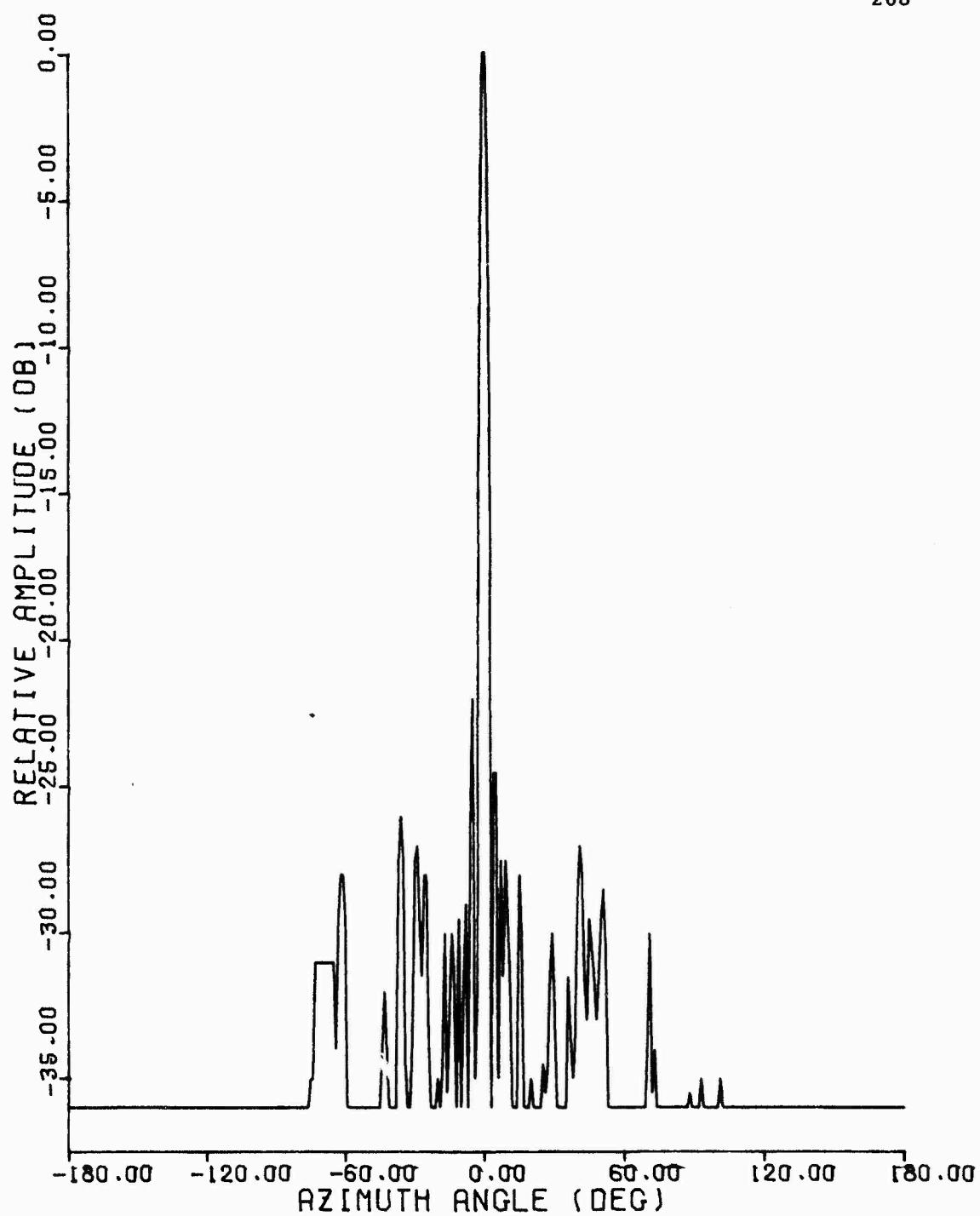
Figure C.33 1030 MHz Azimuth Pattern, Westinghouse Antenna,
