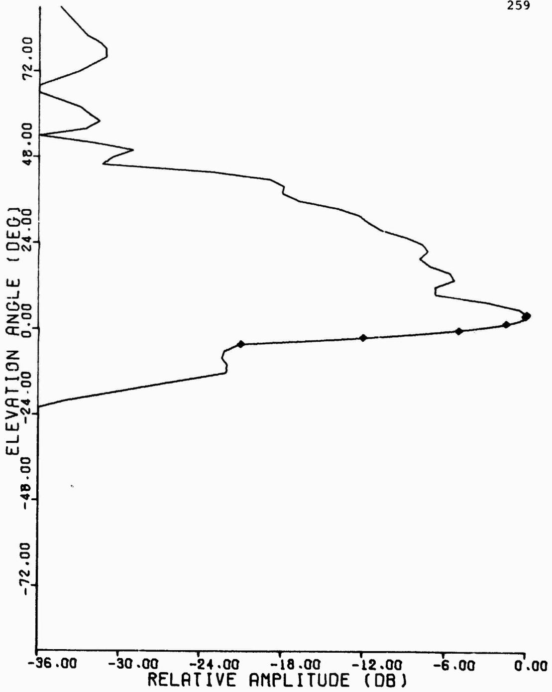
Figure C.24 1030 MHz Elevation Pattern, ARSR Omni Antenna
