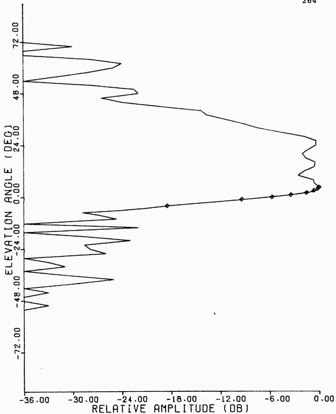
Figure C.29 1030 MHz Elevation Pattern, TI Separate Rotator
