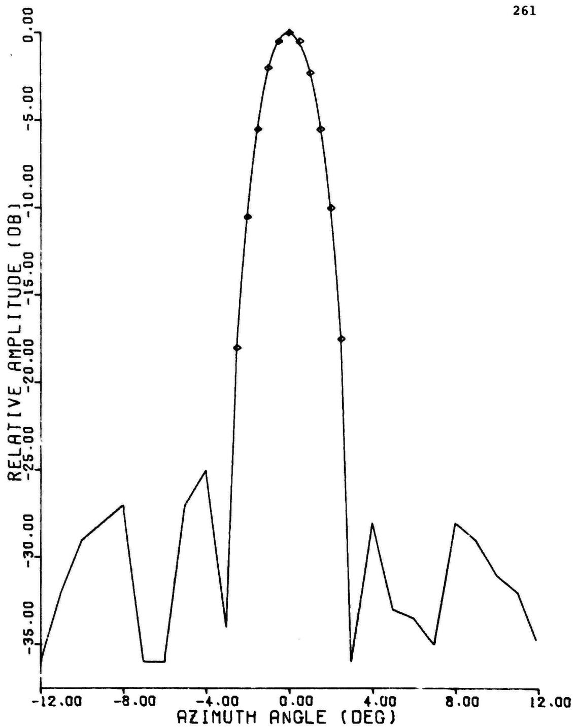
Figure C.26 1030 MHz Azimuth Pattern, TI Separate Rotator,
