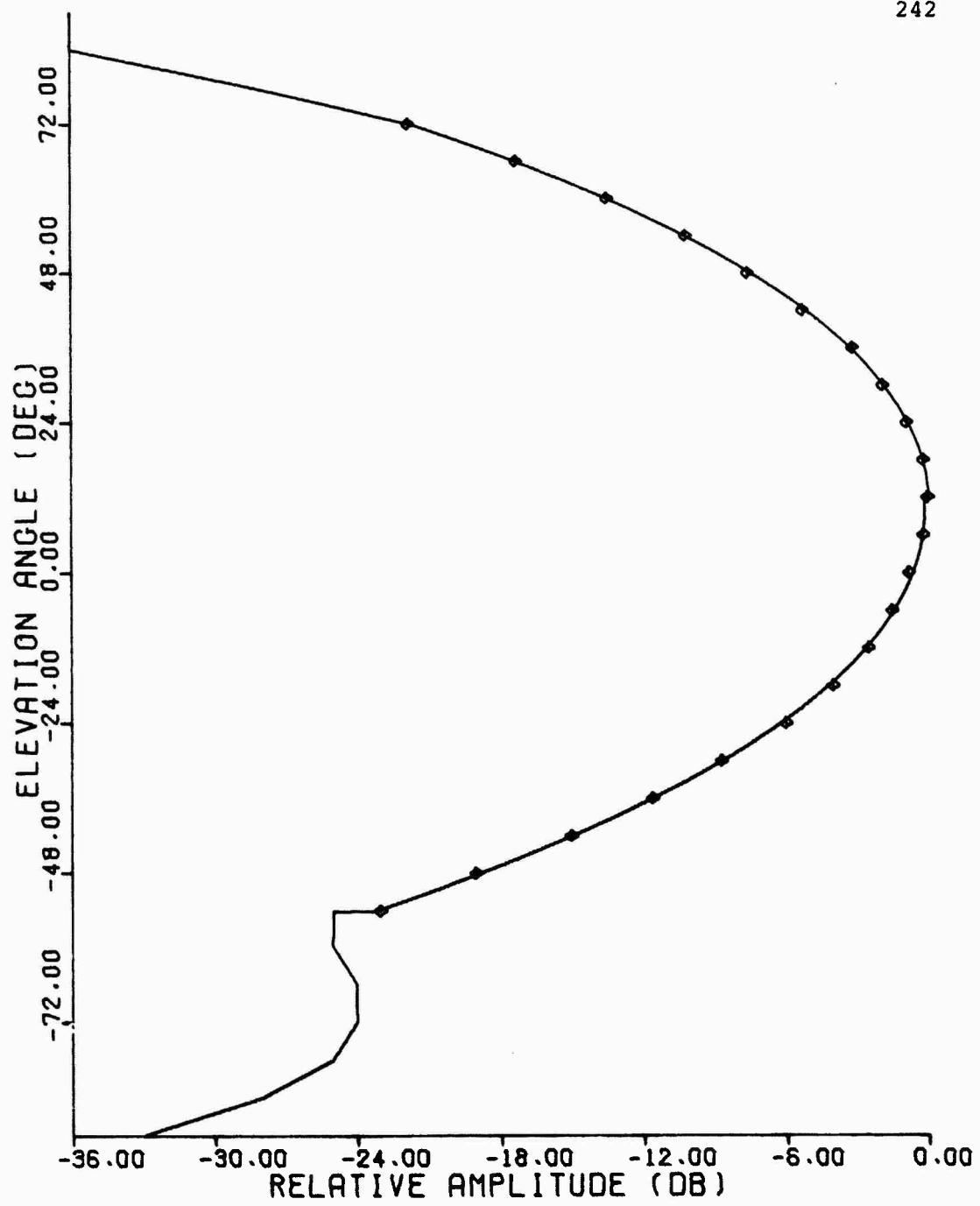
Figure C.7 1030 MHz Elevation Pattern, FA-8044 Antenna
