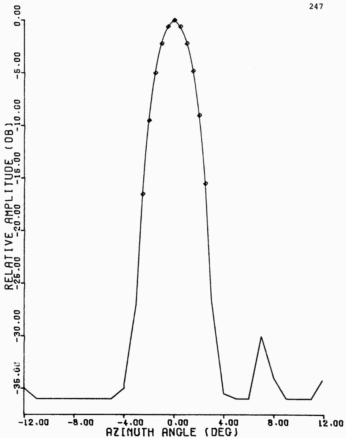
Figure C.12 1090 MHz Azimuth Pattern, Hazeltine Antenna,
