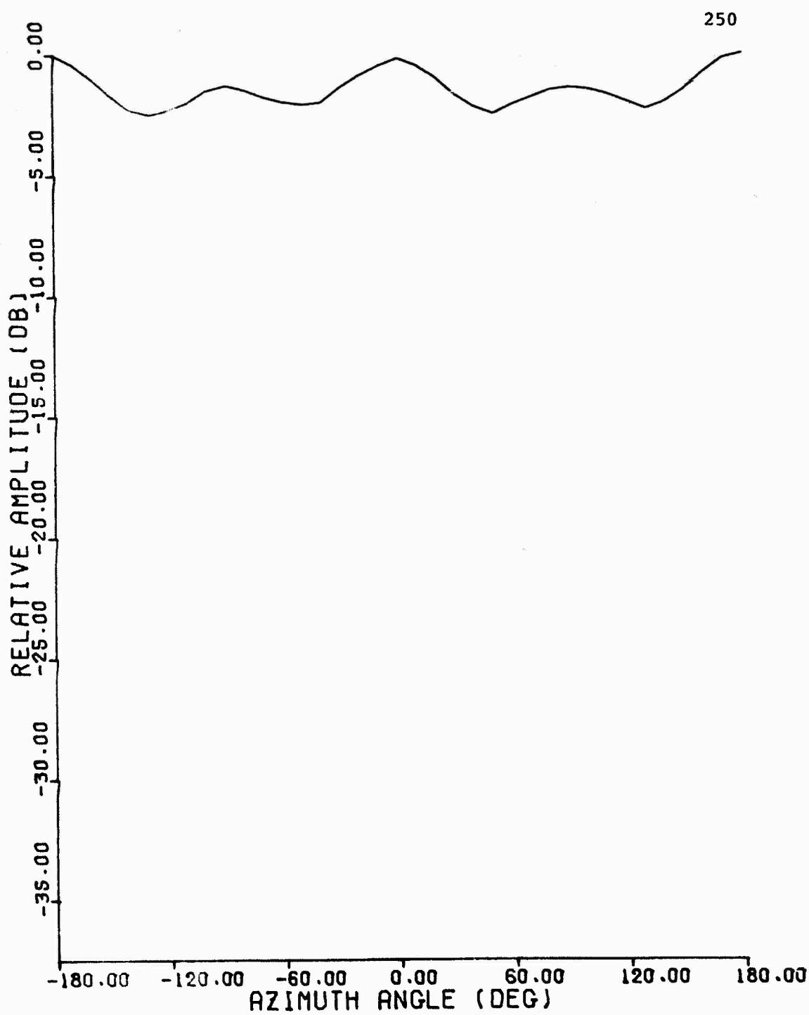
Figure C.15 1030 MHz Azimuth Pattern, Hazeltine Omni Antenna
