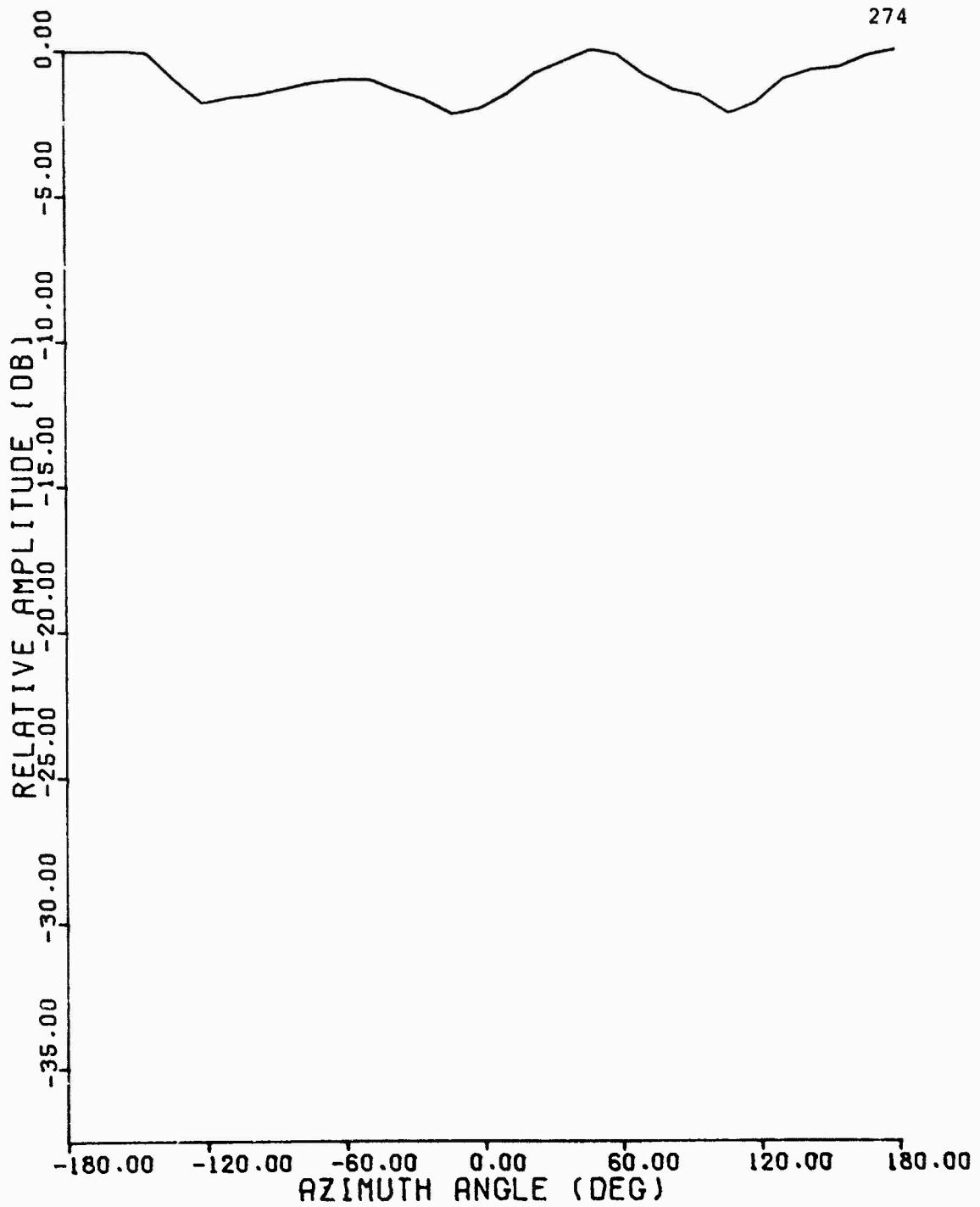
Figure C.39 1030 MHz Azimuth Pattern, Westinghouse Omni
