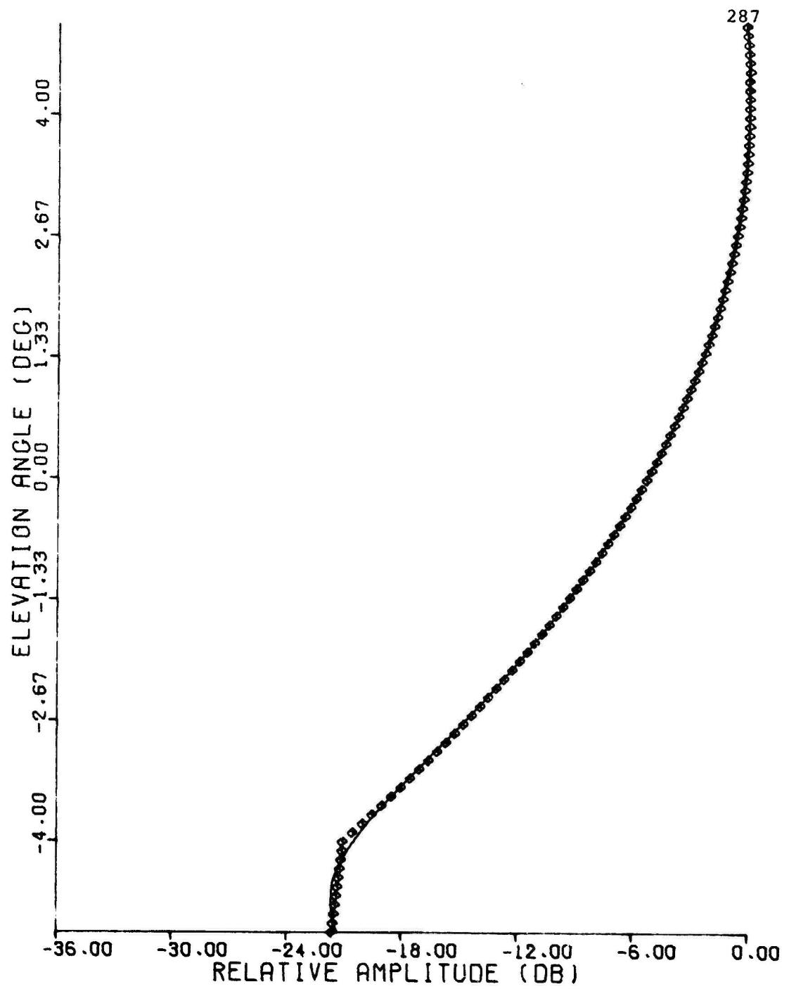
Figure C.51 Least-Squares Fit, 1030 MHz Elevation Pattern,
