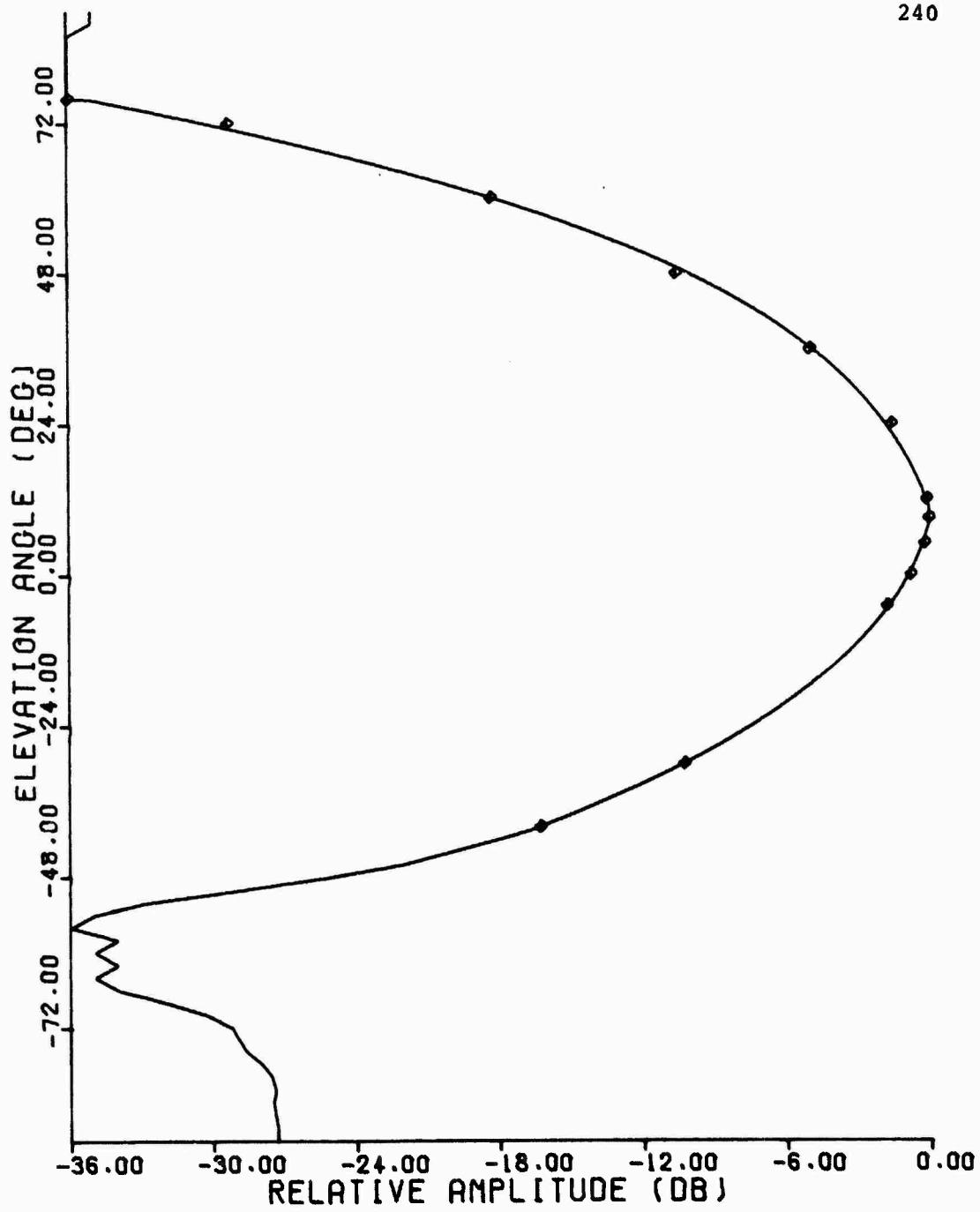
Figure C.5 1030 MHz Elevation Pattern, FA-8043 Antenna
