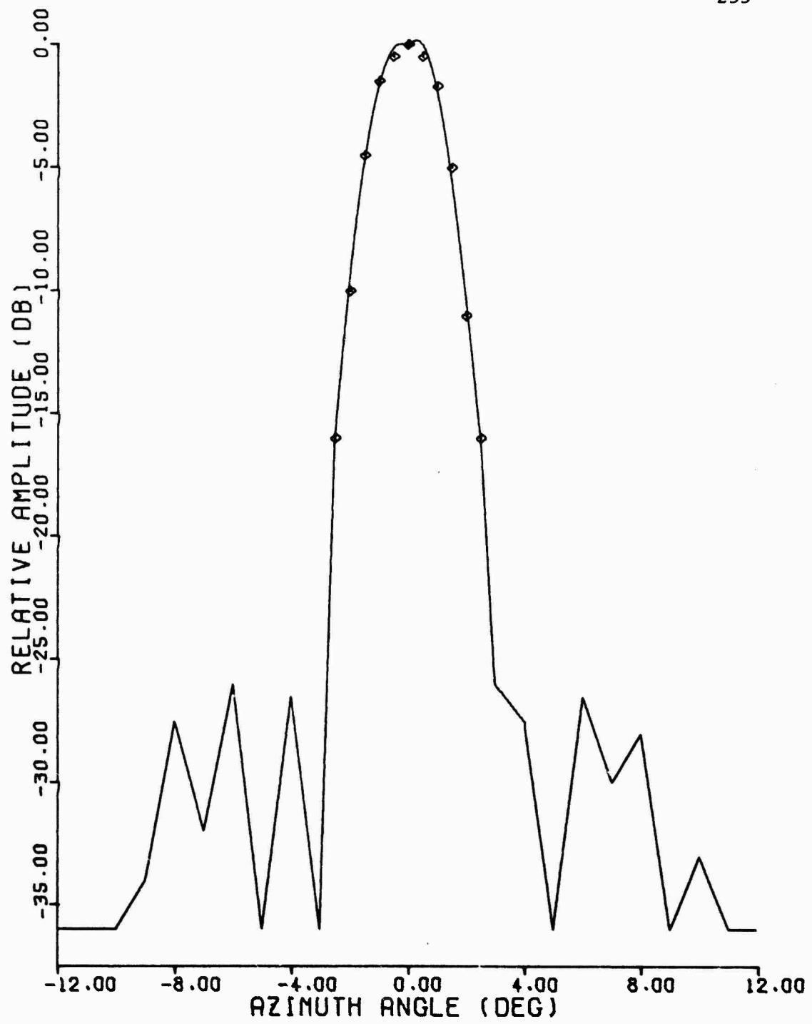
Figure C.20 1090 MHz Azimuth Pattern, ARSR Beacon Feed,
