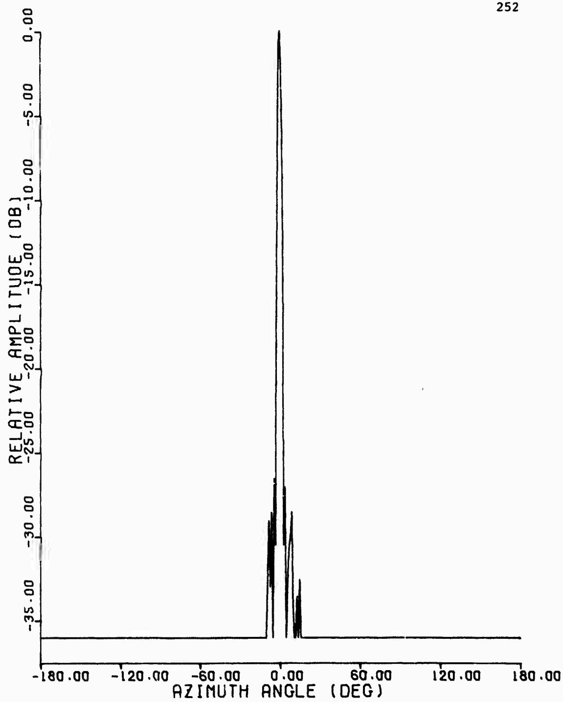
Figure C.17 1030 MHz Azimuth Pattern, ARSR Beacon Feed,
