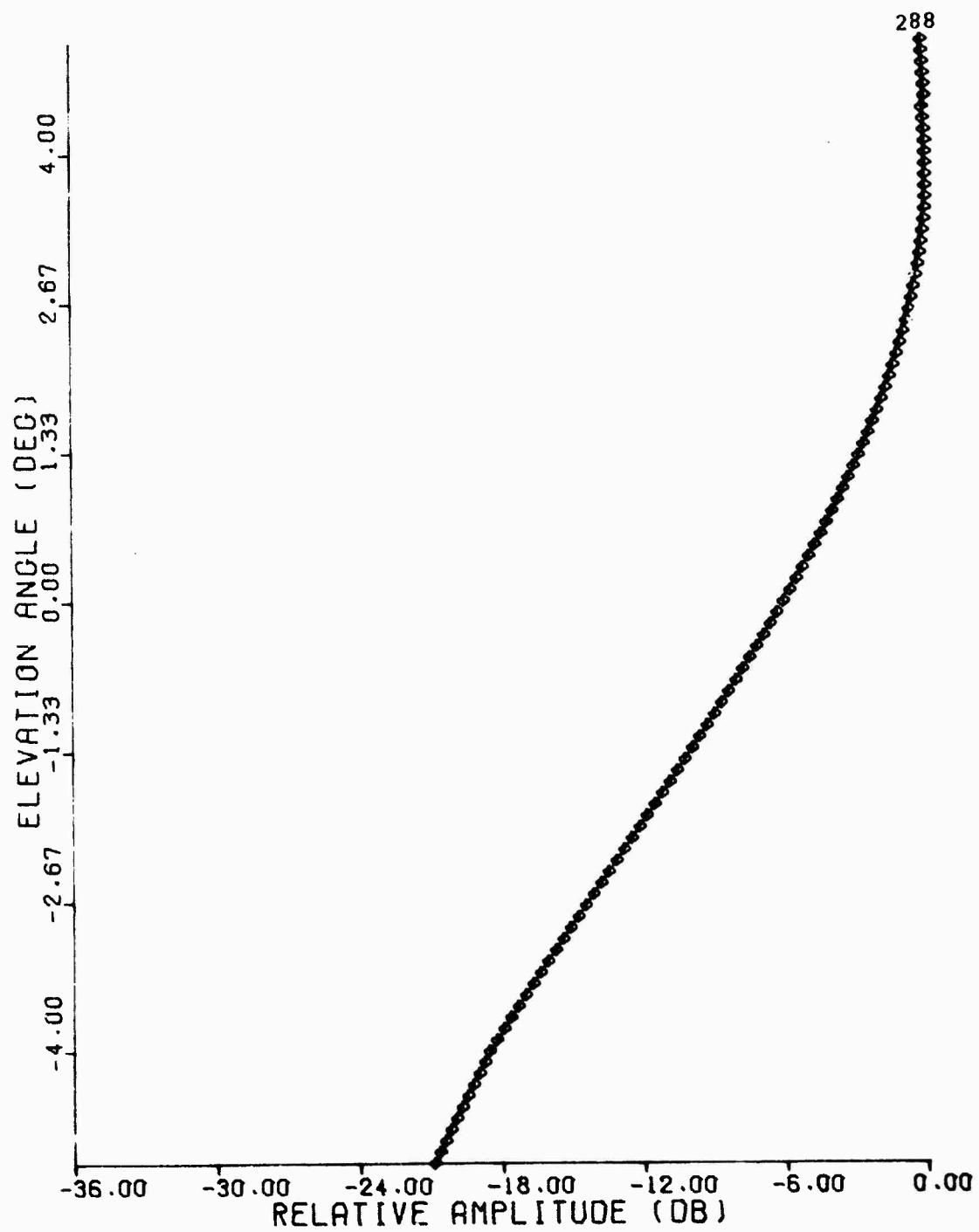
Figure C.52 Least-Squares Fit, 1030 MHz Elevation Pattern
