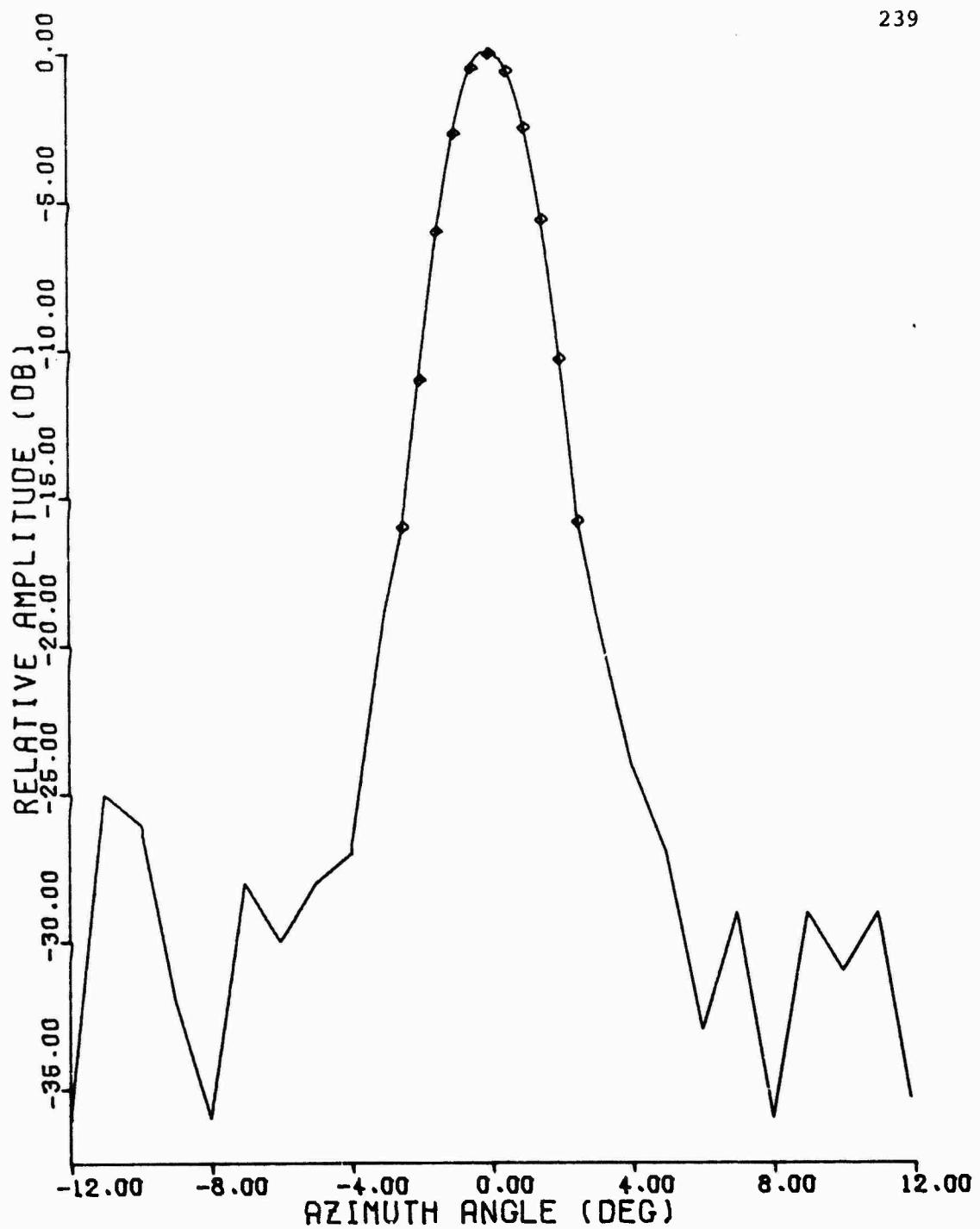
Figure C.4 1090 MHz Azimuth Pattern, FA-8043 Antenna,
